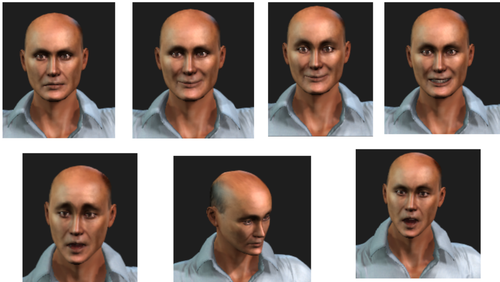
Figure 3.3: Examples of facial expressions and movements (smile, blinking, raising eyebrows, rotating head) that could be animated with the 3D head to spoof the liveness detectors.
