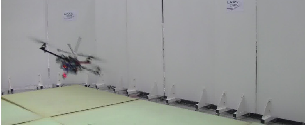
Figure 8.9 – showing the platform flying in a lemniscate manoeuvre at a max velocity of 2.8 \text{ [m.s}^{-1}\text{]} .
