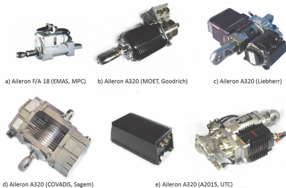
Figure 1.5: Some examples of primary flight control EMAs [8].
