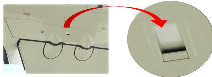
Figure 2.14: Underwing scoops for actuator cooling (EHA of the Airbus A350 aileron) [8].
