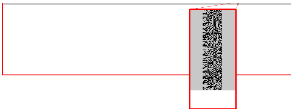
Figure 5.3 – Bitmap obtained from a readback operation after a run of a CNN Int 16 version. Each pixel represents a bit; each bit that was identified with an error appears in black. The red lines are used to limit the region. The grey zone represents the memory usage. Zoom-in is added to increase the visibility of the block event.
