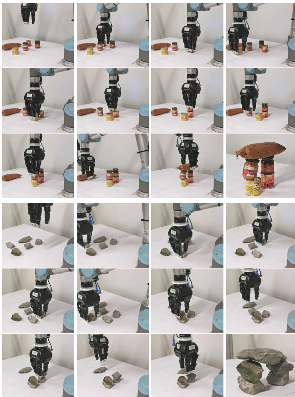
Figure 4.11 – Construction of arches from new primitives that have not been observed during training. Despite the fact that our visual policy has been trained only with block-shaped primitives and only in simulation, it is able to generalize to new diverse primitives in a real robot setup.
