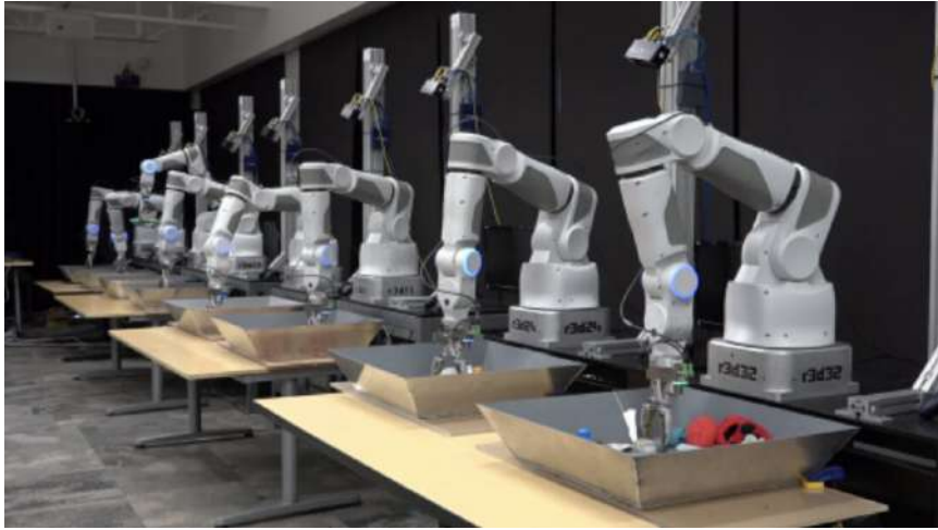
Figure 1.2 – Collecting large-scale datasets for robotics may require thousands of hours of interaction and can be very expensive in practice [Levine et al., 2016].
