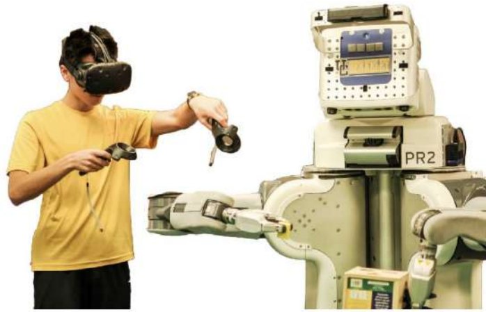
Figure 1.4 – A human teleoperator is using virtual reality to record expert demonstrations for a robot [Zhang et al., 2018].
