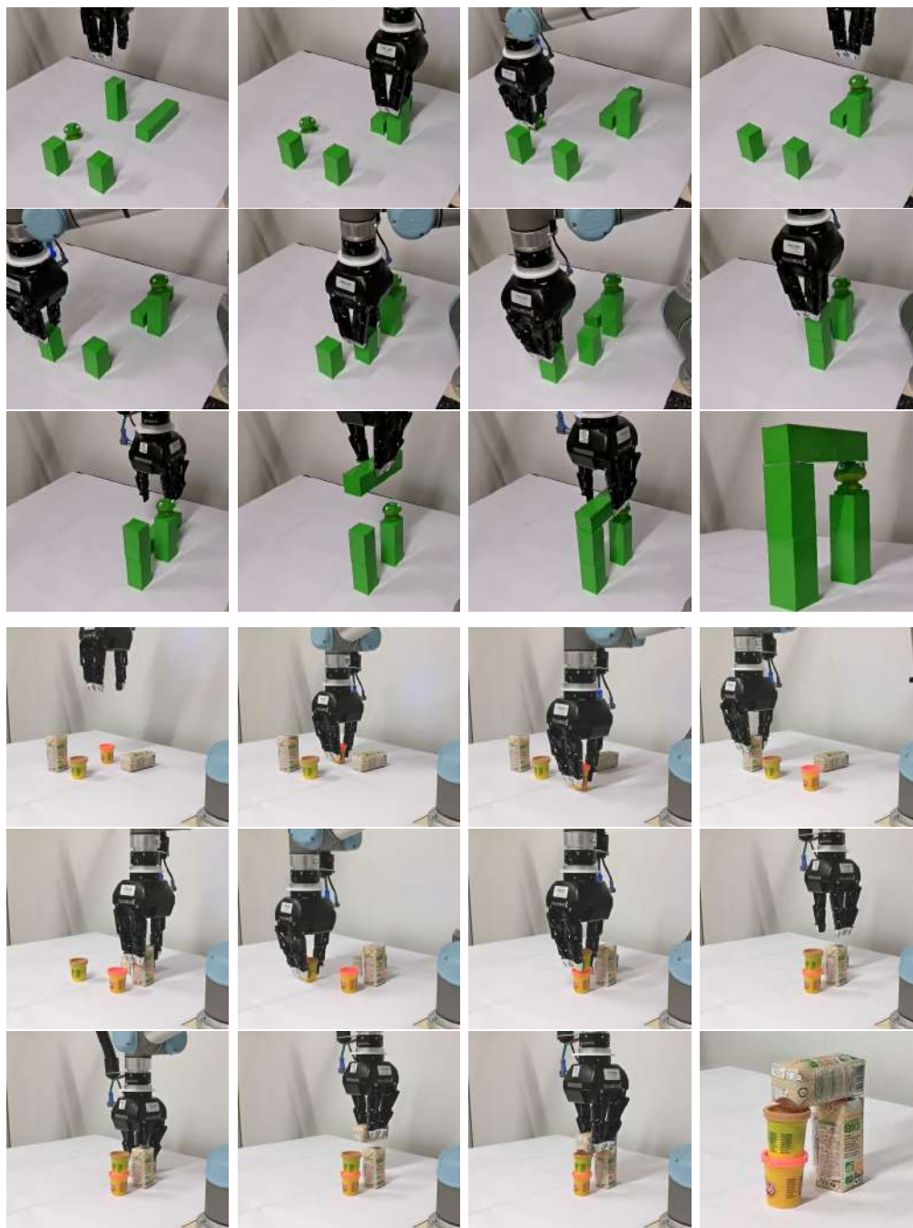
Figure 4.10 – Successful construction of an arch of 5 units from blocks with a real robot (top). Construction of arches from new primitives that have not been observed during training (bottom).
