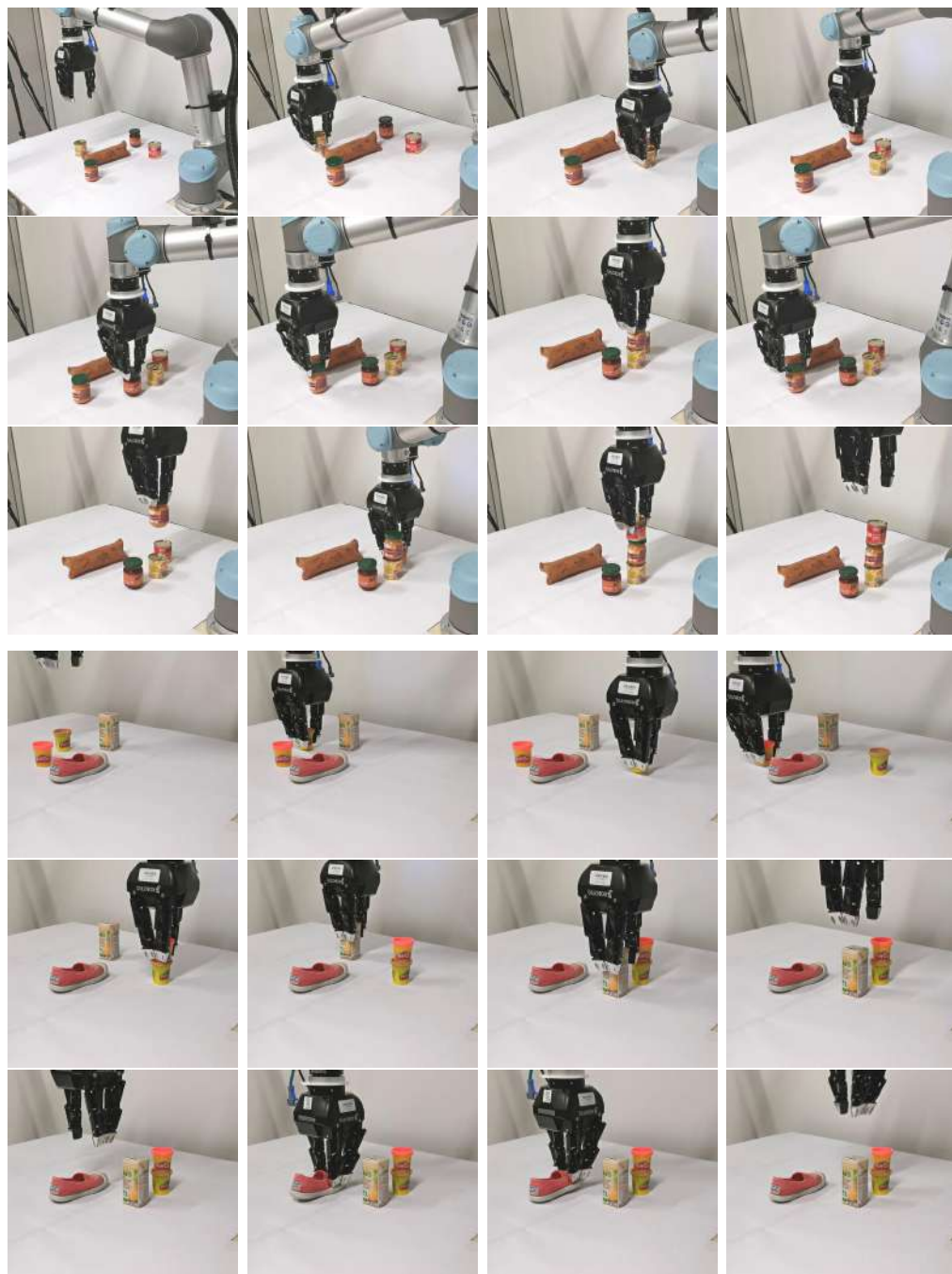
Figure 4.12 – Failure cases for arch construction with a real robot. The failures originate from wrong choice of the target location (top example) and a failure to grasp a soft object (bottom example).
