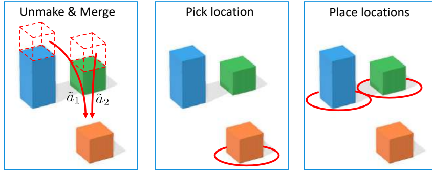
Figure 4.4 – The proposed unmake procedure disassembles objects in multiple ways (left) and generates set of pick & place actions available from each state (right). For visual policies, we use the heatmap representation to predict all the actions simultaneously.
