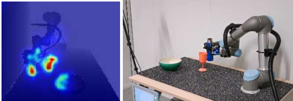
Figure 3.13 – Left: Feature map activations of the RLBC UR5-Breakfast policy are overlaid on the input depth images. Right: corresponding frames taken from a different viewpoint.
