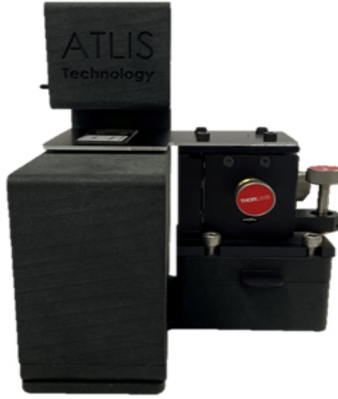
Figure 4.19: ATLIS Modulo microscope for cell analysis
