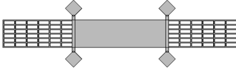
Figure 6.1.1: Scheme of H-square resonator with perpendicular arms anchor position moved to the center part.
