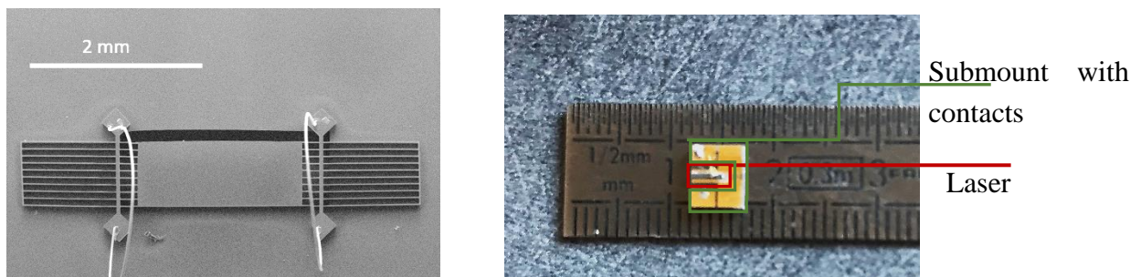
Figure 6.3.1: SEM picture of H-resonator (left panel) and picture of QCL laser with its submount on the millimetric scale (right panel)
