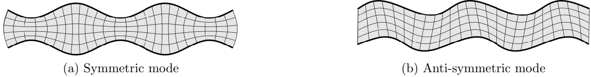
Figure 4.7: Vibrating modes of an infinitely extent elastic layer. While the symmetric mode corresponds to the thickness stretch motion of the layer where the particle velocity varies through the thickness, the anti-symmetric motion corresponds to the bending and shear motions of the layer where the particle velocity is constant through the thickness.
