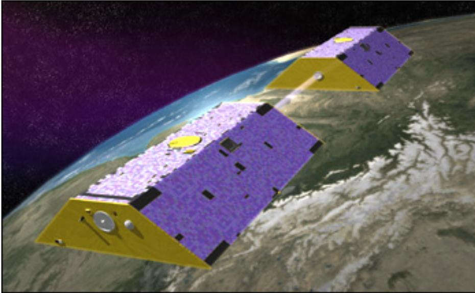
Figure 2.1: The GRACE mission satellites as they orbit Earth. The drawing is not to scale; the trailing spacecraft would actually be about 220 kilometers behind the lead spacecraft [Earth Observatory NASA].
