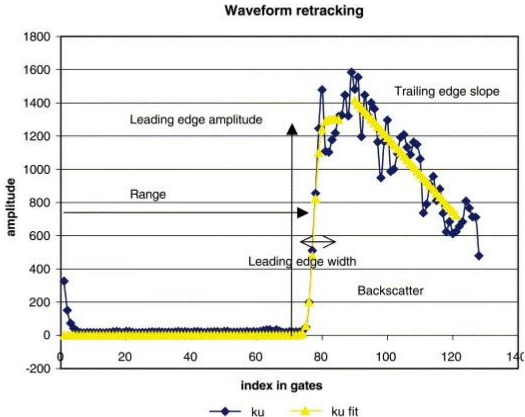
Figure 2.11: The altimetric waveform is represented in blue alongside the retracking fitting function (in yellow). The variables extracted from the altimetric waveform like range, leading edge width and amplitude, and trailing edge slope are shown. Adapted from Legresy et al. [2005].
