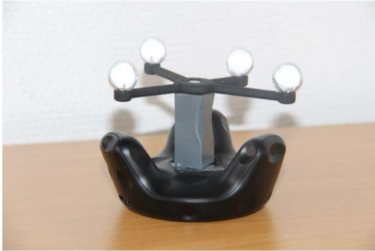
Fig. 1. Vive Tracker with a reflective marker constellation.
