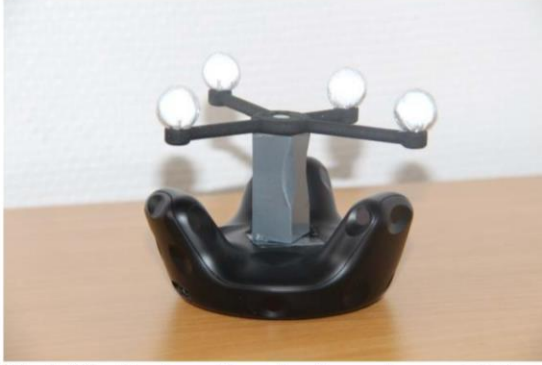
Fig. 1. Vive Tracker with a reflective marker constellation.
