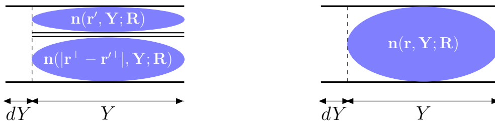
Figure 1.10: Illustration of two terms in Eq. (1.90). The first one is due to the real emission, while the second one represents the virtual correction.
