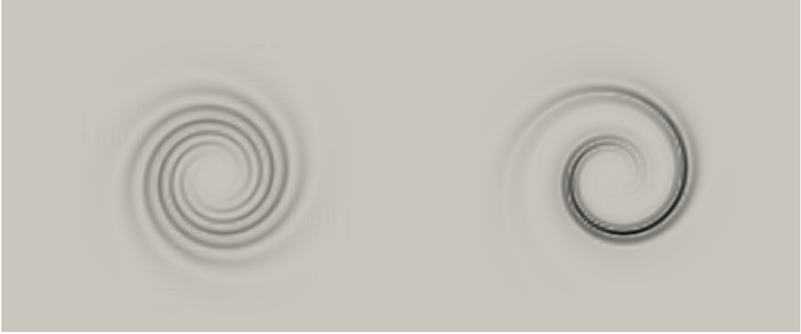
Figure 4.8: Spiral (left) vs. Whip (right) : Contours of vorticity magnitude. Computed for T = 1 and p = 1.6 . On the left, the optimal perturbation remains m = 2 , on the right, the optimal perturbation is a sum of various modes.
