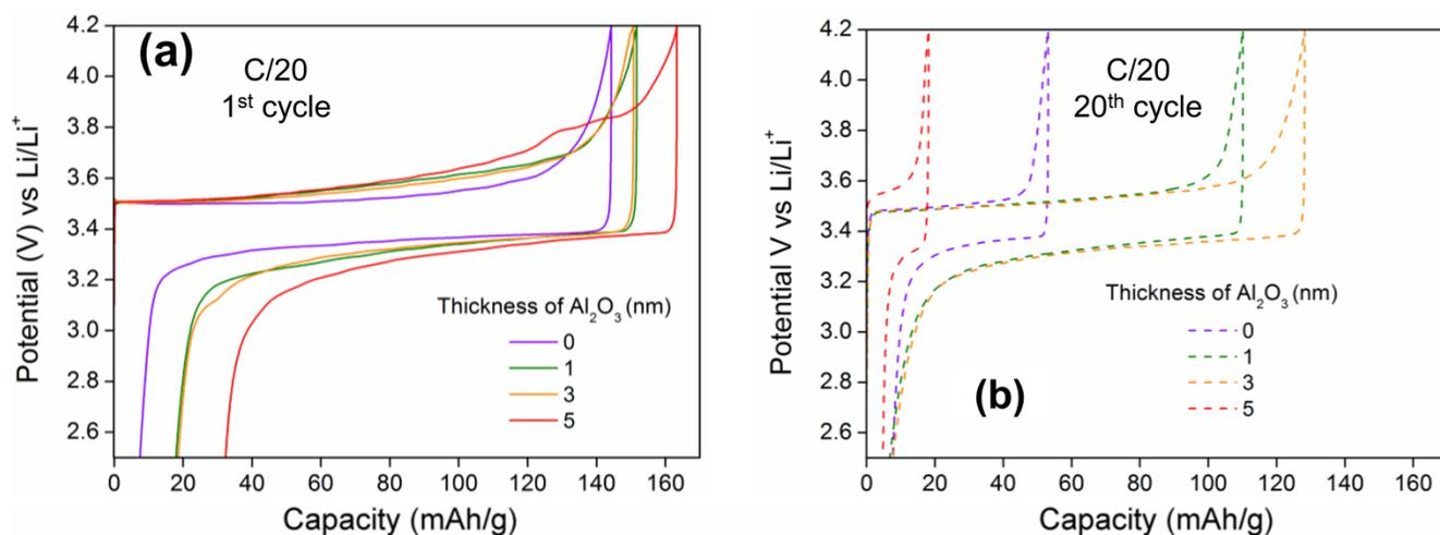
**Figure 4.3** a-b) Charge-discharge curve of 1-mm thick LFP electrodes with and without alumina coated by ALD vs lithium at C/20 rate: 1<sup>st</sup> & 20<sup>th</sup> cycle.
