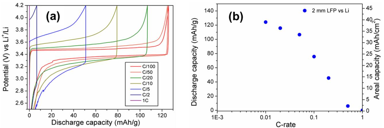
**Figure 3.28** a) Charge-discharge profile for of 2mm thick LFP/Li at different C-rates such as C/100, C/50, C/20, C/10, C/5, C/2, 1C rate. Very low polarization at C/100 rate and increase in polarization as C-rate was increased. b) Ragone plot showing the discharge capacities plotted at different C-rates. A sudden decrease of capacity was seen after C/20 rate due to the mass transport limitations.
