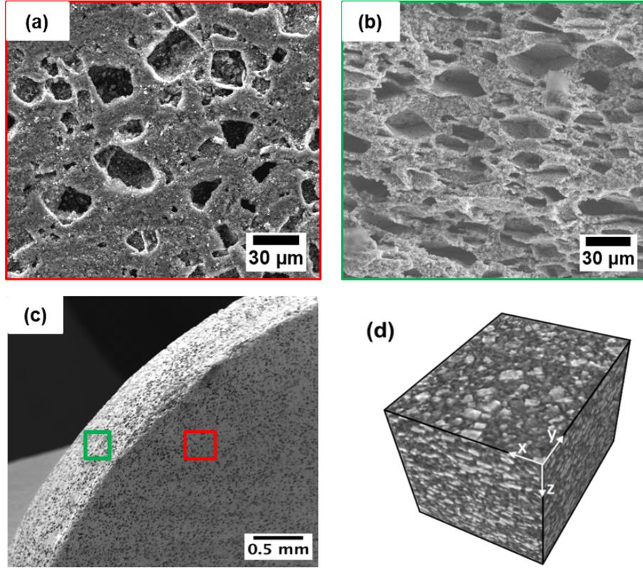
**Figure 2.10** SEM images of 1-mm thick LFP-C porous electrodes a) Top surface view, b) Cross section of the fractured surface of LFP electrode showing the uniformly arranged pores perpendicular to the z direction, c) Low magnification SEM image showing the uniformity of pores in the edge of pellet, d) Stacked SEM images in 3D view showing orthogonal directions.
