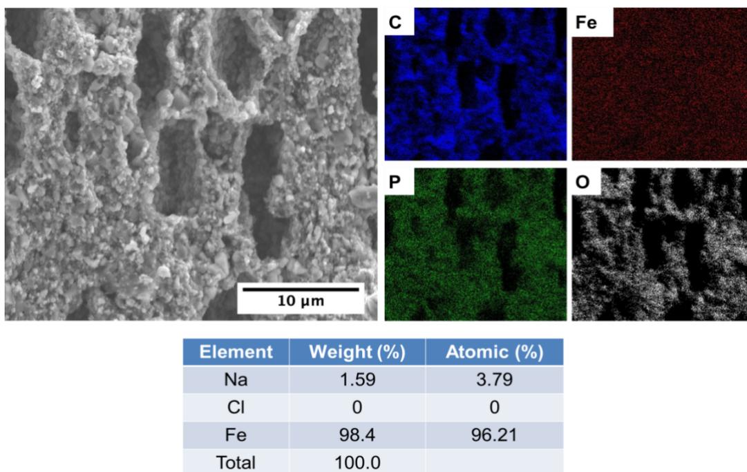
**Figure 2.12** EDX mapping analysis of LFP-C electrode showing the atoms are present uniformly over the surface of the particles with spectrum showing Fe, P and O atoms in LFP with no chlorine atoms after NaCl dissolution present in LFP electrode.
