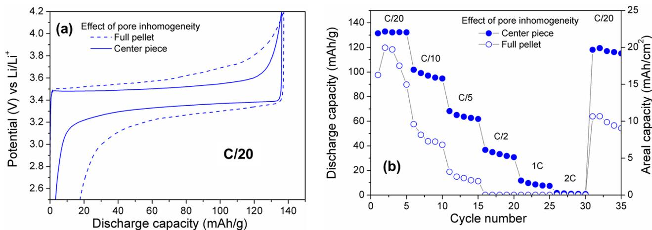
**Figure 2.17** Effect of pore inhomogeneity observed in the LFP-C electrode: (a) Charge-Discharge curve of 2<sup>nd</sup> cycle of full LFP-C pellet and broken piece of LFP-C pellet showing big difference in polarization, (b) Comparison of rate capability curve of LFP-C electrodes with full pellet and a broken piece taken from the center.
