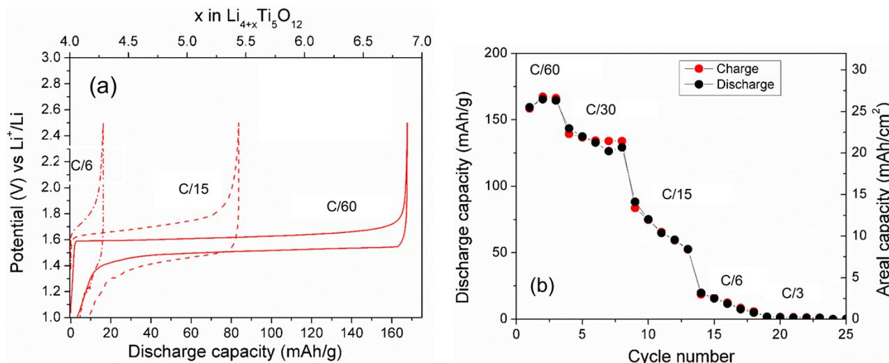
**Figure 2.22** (a) Charge-Discharge profile of 1-mm thick LTO/Li at C/60, C/15 and C/6 rates, (b) Rate capability of LTO vs Li showing the decrease in specific capacity due to mass transport limitations in the liquid phase.
