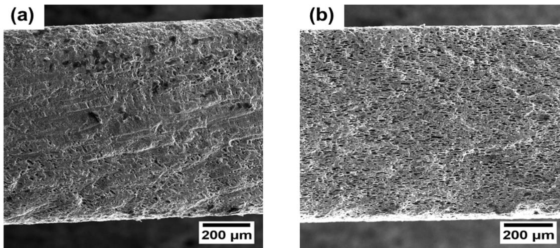
**Figure 2.16** Comparison of SEM images of cross section in the full pellet and fractured surface in the middle of the 1-mm thick binder free LFP electrodes. Pore non-uniformities are present in the edges of the full pellet than the middle of the pellet.
