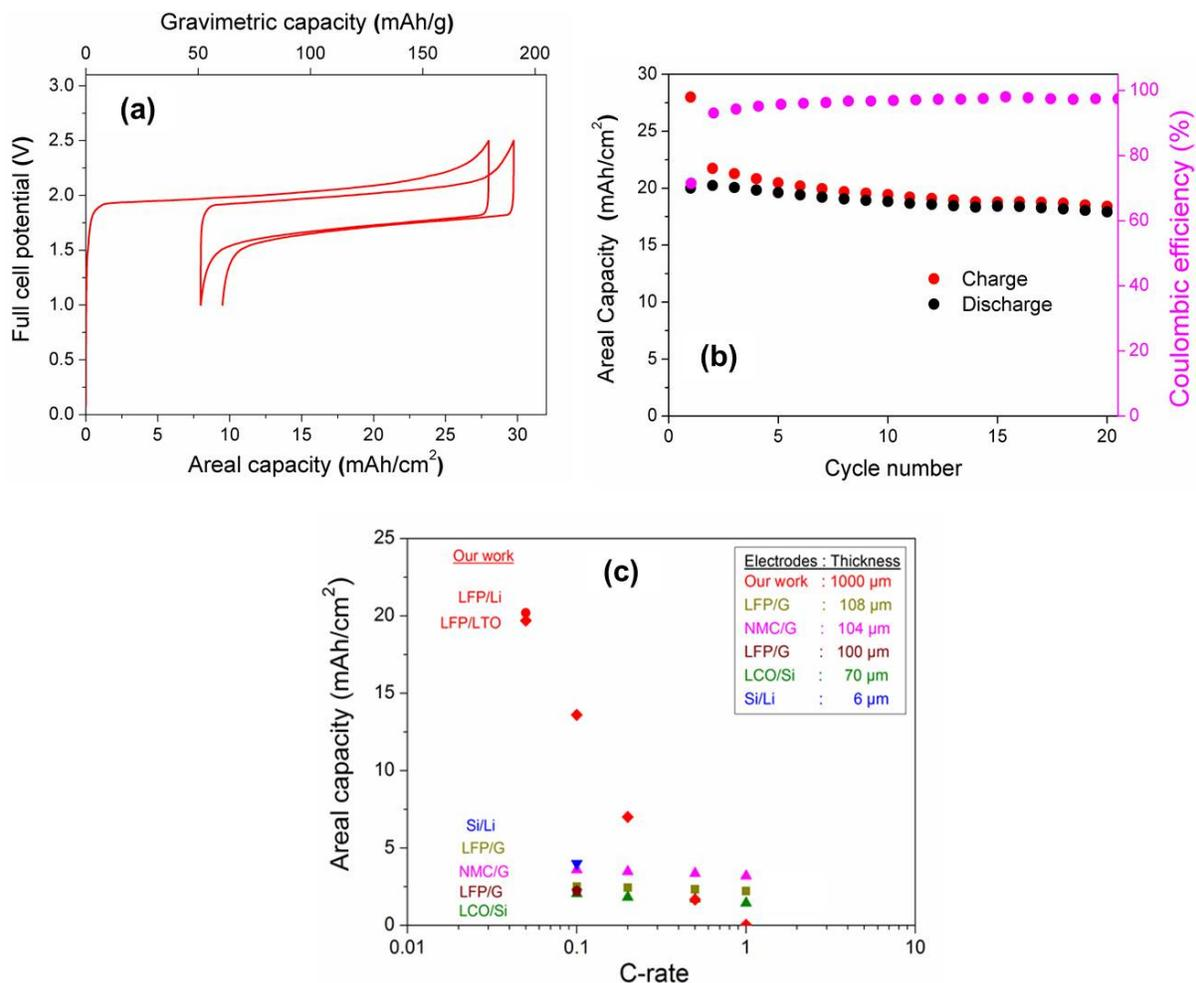
**Figure 2.23** (a) Charge-Discharge profile of 1mm thick LFP/LTO full cell at C/20 rate, (b) Capacity retention curve of the LFP/LTO at C/20 rate. LP30 was used as an electrolyte for the electrochemical cycling. (c) Ragone plot of LFP/Li and LFP/LTO battery systems compared with conventional battery systems.
