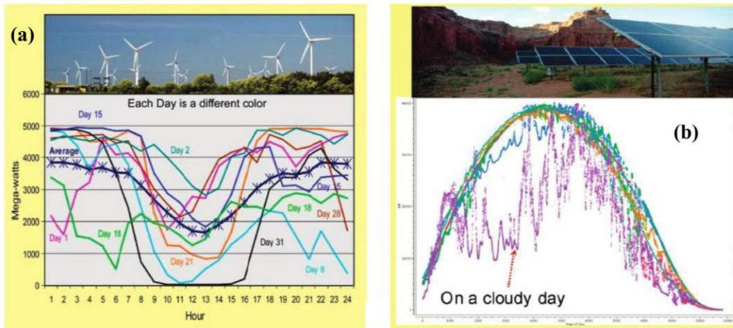
**Figure 1.3** (a) Amount of electricity generated by a) Wind and b) solar power sources. Drastic fluctuations in the supply of energy are observed in both wind and solar power making it less efficient for electrical energy generation facilities.
