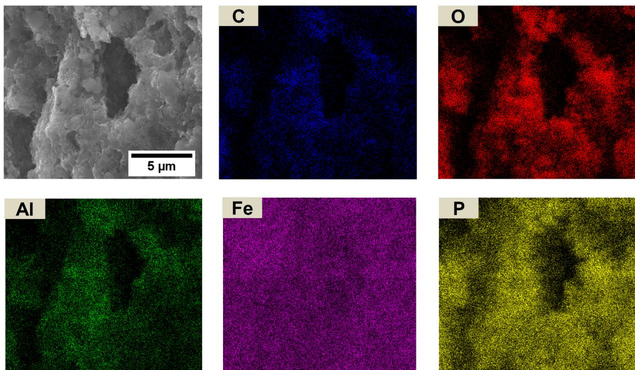
**Figure 4.2** EDX mapping of LFP electrode coated with 3nm thick  $Al_2O_3$  using ALD technique. Cross section of LFP electrode is shown in top left. The presence of Aluminium atoms confirm the alumina layer coating done on the surface of the LFP particles.
