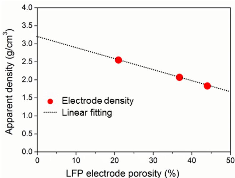
**Figure 3.21** Apparent density vs electrode porosity showing the linear increase of density when porosity is decreased and the intercept of the line corresponds to the 1-mm thick LFP electrode (99% compacity).
