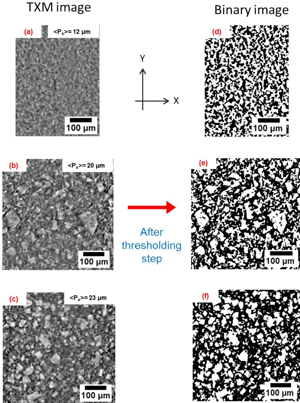
**Figure 3.4.** a-c) 2D-TXM images of 12  $\mu\text{m}$ , 20  $\mu\text{m}$  and 23  $\mu\text{m}$  average pore sized LFP electrode, d-f) corresponding thresholded image of the electrodes showing pores in white and solid as black.
