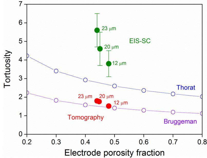
**Figure 3.16** Tortuosity compared between the EIS and micro tomography methods for the three different pore sized LFP electrodes (12,20 and 23 $\mu\text{m}$ ). Average pore size values are written for comparison.
