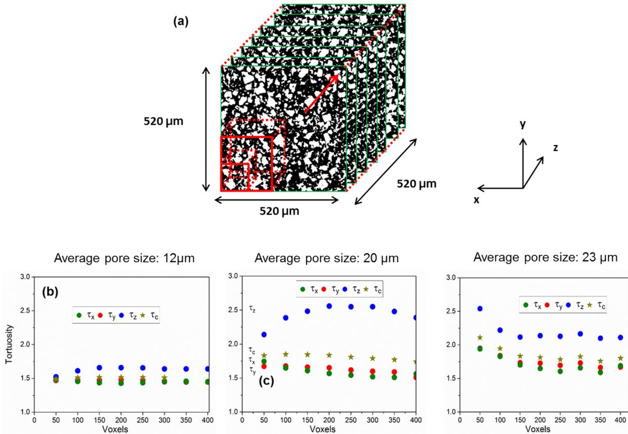
**Figure 3.10** Scale effect of the three 1-mm thick LFP electrode showing the tortuosity values determined from each sub section. Tortuosity stabilization was obtained after 150 voxels for 23  $\mu\text{m}$  pore sized LFP electrode in 3.8d.
