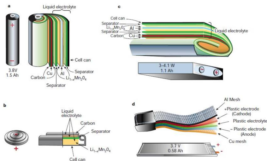
**Figure 1.11** Various Li-ion battery configurations available in the market. a) Cylindrical b) coin c) prismatic and d) thin and flat. About 50% in battery mass and more than  $2/3^{\text{rd}}$  of battery volume is occupied by inactive materials irrespective of different configurations. Reprinted from [62].
