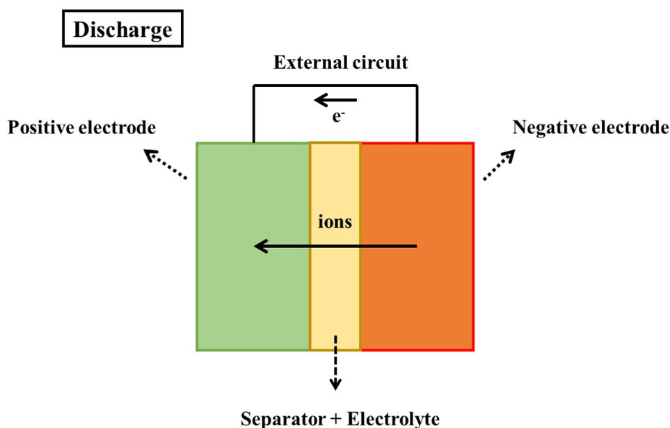
**Figure 1.4** Schematic of a generic electrochemical cell. Electron exchange is occurring at a given potential in each electrode, normally paired with an ion exchange through the electrolyte filled separator.
