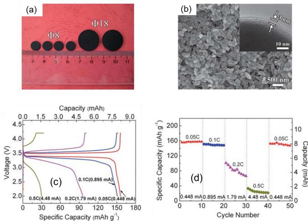
**Figure 1.19:** Fabrication of thick carbon coated LFP electrode using conventional sintering [109]. a) Digital photograph of different sizes of sintered electrode prepared at 700 °C for 7 hours b) Carbon coated LFP electrode with 90 nm-3  $\mu\text{m}$  pore size equivalent to the size of citric acid as porogen. c) Charge-discharge curve at different C-rates. d) Poor performance at 0.2 C and 0.5 C rates are co-related to the smaller pore size due to poor Li diffusion.
