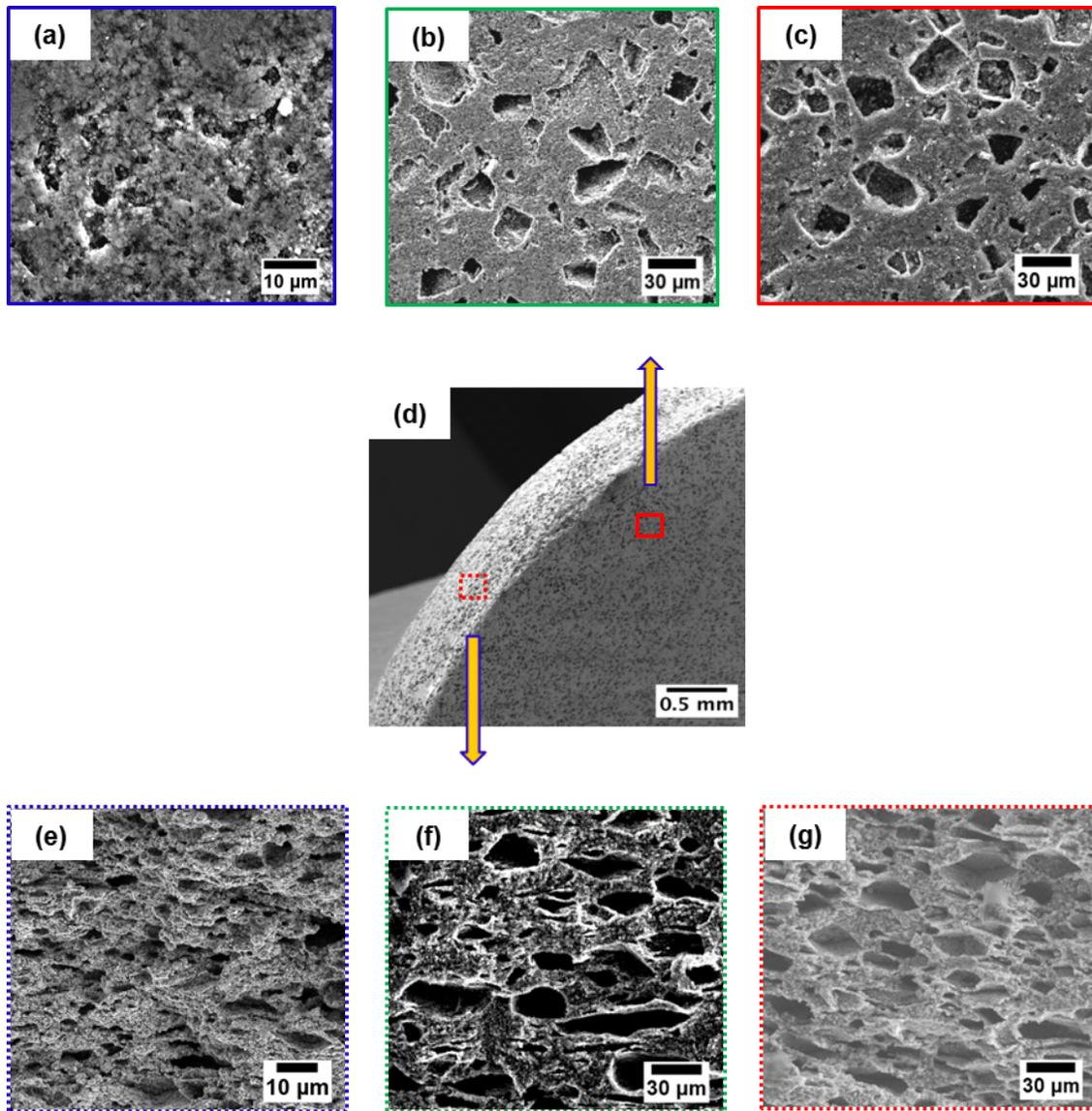
**Figure 3.3** SEM images of porous LFP electrodes containing the pores created by the NaCl dissolution. (a, b, c) top surface view of the electrodes showing the cubic shape of the crystals with corresponding sizes of the crystals used, (e,f,g) Cross section of thick LFP electrodes showing the pore shape aligned perpendicular to the z-direction due to the uniaxial pressing of SPS operation.
