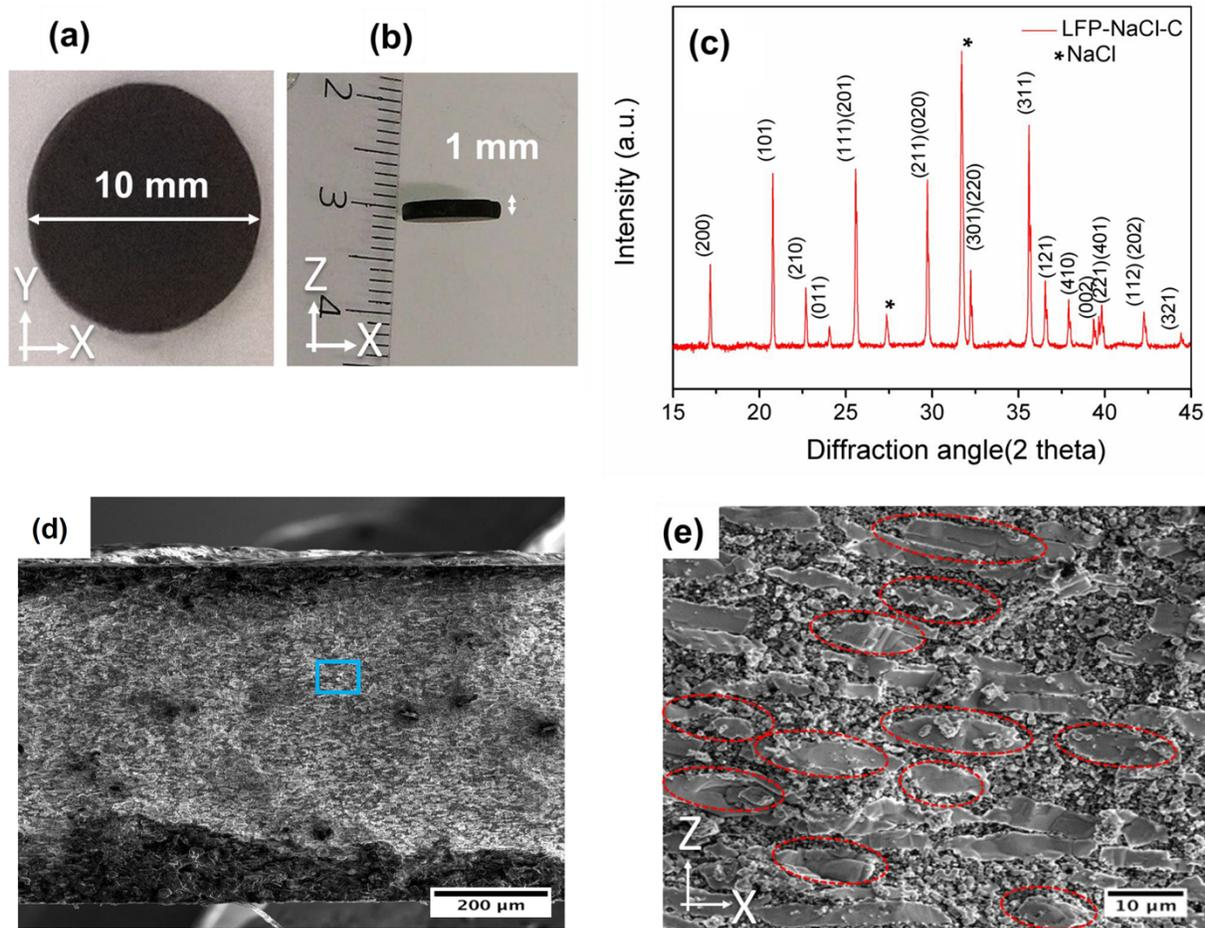
**Figure 2.9 a-b)** Digital photo of the LFP-C pellet obtained after SPS treatment, c) XRD pattern of sintered LFP-NaCl-C pellet, d,e) SEM image of cross section of LFP-NaCl-C pellet showing the embedded NaCl particles along with LFP and Carbon.
