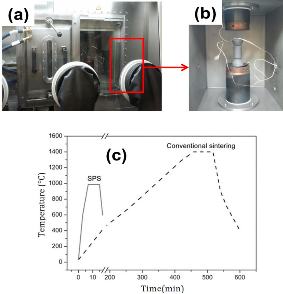
**Figure 2.2** Advantages of SPS technique: a) Digital photograph of SPS technique attached to the glove box installed in LRCS, Amiens, b) Graphite die packed with electrode powder placed in the SPS chamber, c) Comparison of SPS and conventional sintering parameters.
