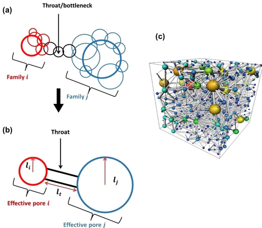
**Figure 3.6.** a) Two pore families connected by the pore throat b) Effective pores and throat obtained after assigning effective pore radii and throat lengths. c) Schematic showing the spheres and cylinders forming the interconnected pore network [26].
