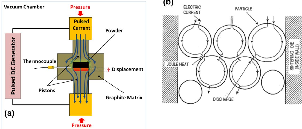
**Figure 2.1** a) Schematic of SPS process showing application of temperature and pressure simultaneously to the graphite die holding the powder in order to prepare thick pellet [7], b) Pathway of direct current passing to the powders forming sinter necks with strong grain-grain bonding and well-connected atomic interfaces [3].
