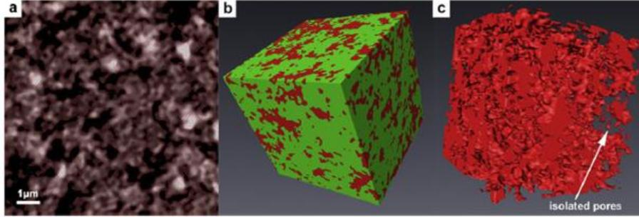
**Figure 1.14** X-ray computed tomography (XCT) 3D image reconstruction of cropped cube of LFP/C electrode ( $15 \mu\text{m} \times 15 \mu\text{m} \times 15 \mu\text{m}$ ) after the segmentation (a) in a single slice, (b) LFP/C cube (green-LFP/C and red-pores) with 28.68% porosity and (c) Interconnected pore network with few closed pores are observed. Image reconstruction was done by Avizo and ImageJ software [82].
