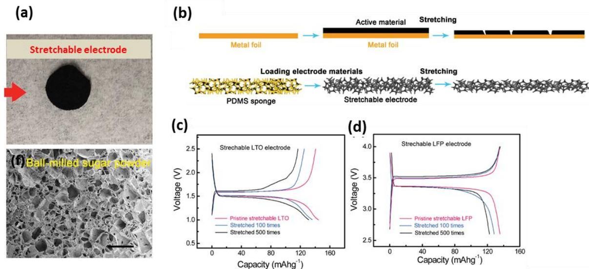
**Figure 1.25** 3D porous sponge inspired LFP and LTO electrodes by sugar templating. a) Stretchable LFP/LTO electrode and corresponding SEM images of the porous LFP or LTO electrode with pore size equivalent to the initial sugar particles size. Scale bar: 500  $\mu\text{m}$ . b) Schematic of conventional and stretching electrode fabrication method. c) and d) Charge-discharge profiles showing enhanced performance of stretchable electrodes vs lithium. Reprinted from [183].
