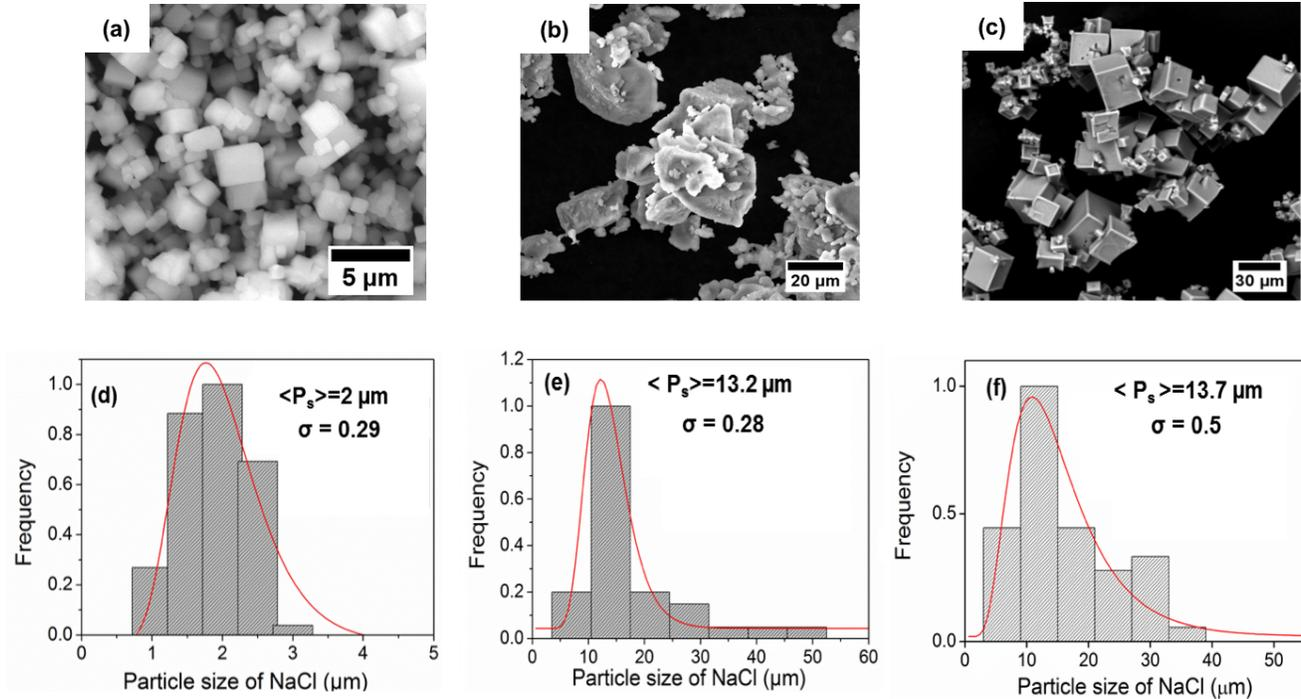
**Figure 3.2** (a-c) SEM images of NaCl particles prepared by three methods. (d-f) Corresponding particle size distribution obtained for the three NaCl crystals using FIJI software and fitted with log-normal distribution.
