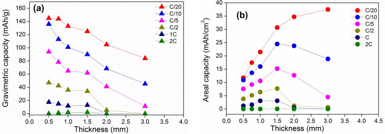
**Figure 3.26** Comparison of a) gravimetric capacity and b) areal capacity as function of electrode thickness at different C-rates. Increase in areal capacity was observed due to high active material loading and corresponding decrease of gravimetric capacity is seen due to the mass transport limitations.
