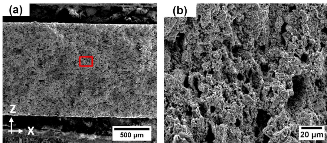
**Figure 4.6** Cross section SEM images of NVPF electrodes showing 1-mm thickness and closer magnification shows the pore size of 10-20  $\mu\text{m}$  corresponds to the particle size of the NaCl crystal.
