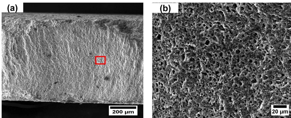
**Figure 4.1** (a) Cross sectional SEM image of the alumina coated 1-mm thick LFP electrode by ALD technique showing the 1-mm electrode thickness (b) higher magnification shows the uniform arrangement of pores present in the LFP electrode.
