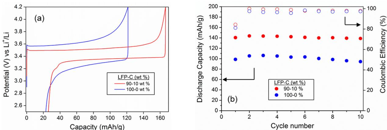
**Figure 2.15** Comparison of electrochemical performance of LFP-C pellet having two different compositions of 90-10 and 100-0 wt.% (a) Charge-discharge profile at C/20 rate and (b) capacity retention curve at C/20 rate of 1-mm thick LFP electrodes with and without extra carbon added.
