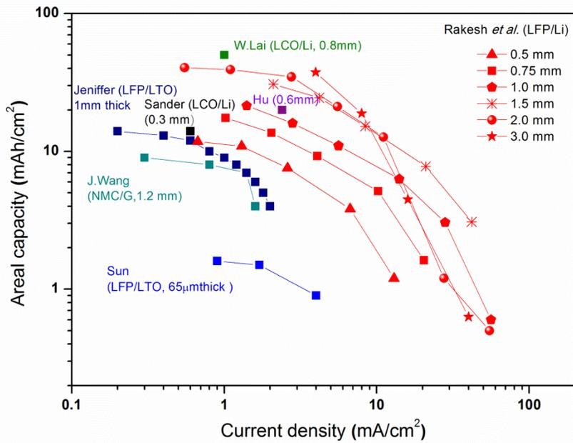
**Figure 3.29** Ragone plot comparing areal capacity versus current density of the thick electrodes prepared with SPS/templating and reported literature values. [Note: Thickness and battery systems are given in brackets] [45]–[50].
