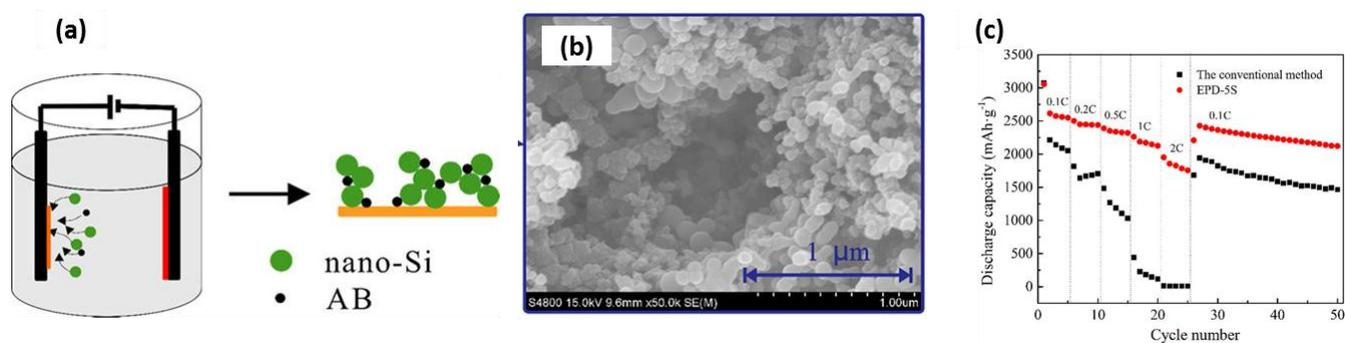
**Figure 1.13** Electrodeposition of nano silicon and its electrochemical performance. a) Application of short current pulse accelerates the uniform coating of nano silicon present in the electrochemical bath. b) SEM image clearly shows the nano size of silicon coated with acetylene black. c) Superior performance of ED silica is observed from the rate capability tests compared to the conventional method. Reprinted from [80].
