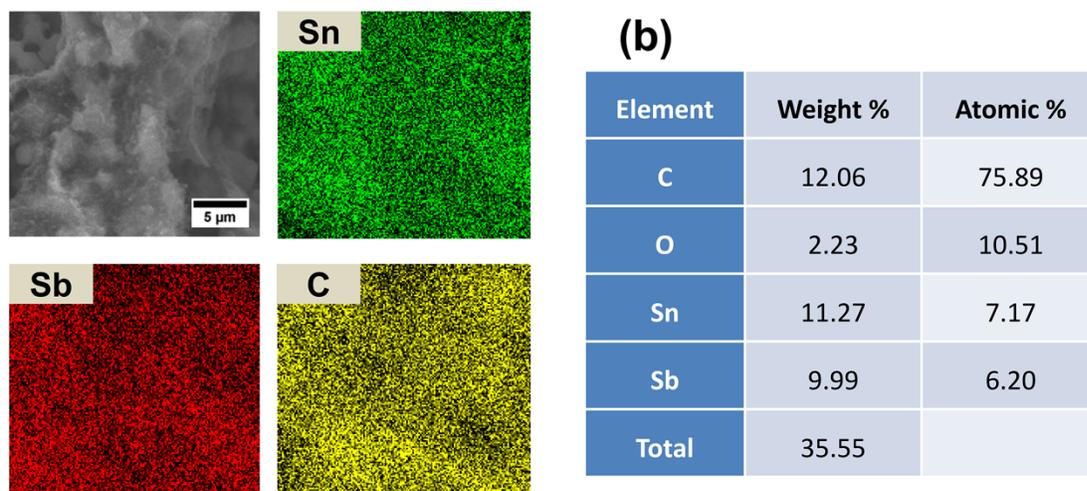
**Figure 4.13** a) EDX mapping of 1-mm thick SnSb electrode fabricated using SPS and templating strategy showing the tin and antimony are homogeneously distributed in the Sn-Sb surface, b) Quantification of individual components present in the SnSb alloy electrode.
