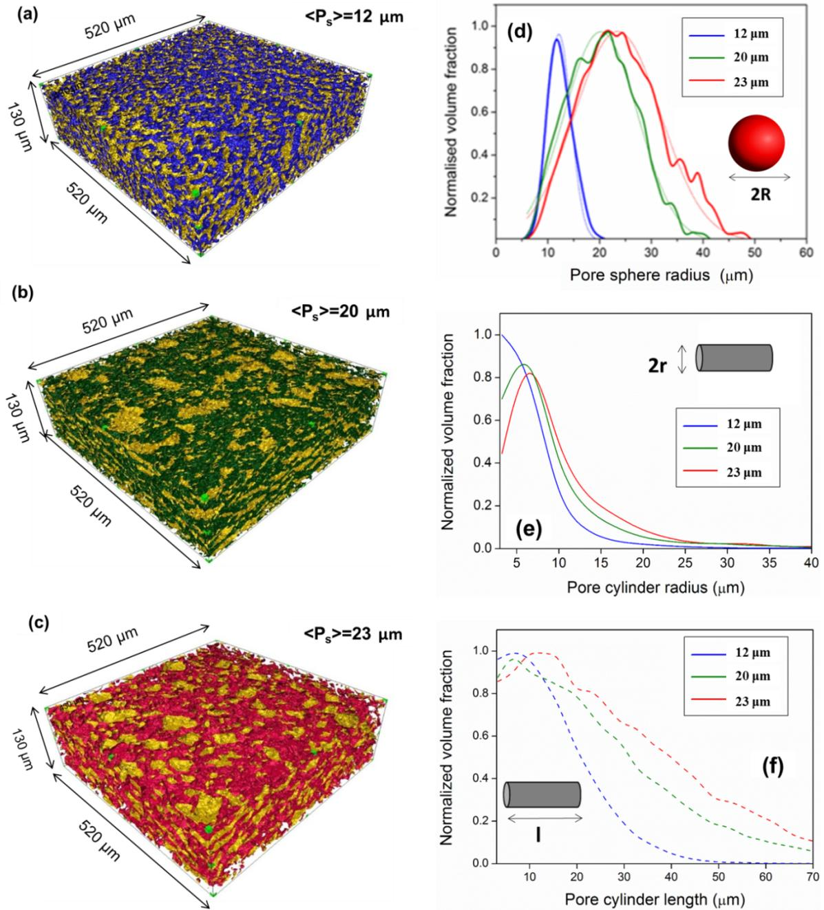
**Figure 3.7** 3D reconstructed images of three 1-mm thick LFP electrodes using AMIRA software. d-e) The individual pore size distribution obtained by fitting as spheres and cylinders using Blunt algorithm.
