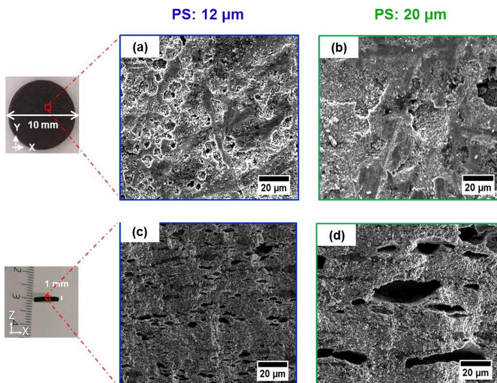
**Figure 3.18** SEM images of 1-mm thick LFP electrodes prepared with 21% porosity: a, b) Top surface view showing the pore shape and size corresponding to the initial crystal size of 12 and 20  $\mu\text{m}$  ; c, d) Cross sectional images of the porous electrodes showing the distribution of cylindrical pores.
