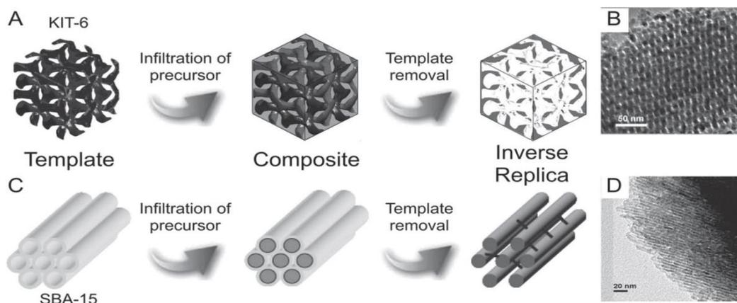
**Figure 1.22** Schematic of templating methods to create porous electrodes[168]. KIT-6 and SBA-15 are the silica material used as hard templates creating micro/meso pores in the electrode material obtained by chemical etching.
