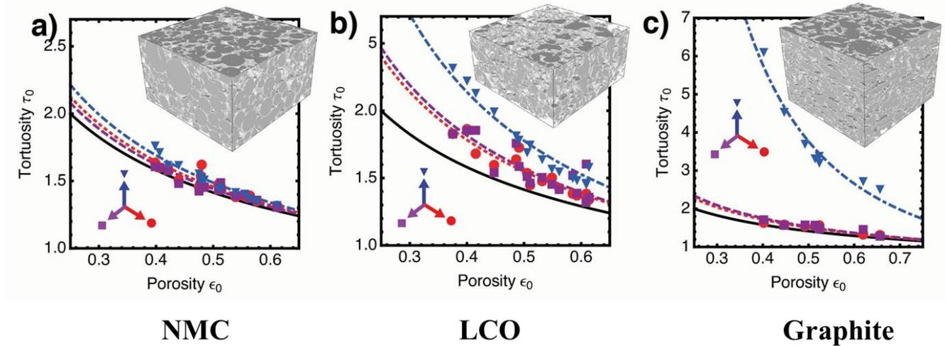
**Figure 1.15** Tortuosity measured for 3 electrodes a) NMC, b) LCO and c) Graphite using numerical differential effective medium (DEM) approximation method. Large degree of anisotropy was observed for graphite compared to other two electrodes that can be explained by high tortuosity values and big deviation from the classical Bruggeman relation.
