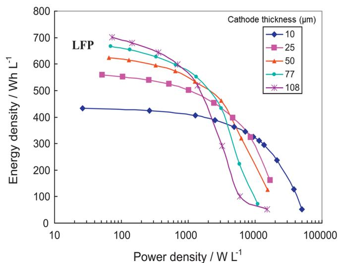
**Figure 1.18** Ragone plot of LFP/G cell with different cathode thicknesses [97]. Linear increase energy density as thickness and decrease in power density which is due to increase in Ohmic drop and diffusion limitations for the thicker electrodes.
