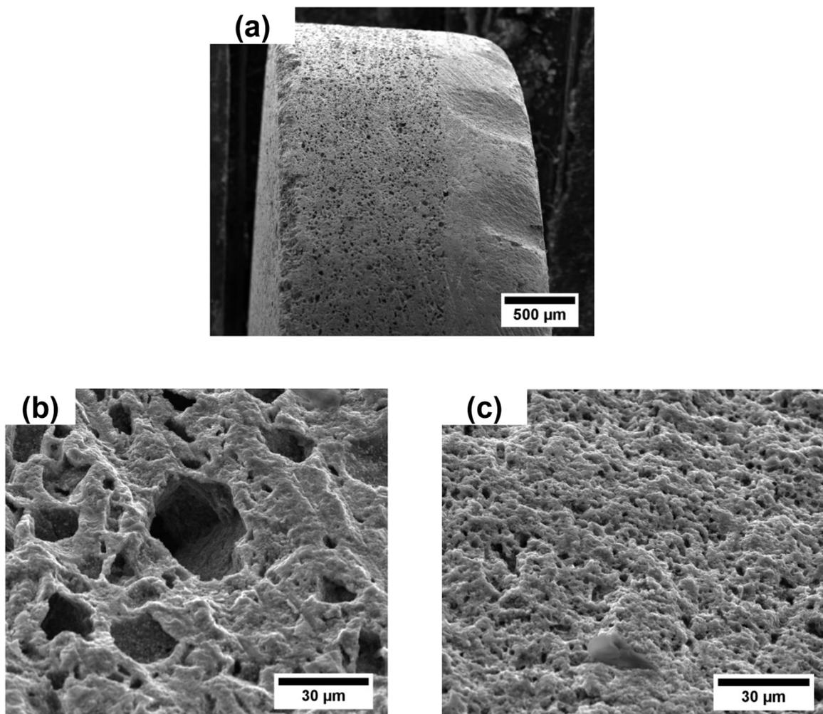
**Figure 4.18** (a) The thick LFP electrode with two layers of different pore sizes obtained by using two different particles sized templates. (b-c) Higher magnification of LFP electrodes in each layer showing the larger and smaller pores.
