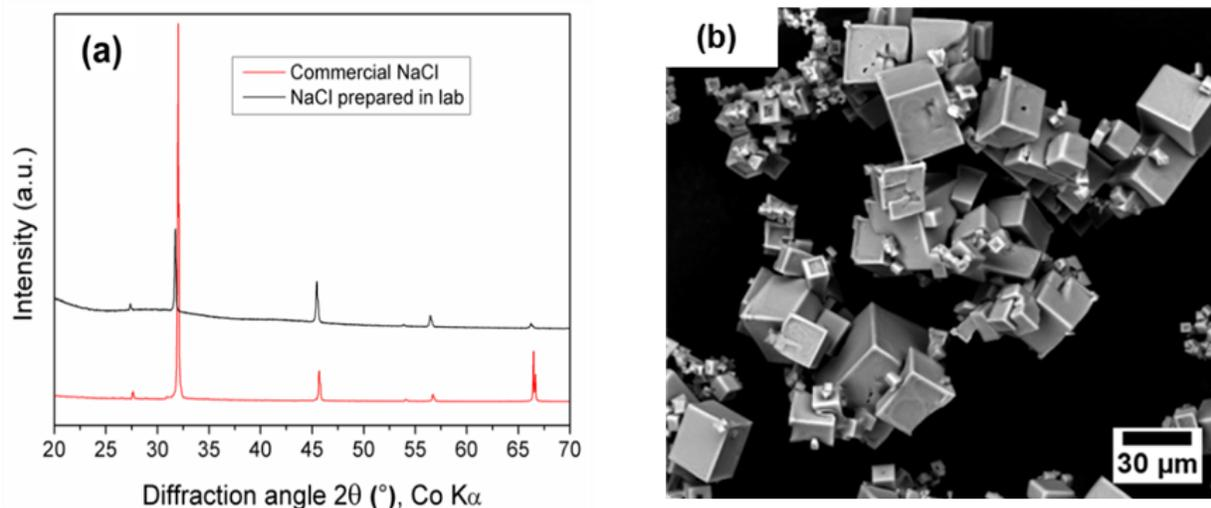
**Figure 2.4** XRD pattern of NaCl template prepared by evaporative crystallization, b) SEM image of cubic shaped salt showing the average particle size is 10  $\mu\text{m}$ .
