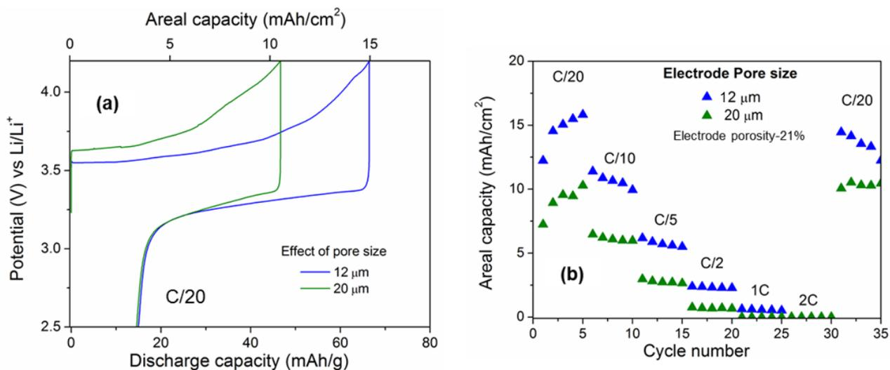
**Figure 3.19** Effect of pore size for 21% porosity electrodes. a) Charge-discharge profile of first cycle at C/20 rate of 1-mm thick LFP-C electrodes showing high polarization. b) Rate capability curve showing significant capacity increase for smaller pore sized electrodes at different C-rates.
