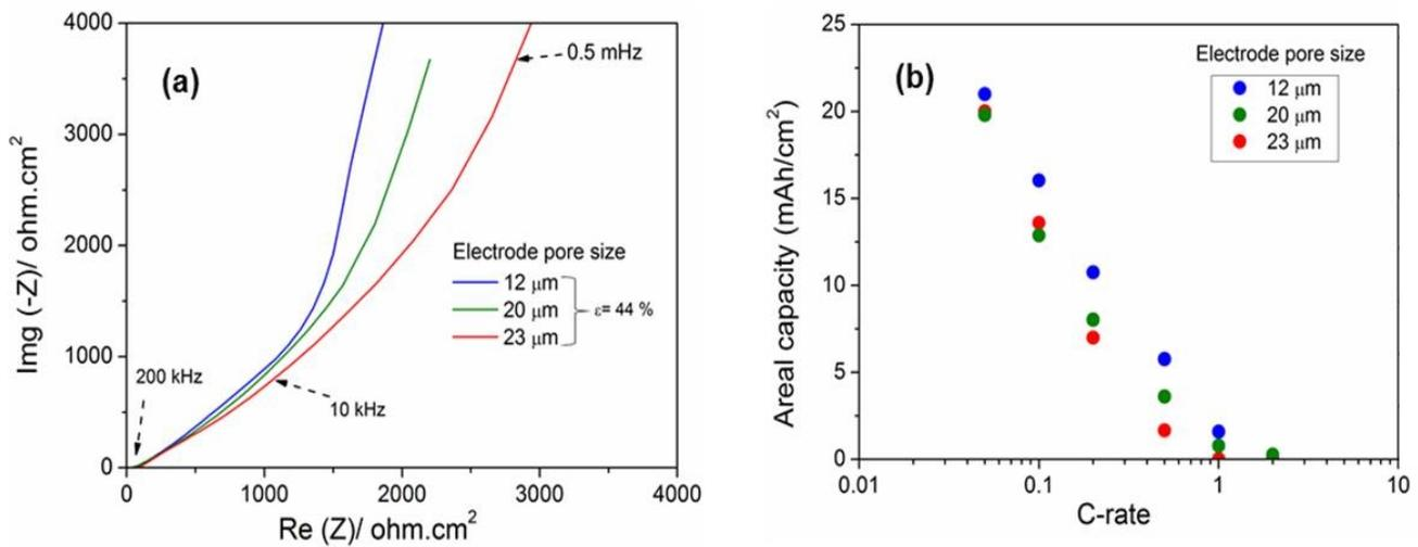
**Figure 3.15** a) Impedance spectrum of LFP-C electrodes obtained from the EIS-symmetric cell experiments. The ionic pore resistances are measured as an effect of pore size by fitting the experimental curve with the transmission line model. b) Rate capability performance in-line with the EIS experiments.
