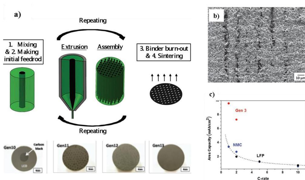
**Figure 1.23** Co-extrusion/sintering of LCO electrodes and its electrochemistry[110]. a) Initial feed rod of carbon/binder mixture surrounded by LCO active material was extruded multiple times to obtain periodic array and then sintered feed rod turns to porous channels. b) SEM images show the macro-pore channels where controlled channel spacings are observed. c) Higher areal capacity at 1C and 2C rate is compared to conventional electrodes.
