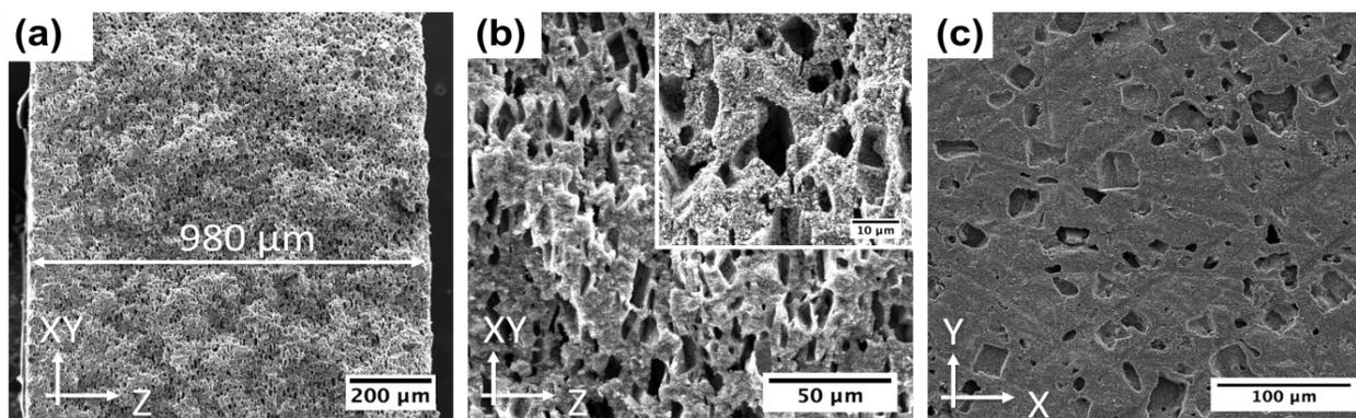
**Figure 2.20** a) SEM images of LTO electrode: (a) Cross section of LTO electrode showing 1-mm thickness, (b) Uniform distribution of pores is seen in cross section and (c) top surface view of LTO electrodes.
