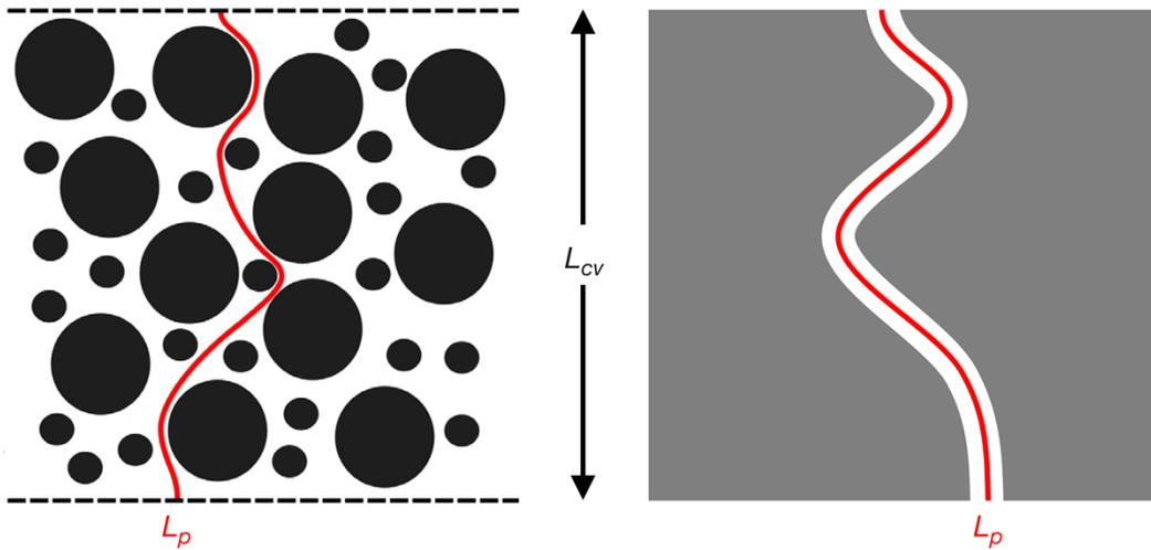
**Figure 3.5** a-b Geometrical tortuosity representation in the composite electrode showing the effective path length  $L_p$  and edge length of the control volume,  $L_{cv}$  ( $\mathcal{T} = L_p / L_{cv}$ ) [21].
