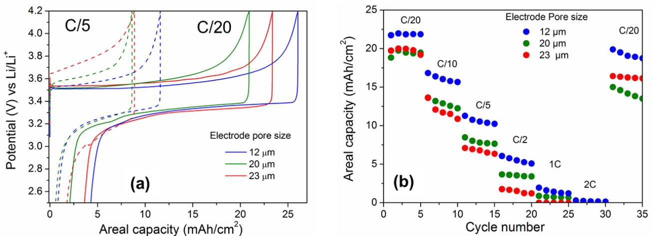
**Figure 3.17** (a) Charge-discharge profile of 1-mm thick LFP-C electrodes against lithium at C/5 rate with three different pore sizes. (b) Rate capability curve showing highest capacity for smallest pore sized LFP electrode.
