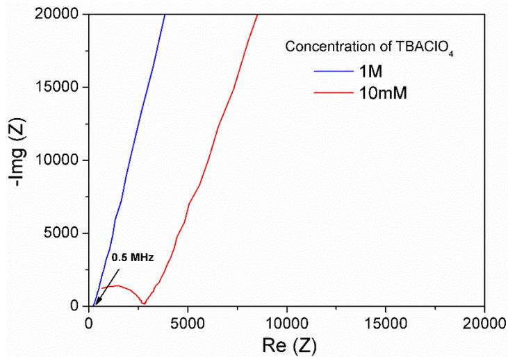
**Figure 3.14** Electrical impedance spectrum obtained from the conductivity measurements using tetra-n-butyl ammonium perchlorate dissolved in EC: DMC solvent mixture. The intercept in the real axis represent the electrolyte resistance thereby electrolyte bulk ionic conductivity can be measured.
