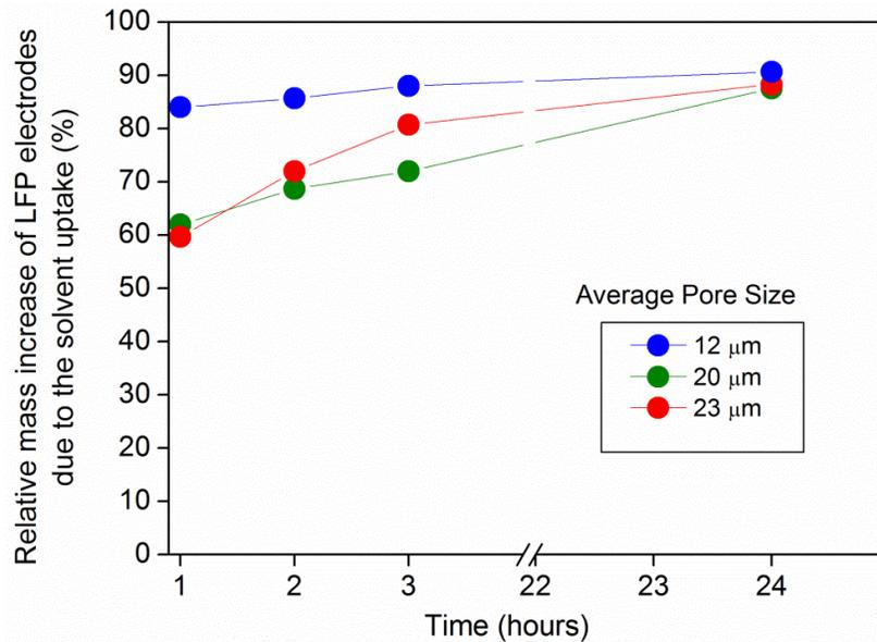
**Figure 3.13** Impregnation test result showing the behavior of rate of filling of solvent as a function of time. The rapid increase in electrode mass was obtained for the 12  $\mu\text{m}$  pore sized electrodes.
