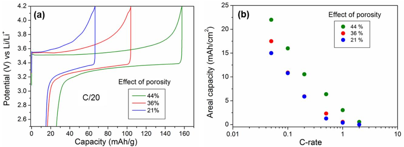
**Figure 3.22** a) Charge-discharge cycling curve of the 1-mm thick LFP electrodes with three different porosities at C/20 rate, b) Ragone plot showing the improved C-rate performance for 44 % porous LFP electrodes.
