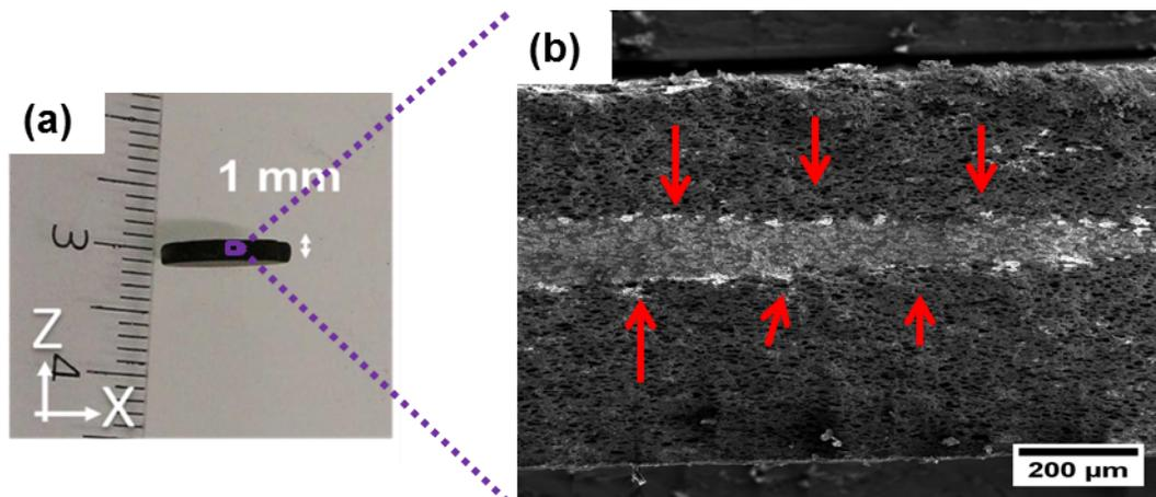
**Figure 2.18** (a) Digital photo showing 1-mm thickness of LFP electrode, (b) SEM image of 1-mm thick LFP pellet after dissolution of salt particles. Incomplete dissolution of salt particles was observed in the middle (white) of the cross section of the full LFP-C pellet. The water penetrates to dissolve salt particles from the either sides of the pellet and shows the salt crystals (in bright) due to incomplete NaCl dissolution.
