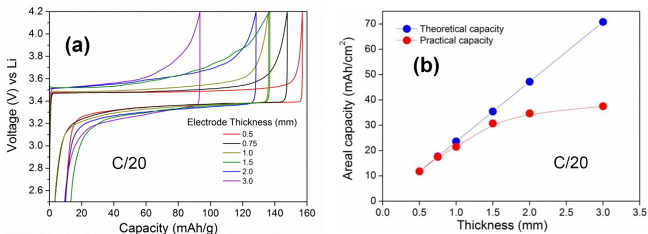
**Figure 3.25** Electrochemical performance as a function of electrode thickness at C/20 rate: a) Charge-Discharge profile of second cycle for six different thicknesses of LFP electrodes, b) Practical vs theoretical capacity showing less active material utilization for 3mm thick LFP electrode.
