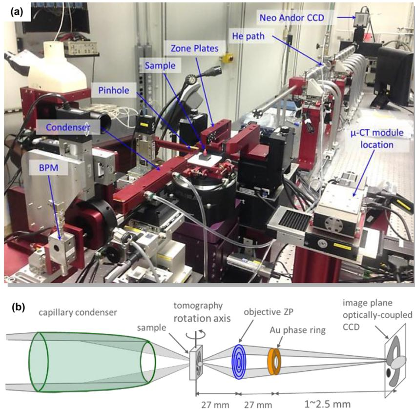
**Figure 3.30** a) Experimental setup of TXM. X-ray with a beamline 32-ID of the APS -ANL is focused on to the sample with a condenser where the field of view is increased. Pinhole removes the unfocused beam and the sample is rotated from 0 to 180 in 5 minutes. The detector system with scintillator screen converts X-rays to visible light and recorded by CCD camera on
