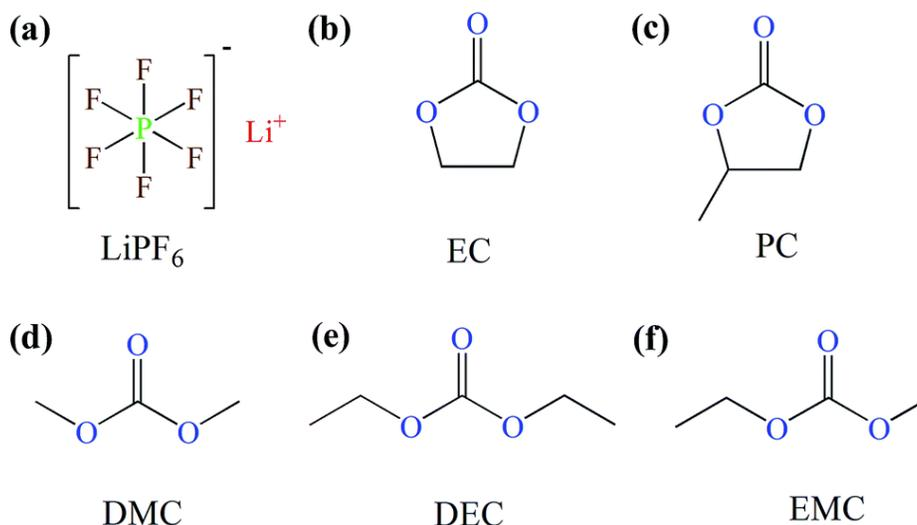
**Figure 1.9** Molecular structures of commonly used electrolyte salt and organic solvents in LIBs. (a)  $\text{LiPF}_6$  salt, (b) Ethylene Carbonate, (c) Propylene Carbonate, (d) Di Methyl Carbonate, (e) Di Ethylene Carbonate, (f) Ethyl Methyl Carbonate [24].
