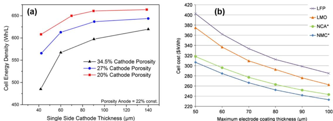
**Figure 1.17** Effect of cathode thickness in the LIB energy density: a) Increase in cathode thickness/ active material loading leads to increase in volumetric energy density. b) Similar trend is observed for four different cathodes showing reduction in cell cost and increase in areal capacity. Reprinted from [66], [96].
