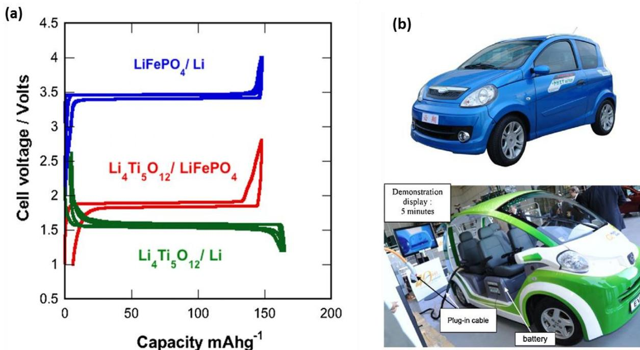
**Figure 1.8** a) Voltage–capacity cycle showing the charge-discharge plateau with much less polarization for LFP/Li, LTO/Li and LFP/LTO equipped with liquid electrolyte (1M LiPF<sub>6</sub>- EC-DEC). b) Electric cars equipped with C-LFP/LTO battery demonstrated the 5 minutes charging time with 500 V, 125 A charging station.
