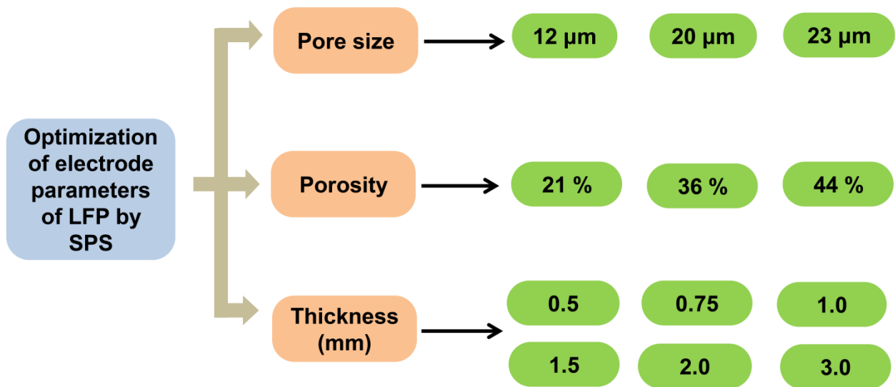
Figure 3.1 Schematic of optimization of electrode parameters for the thick binder free LFP electrodes obtained using SPS and templating approach.
