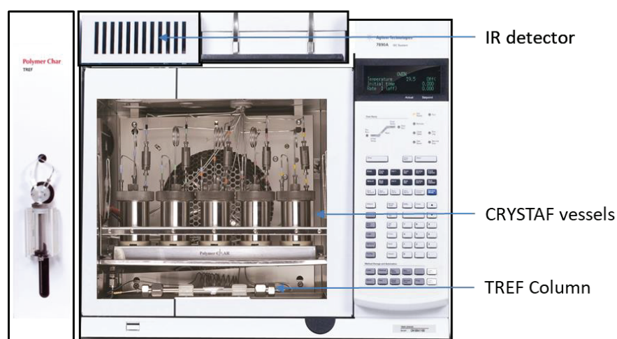
Figure 3-10: CRYSTAF-TREF instrument overview. CRYSTAF and TREF methods can be performed in the same instrument. CRYSTAF analyzes the sample during the crystallization step and TREF during the dissolution step.
