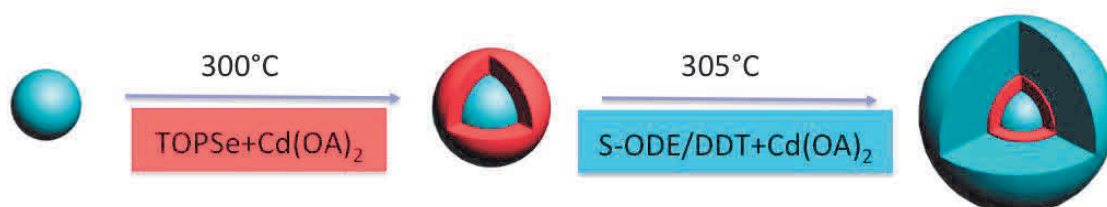
Figure 3.9. The protocol of spherical quantum wells synthesis
