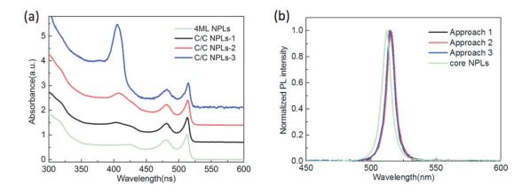
Figure 3.18 (a)Absorption spectra of CdSe/CdS core/crown NPLs with the crown increasing, (b) photoluminescence spectra of C/C NPLs synthesized by three methods with different crown size, comparing with core 4ML NPLs.
