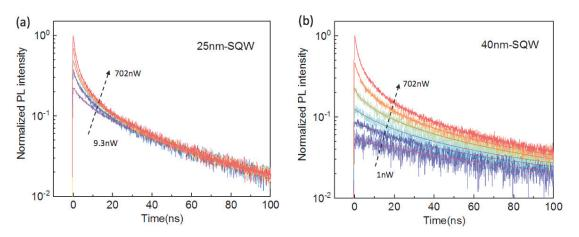
Figure 4.15 The PL decay curves of 25nm(a) and 40nm(b) diameter SQWs under various excitation powers are normalized at 100ns and 250ns to match the single exciton tail, compared to that of 15nm SQWs, the multiexcitons components are longer lived.
