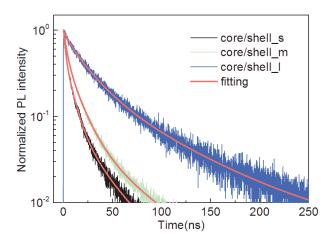
Figure 5.8 Normalized fluorescence decay curves of CdSe/CdZnS core/shell NPLs with different shell thickness in polymer under low intensity photoexcitation(defocusing), red lines are the triexponential fitting curves.
