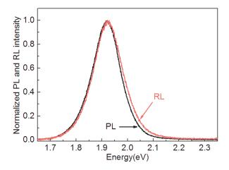
Figure 5.13 Normalized steady state PL and RL spectra for core/crown/shell CdSe/CdS/CdZnS NPLs. The power of photoexciton source is low with 405nm wavelength.
