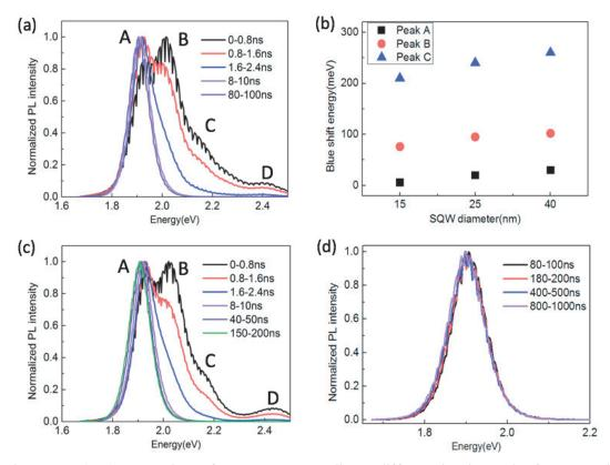
Figure 4.18 (a, c) Comparison of spectra corresponding to different time intervals of 25 nm and 40 nm SQWs at power 35.78 μW. (b) The energy shift of the different peaks with respect to single exciton peak for 15 nm, 25 nm and 40 nm SQWs. (d) Delayed emission at the late time of 40 nm SQWs.
