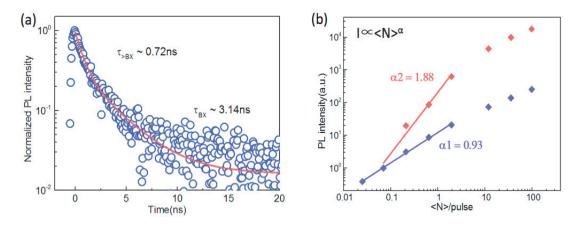
Figure 4.14 (a) Multiexcitons dynamics in 15nm SQWs obtained by subtracting the scaled single exciton contribution from high power decay (<N>~4), it can be fitted with two exponentials by 0.72ns and 3.14ns. (b) Power dependent integral PL intensity of fast component (red square) and slow component (purple square). Slow component shows a single exciton signature and the fast component follows an approximately quadratic dependence on power.
