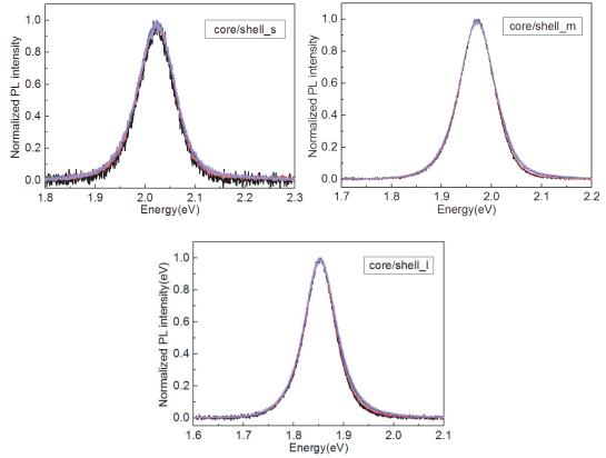
FigureA2.3 Emission spectra of CdSe/CdZnS nanoplatelets with varying shell thickness under varying laser power.
