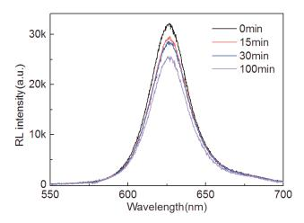
Figure 5.2 Radioluminescence spectra of C/S NPLs for different illuminated time. Excitation source: X-rays generated by 35kV voltage and 35mA current.
