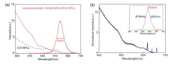
Figure 3.23 (a)Absorption and photoluminescence spectra comparison of core/shell (black dash line) and core/crown/shell NPLs (red solid line). (b)PLE of C/C/S NPLs with different thickness shell measured at different emission wavelengths.
