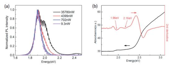
Figure 4.17 (a) Normalized time-resolved PL spectra in first 800ps as a function of power for drop-cast 15nm SQWs. The excitation wavelength is 405nm. (b) Absorption (black), and absorption second derivative (red) spectra of 15nm SQWs. The arrows mark the 1S<sub>e</sub>-1S<sub>h</sub>→1.96eV and 1P<sub>e</sub>-1P<sub>h</sub>→2.16eV transitions.
