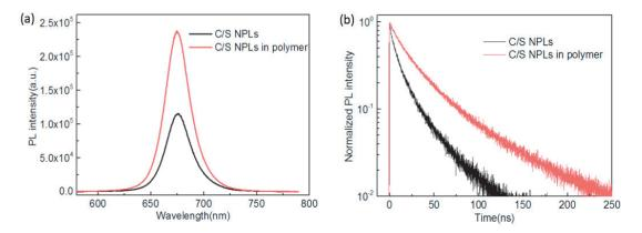
Figure 5.1 Comparison of the optical properties between core/shell NPLs film(black line) and core/shell NPLs in polymer film(red line). (a) PL spectra recorded under low intensity optical excitation. (b) PL decay curves of the peak wavelength excited by low intensity pulsed laser to avoid the formation of multiexcitons.
