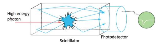
Figure 2.11 A simplified schematic representation of scintillation detector[60].
