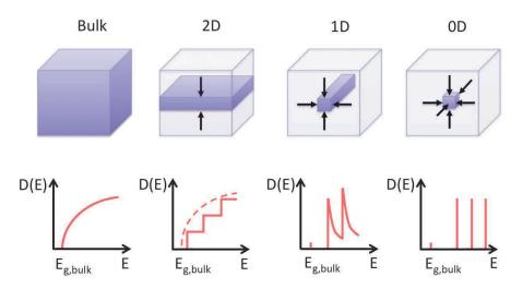
Figure 2.3 Schematic diagram of the density of states as a function of dimensionality. Bulk materials(3D) without quantum confinement effects in three dimensions; 2D refers to quantum wells with quantum confinement effects in only one dimension; 1D refers to rod-shaped or wire-shaped nanocrystals restricted in two dimensions; 0D mainly refers to quantum dots confined in three dimensions.
