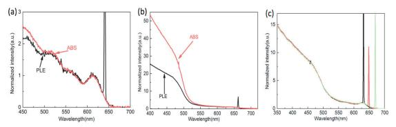
Figure 3.6 Comparison between ABS and PLE spectra. (a) without secondary nucleation and (b)with secondary nucleation. (c) taken at different emission wavelengths (the maximum of the emission, lower energy side and the higher energy side of the emission peak).
