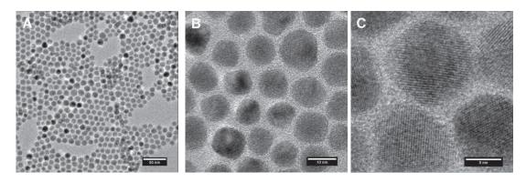
Figure 3.8 TEM images of nanoparticles at different magnifications: A.20000X, B.120000X, C.300000X.
