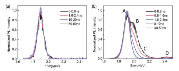
Figure 4.16 Comparison of time gated spectra corresponding to different time intervals of 15nm SQWs. (a) 9.3nW, (b) 35.78µW.
