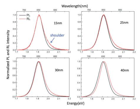
Figure 4.9 Steady-state PL and RL spectra of a series of drop-cast SQWs (15nm, 25nm, 30nm, 40nm). Excitation source: 405nm light emitting diode(black line) and X-rays illumination at a voltage of 35 kV (red line).
