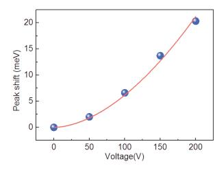
FigureA3.3 The red shift of PL peak position over applied voltage with respect to PL peak at 0V extracted from the spectra shown in Figure A3.2(b), fitted approximately with a quadratic function(~1.8) of applied voltage (red line)
