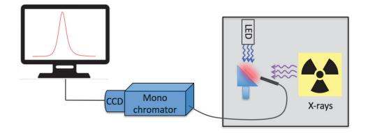
Figure 4.1 Schematic representation of radioluminescence and photoluminescence setup.
