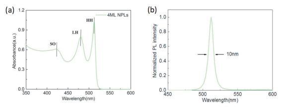
Figure 3.16 Absorption and normalized photoluminescence spectra of 4ML nanoplatelets. The excitation photon wavelength is 350nm.
