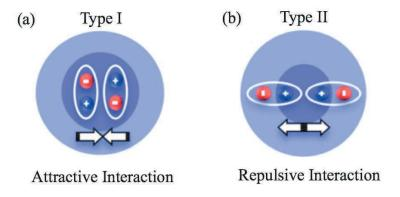
Figure 2.7 Schematic diagram of the exciton and exciton Coulomb interaction in nanocrystals: (a) attractive force, (b) replusive force[48].
