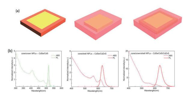
Figure 2.16 (a)Schematic illustration of core/crown, core/shell and core/crown/shell heterostructures. (b) Absorption and photoluminescence spectra of CdSe/CdS core/crown, CdSe/CdZnS core/shell and CdSe/CdZnS core/crown/shell NPLs, all of which are synthesized at our laboratories.
