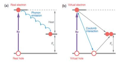
Figure 2.9 Schematic diagram of the carrier multiplication process. (a)Absorbing a photon with energy<2Eg, the electron dissipate the energy as heat. (b) After the absorption of a single high-energy photon(>2Eg), two excitons can be created through the Coulomb interaction in carrier multiplication processs[39].
