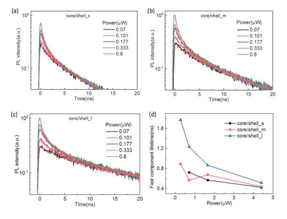
Figure 5.9 (a-c) Power dependent PL decay trace of core/shell NPLs with varying shell thickness, the traces are normalized at long tail to match the single exciton, highlighting the fast components arising at intense optical excitation. (d) The fitting lifetimes of the fast component as a function of power.
