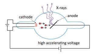
Figure 2.10 Schematic representation of X-rays tube
