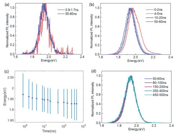
Figure 5.15 Normalized time gated PL for C/C/S NPLs in different time intervals as indicated in the figures under different power intensity. (a) Laser power is 4nW, (b) and (d) the slices for 0-60ns and after 60ns at laser power 33µW. (c) The position of the main peak and the change of the spectral width over time at laser power 33µW.
