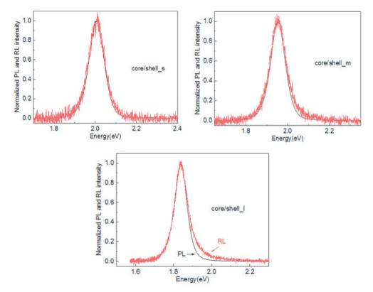
Figure 5.7 Normalized steady state PL and RL spectra comparison of core/shell CdSe/CdZnS NPLs with varying shell thickness.
