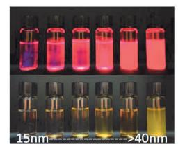
Figure 3.13 Image of different size SQWs from 15nm to 40nm dispersed in hexane or toluene with the same concentration under white light and UV light excitation.
