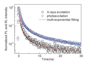
Figure 5.6 Normalized time-resolved fluorescence decay curves of CdSe/CdS core/crown NPLs under photoexcitation (23µW/cm<sup>2</sup>) (black circle) and X-rays excitation(blue circle), red line is the tri-exponential fitting curve. Photoexcitation is measured by defocusing of 405nm pulsed laser(repetition:500kHz) to avoid the multiexcitons.
