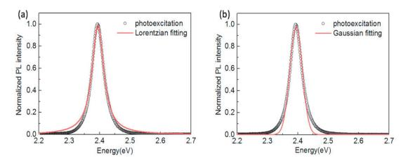
Figure 5.3 The photoluminescence spectrum is fitted by two different functions. (a) Lorentzian fitting, (b) Gaussian fitting.
