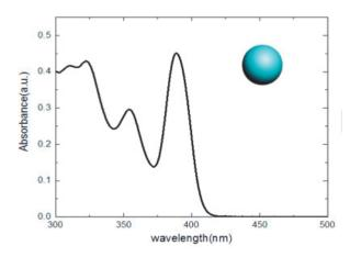
Figure 3.10 Absorption spectra of CdS seeds in hexane
