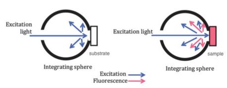
Figure 3.7 Schematic representation of absolute method with integrating sphere. Left: substrate spectrum measurement, right: sample spectrum measurement.
