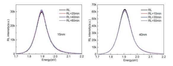
Figure 4.10 Emission intensity evolution with different X-rays illumination time of 15nm and 40nm SQWs. The X-ray images were recorded at a voltage of 35 kV. The accumulation time is 400s.
