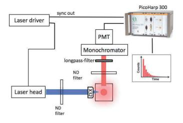
Figure 4.2 Schematic representation of photoluminescence decay curve measurement setup.
