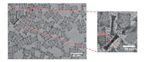
Figure 3.24 TEM image of core/crown/shell CdSe/CdS/CdZnS NPLs.
