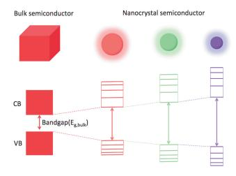
Figure 2.1 Schematic representation of quantum confinement effect: a bulk semiconductor with continue energy band and a fixed energy gap E<sub>g,bulk</sub>, while NCs possess discrete energy levels and the band gap energy increases with decreasing size.
