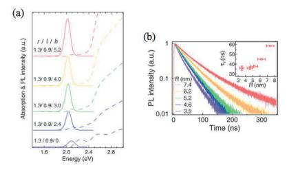
Figure 2.14 (a)Absorption and photoluminescence spectra of different shell thickness SQWs(r: CdS core; l: CdSe well; h: CdS shell), (b) The evolution of ensemble PL decay dynamics with shell thickness (inset: single-exciton radiative recombination lifetime; R is the total size)[81].
