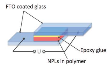
FigureA3.1 Schematic representation of the device for applying voltage on NPLs: CdSe/CdZnS NPLs in polymer is sandwished between two FTO electrodes coated on glass, epoxy glue is used to attach the second electrode.
