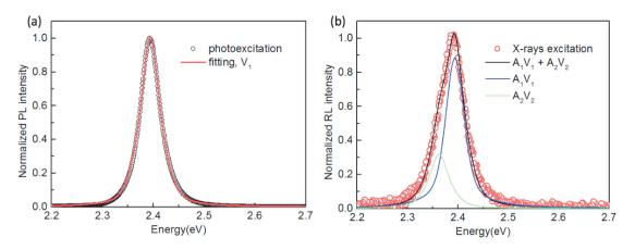
Figure 5.4 The comparison between PL and RL spectra and their fitting line shape with pseudo-Voigt function. PL was measured at low power to avoid the multiexcitons generation. (a) PL spectrum shows a single symmetric peak. And the RL spectrum is fitted by the sum of two components, y=A<sub>1</sub>V<sub>1</sub>+A<sub>2</sub>V<sub>2</sub>, the corresponding fitting of V<sub>1</sub>(blue line) and V<sub>2</sub>(green line) are also shown in the Figure(b).
