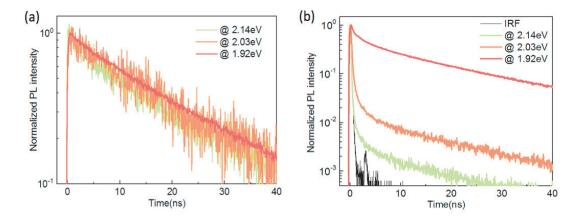
Figure 4.12 Decay dynamics measured at three different energy positions of a drop-cast 15nm diameter SQWs. (a)  $<N> \sim 0.003$ , (b)  $<N> \sim 4$ . Black curve in (b) is the instrument response function (IRF).
