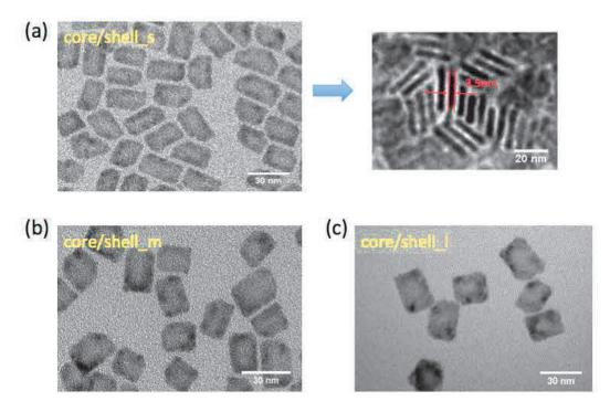
Figure 3.22 TEM images of different thicknesses core/shell CdSe/CdZnS NPLs. (a) and (b) are core/shell\_s, the arrow shows the vertical thickness is around 3.5nm, (c) and (d) are core/shell\_m and core/shell\_l, respectively.
