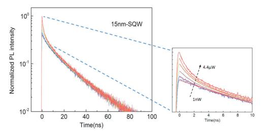
Figure 4.13 The PL decay curves of 15nm diameter SQWs under various excitation powers are normalized at 60ns to match the single exciton tail, highlighting the fast multiexcitons component at early time.
