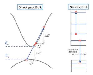
Figure 2.6 Schemes showing the difference between Auger recombination process in direct gap bulk (left) and NCs (right) semiconductors.  $\Delta E$  and  $\Delta p$  present the change of energy and momentum, respectively. E<sub>c</sub> and E<sub>v</sub> are the edge of conduction and valence bands. Compared to bulk material, the requirement of momentum conservation is largely relaxed in NCs and Auger recombination occurs efficiently for band edge carriers[18].
