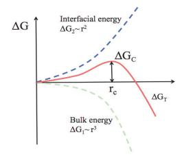
Figure 3.1 Red curve is the total Gibbs free energy as a function of the nuclei radius.  $\Delta G_c$  is the homogeneous nucleation energy barrier, and  $r_c$  is the critical radius. The bulk term  $\Delta G_1$  that scales with  $r^3$  is plotted in green. The interfacial energy  $\Delta G_2$  is the blue curve that is proportional to surface area.
