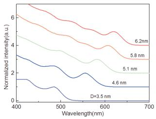
Figure 3.4 Evolution of the absorption spectra with increasing size of CdS/CdSe quantum dots, which are synthesized in our laboratory. Size is calculated by the precursors used
