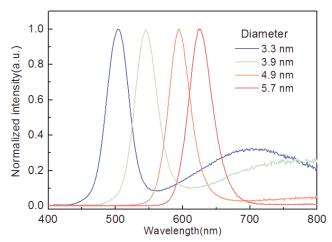
Figure 3.5 Evolution of the photoluminescence spectrum with increasing size of CdS/CdSe quantum dots, which are synthesized in our laboratory. Size is calculated by the precursors used.
