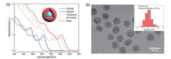
Figure 3.11 (a)Absorption spectrum of CdS/CdSe in hexane: variety color curves represent different aliquots taken during size growing, showing a red shift; (b)TEM image of CdS/CdSe at 400000X magnification, inset is the histogram of size distribution of ~100 particles.
