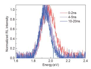
Figure 5.16 Normalized RL spectra for C/C/S NPLs in different time intervals as indicated in the figures under X-rays excitation with 30kV accelerating voltage.
