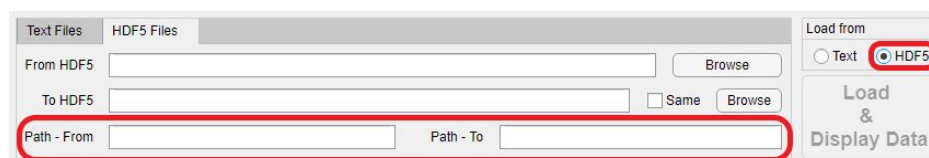
Figure 6: Paths to the From and To data, inside the HDF5 files, should be put in the boxes circled in red.
