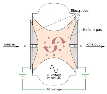
Figure 23. Ion trap set-up
