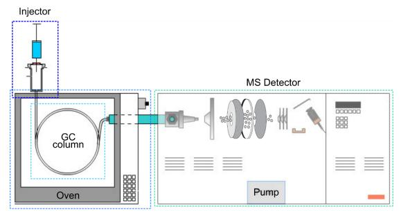
Figure 22. GC-MS schema equipped with a quadrupole ion trap
