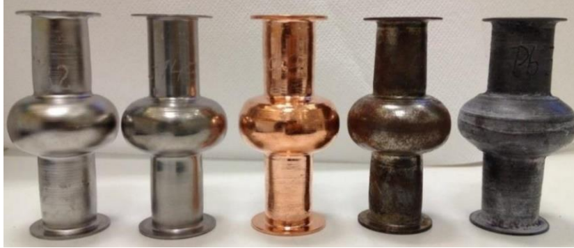
Figure 1.14: Seamless 6 GHz cavities fabricated at INFN LNL with spinning and different materials [71].
