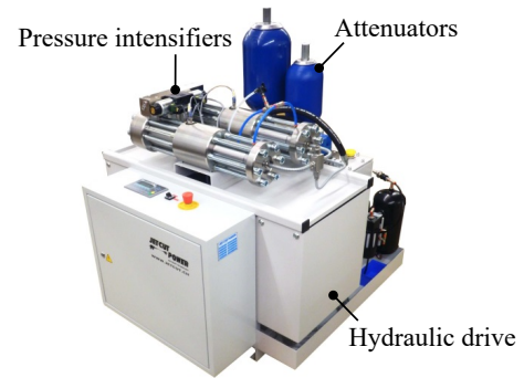
Figure 1.1 – Example of a conventional high-pressure pump (Type JPC 22 LC): hydraulically driven pressure intensifiers with two single acting pistons. 1
