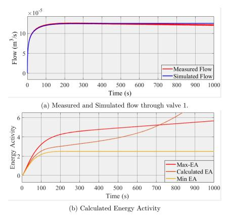
Figure 5.12: Flow through valve 1 and Energy Activity for two tank system undergoing leakage in tank 1.
