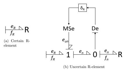
Figure A.5: Uncertainty modelling of an R-element in resistive causality.
