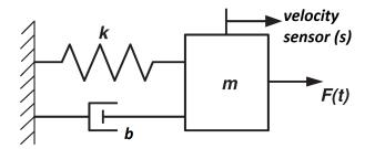
Figure 4.3: Spring Mass Damper System.
