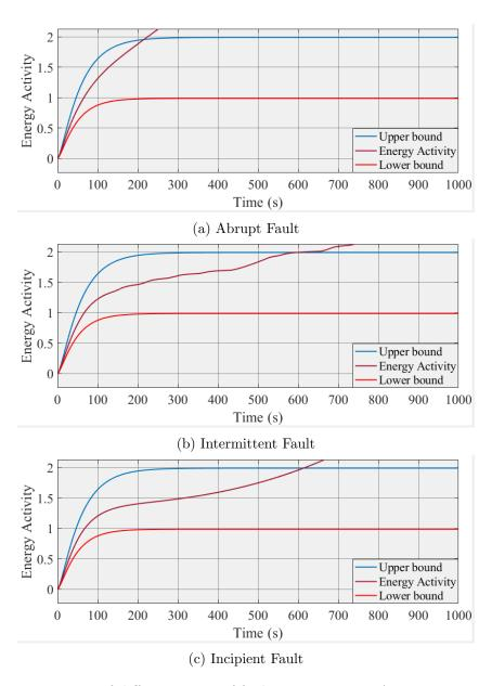
Figure 5.10: Detection of different types of faults using Energy Activity in integral form.
