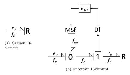
Figure A.6: Uncertainty modelling of an R-element in conductive causality.
