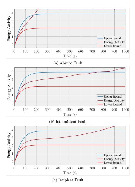
Figure 5.11: Detection of different types of faults using Energy Activity in dual (differential + integral) form.
