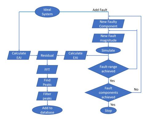
Figure 4.1: Generation of fault signature database.
