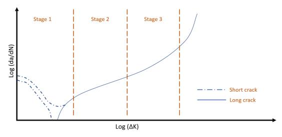
Figure 2.3: Fatigue crack graoth.
