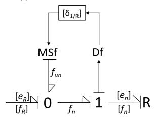
(b) Conductive R-element in interval form.
