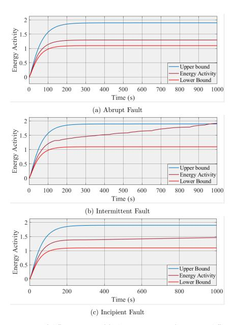
Figure 5.9: Detection of different types of faults using Energy Activity in differential form.
