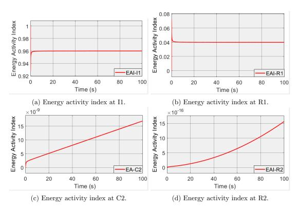
Figure 3.6: Energy Activity Index of elements in circuit.
