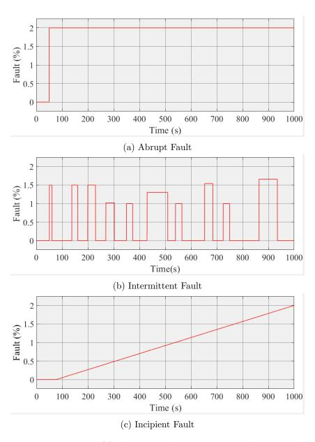
Figure 5.7: Various types of faults measured as percentage change in ideal flow.
