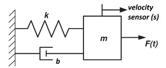
Figure A.7: Spring Mass Damper System.
