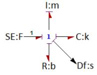
Figure 4.4: Bond Graph of Spring Mass Damper System.
