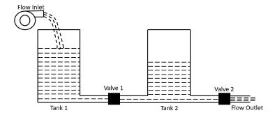
Figure 5.2: Schematic diagram of a two tank system.
