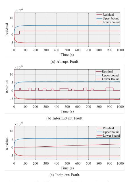
Figure 5.8: Residuals generated for different types of faults using ARRs from LFT-Bond Graph.
