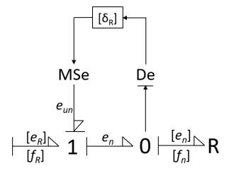
(a) Resistive R-element in interval form.
