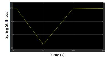
Figure 4.5: Fault as a variation in spring stiffness.
