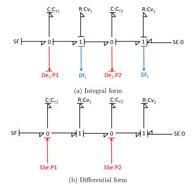
Figure 5.4: Bond graph models of two-tank system.
