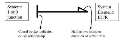
Figure A.1: General structure of a bond.
