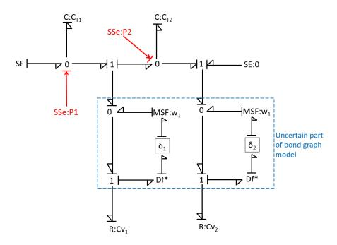
Figure 5.5: LFT-Bond Graph model of 2 tank system.
