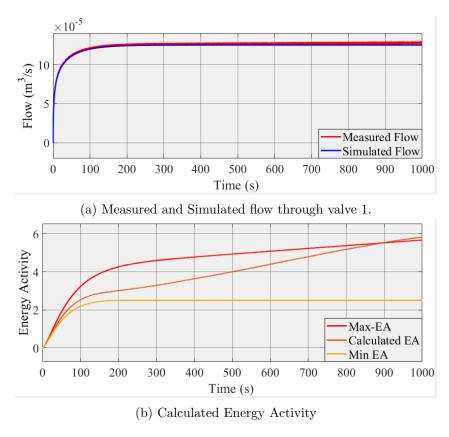
Figure 5.13: Flow through valve 1 and Energy Activity for two tank system with faulty pump.
