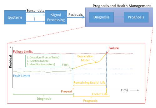
Figure 1.2: Schematic of Condition Based Maintenance.
