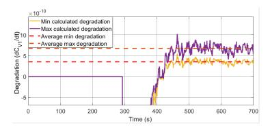
Figure 5.15: Valve degradation from prognosis.
