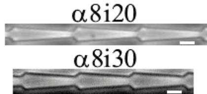
Figure 3.16: Images of \alpha 8i20 and \alpha 8i30 ratchet microchannels. Scale bar 10\mu\text{m} .
