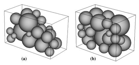
Figure 4.4: Illustration of DSBH's behavior on SYS1 instance (Set1: (a) the starting solution with a length equal to 11.5051 and (b) the best solution's structure and its length (9.2431) reached by DSBH.
