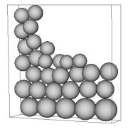
Figure 6.1: Illustration of BGP's solution for the instance KBG2 containing 30 spheres (the density of the provided solution is equal to 30.0709%).
