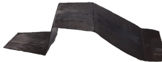
Figure 5.28: Unified simulation of a UD ply on Omega mold: Final deformed shape from the experiments
