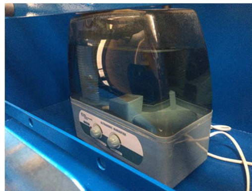
Figure 5-56: Humidifier by ultrasound (cold cell)
