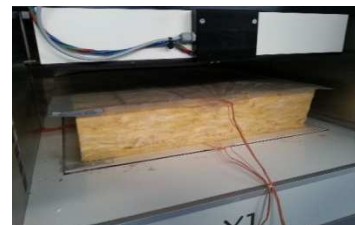
Figure 3-32: Image of sample inside guarded hot plate (TLP 500 X1)
