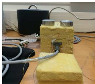
Figure 3-21: Image of the sensor inside sample
