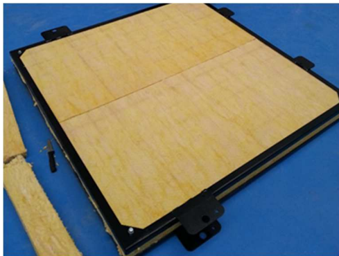
Figure 5-25: manufacturing glass wool wall and fixing it on the frame.
