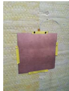
Figure 5-27: flowmeter to evaluate the flux rate.
