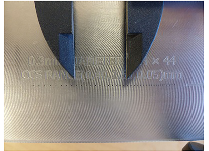
Fig. 9. Stainless steel block containing a set of 41 close aligned SDHs ( \varnothing 0.3 mm), with decreasing separation distance from left to right. The black elements are the jaws of a sliding caliper, showing a 1-inch distance.
