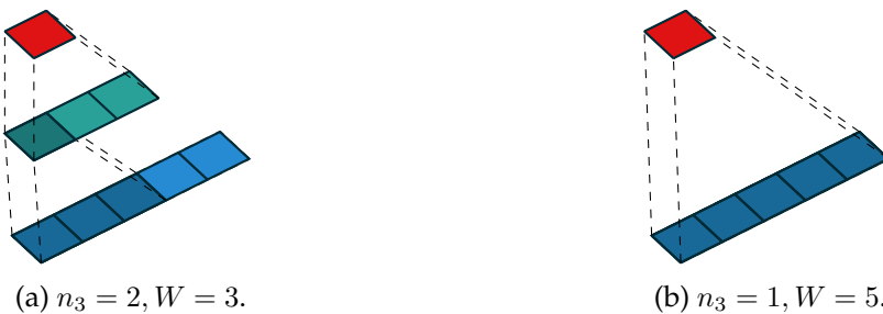
Figure 4.2: A 1D receptive field of size D = 5 , captured either by one or two convolution layers. Inspired from Dumoulin et al. [DV16].
