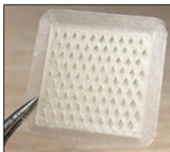
Figure IV.11: Lattice support designed by 3D-printing.
