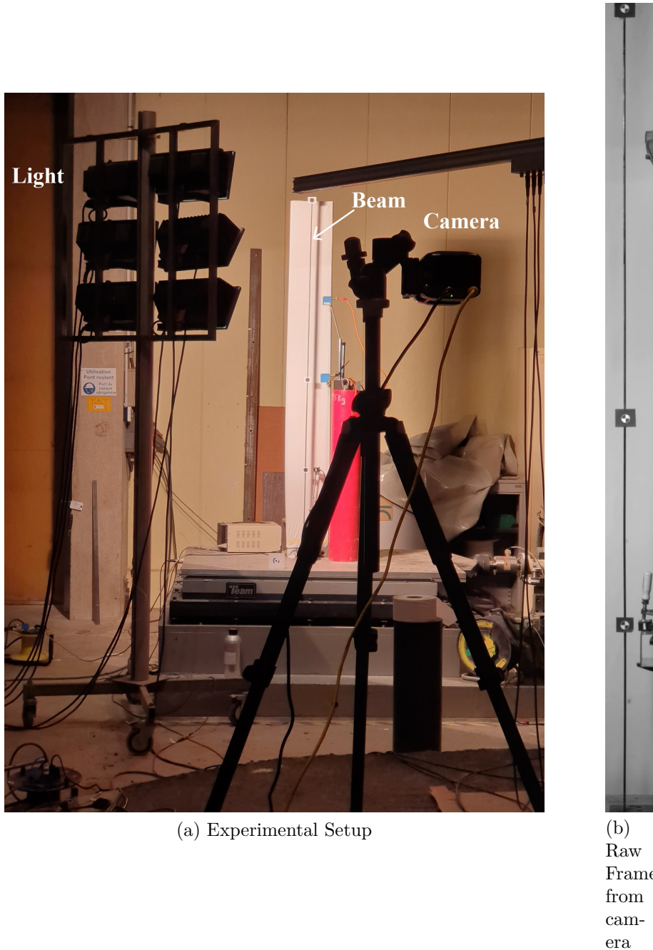
Figure 5.15 – Setup for motion extraction of three targets pasted on the beam with white background of beam test oscillated by random Gaussian signal
