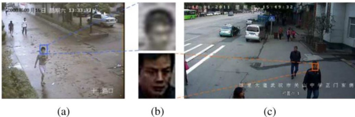
Figure 1.6: Typical frames from surveillance videos. (a) and (c) are the surveillance images from a camera with CIF size (pixels) and a camera with 720P size (pixels) respectively; (b) shows two noisy interested faces extracted from (a) and (c) [73].
