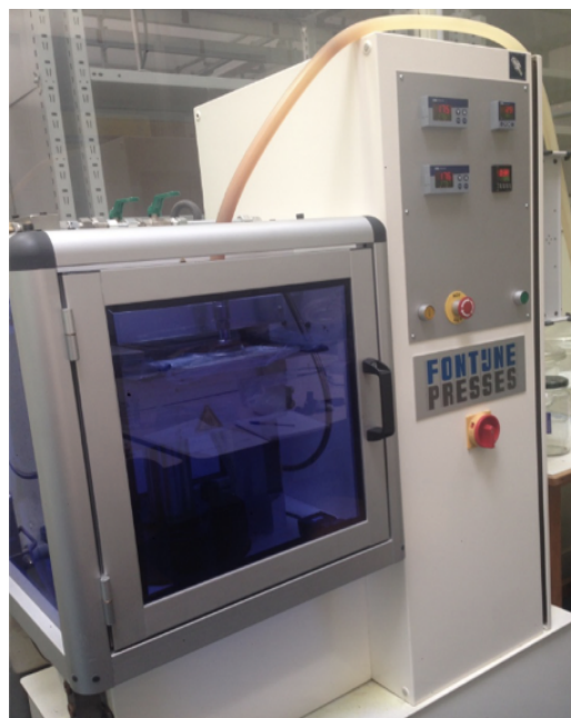
Figure 3.4 – Compression molding and heating press LabPro TP 1000 from Fontijne Presses
