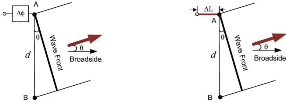
Figure 1.3 Beam steering (a) using a phase shifter, and (b) using a delay line. [2]
