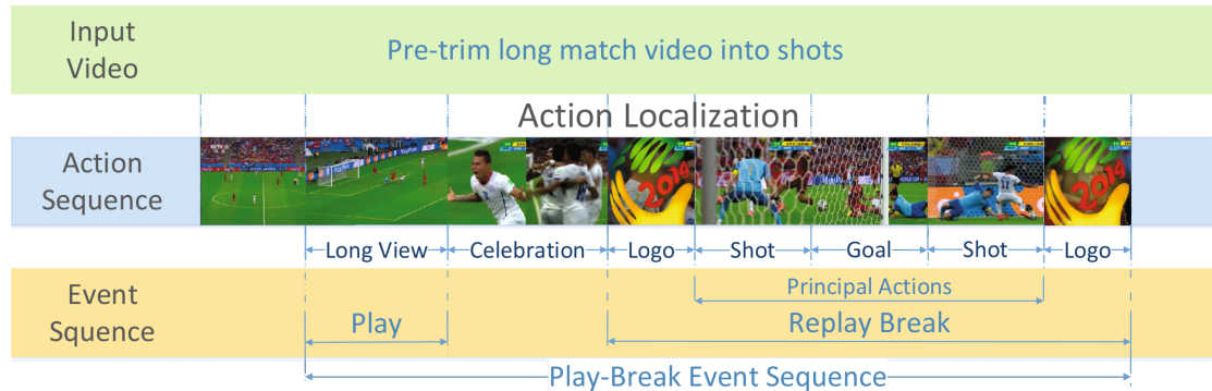
FIGURE 2.14: Play and break example. A long view scene (Play) followed by non-long view actions (break), and shot sequences surrounded by a pair of replay logos. Image from [9]
