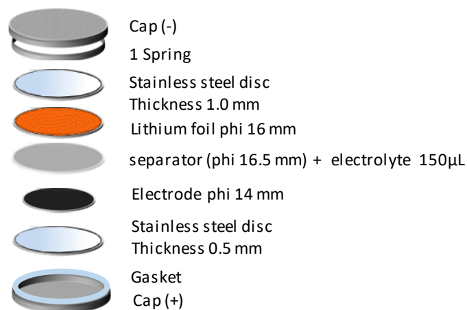
Figure II-4 : An illustrative schema of coin cell components in the order of their assembly.
