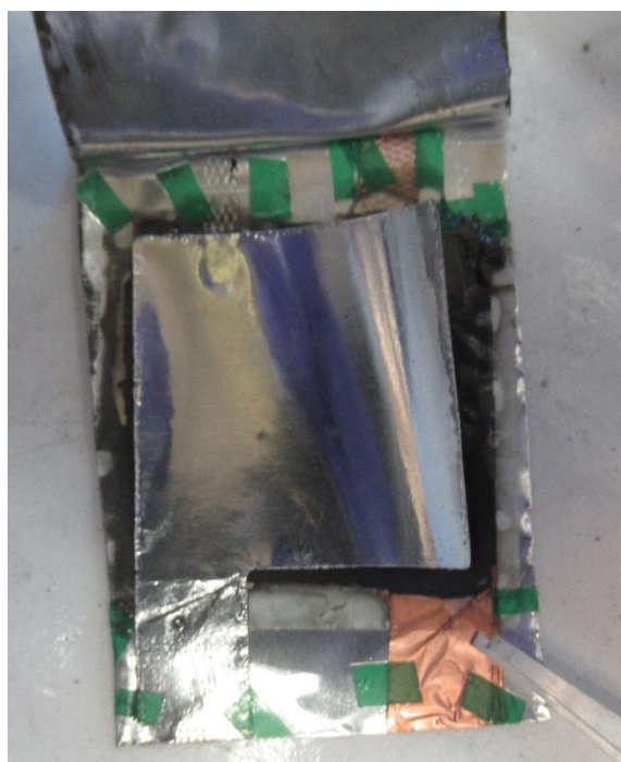
Figure II-25: Sandwich of the dismantled 4-electrode design cell.
