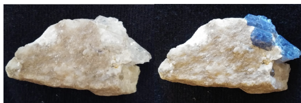
Figure I.22: Colouration of tenebrescent marialite under UV light irradiation. It goes from colourless (left) to blue (right).
