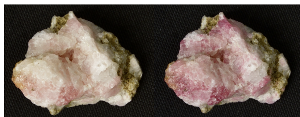
Figure I.20: Colouration of tenebrescent tugtupite under UV light irradiation. It goes from colourless (left) to red (right).
