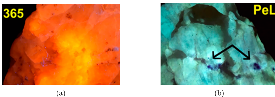
Figure VI.1: (a) Fluorescence of a tenebrescent sodalite mineral after UV irradiation (365 nm). (b) Persistent luminescence at 490 nm of a sodalite mineral after UV irradiation (275 nm).[1]
