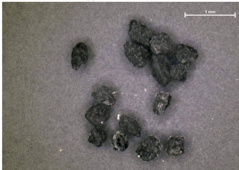
(b) Carbon C filled with NaClO<sub>4</sub> from a 56 wt% aqueous solution.
