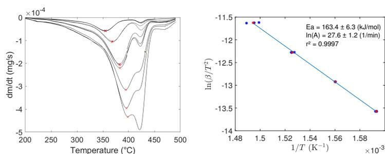
Figure H.11: TGA results (at 0.5, 1, 2, 4 and 7 K/min) of a physical mixture of carbon C and sodium perchlorate at 1.79 g/g, both milled and sieved between 25 and 50  $\mu\text{m}$ , and decomposition kinetics modelling.
