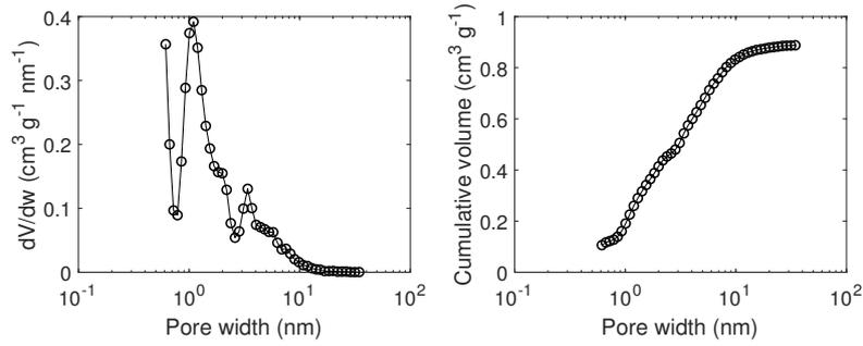
Figure C.10: Pore size distribution modelled by QSDFT based on N<sub>2</sub> adsorption/desorption isotherm for carbon C-R600.
