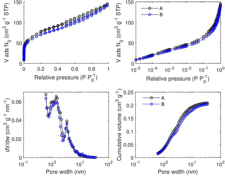
Figure F.18:  $N_2$  adsorption/desorption isotherm data measured at 77 K and pore size analysis by equilibrium QSDFT for carbon BPL-37 filled with  $NaClO_4$  from a 56 wt% aqueous solution. A and B are repetitions (from the synthesis).
