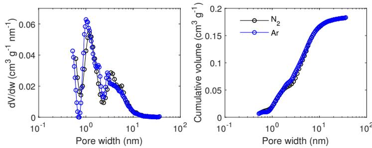
Figure D.9: Pore size distribution modelled by QSDFT based on N<sub>2</sub> at 77 K and Ar at 87 K adsorption/desorption isotherms for carbon C-R300 filled with NaClO<sub>4</sub> from a 56 wt% aqueous solution.
