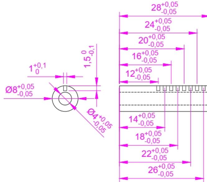
Figure A.3: Plan of the confinement tubes for charges with a diameter of 4 mm (dimensions in mm).
