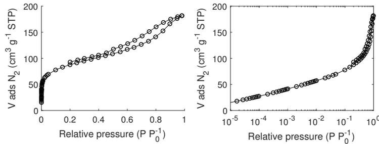
Figure D.10: N<sub>2</sub> adsorption/desorption isotherm of carbon C-600 filled with NaClO<sub>4</sub> from a 56 wt% aqueous solution measured at 77 K.
