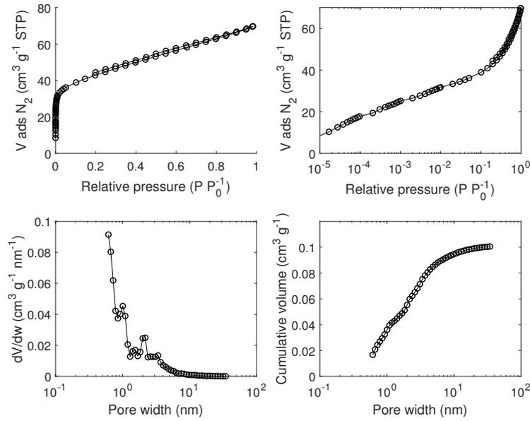
Figure F.19: N<sub>2</sub> adsorption/desorption isotherm data measured at 77 K and pore size analysis by equilibrium QSDFT for carbon FY5 filled with NaClO<sub>4</sub> from a 40 wt% aqueous solution.
