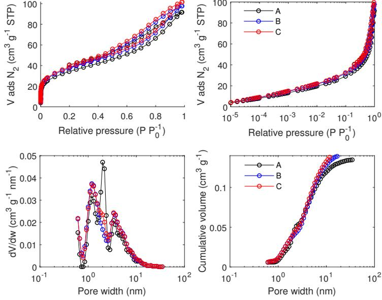
Figure F.2:  $N_2$  adsorption/desorption isotherm data measured at 77 K and pore size analysis by equilibrium QSDFT for carbon C filled with  $NaClO_4$  from a 50 wt% aqueous solution. A, B and C are repetitions (from the synthesis).
