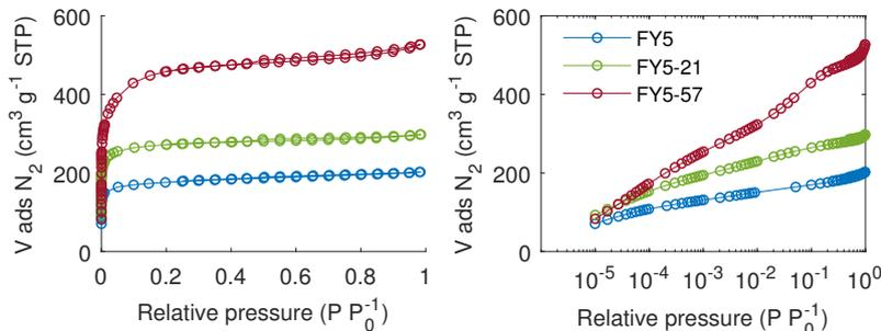
Figure 3.10: N<sub>2</sub> adsorption isotherm measured at 77 K of carbon FY5 and its overactivated derivatives.
