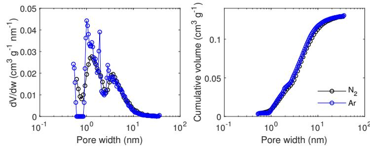
Figure D.6: Pore size distribution modelled by QSDFT based on  $\text{N}_2$  at 77 K and  $\text{Ar}$  at 87 K adsorption/desorption isotherms for carbon C filled with  $\text{NaClO}_4$  from a 60 wt% aqueous solution.
