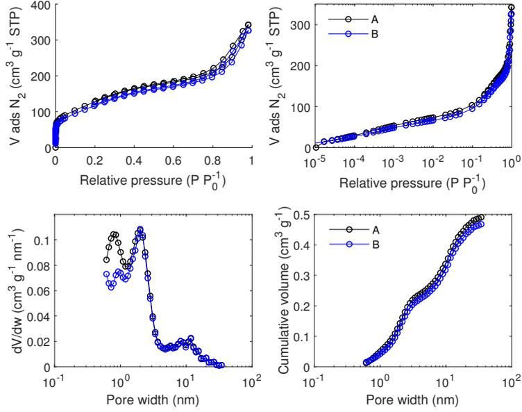
Figure F.8:  $N_2$  adsorption/desorption isotherm data measured at 77 K and pore size analysis by equilibrium QSDFT for carbon F5001 filled with  $NaClO_4$  from a 50 wt% aqueous solution. A and B are repetitions (from the synthesis).
