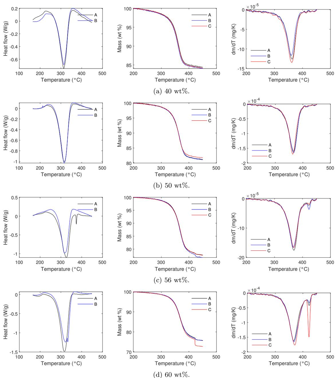
Figure H.7: DSC (left), TGA (middle) and DTG (right) results of carbon FY5 filled with NaClO<sub>4</sub> from solution at different concentrations (40, 50, 56 and 60 wt%).
