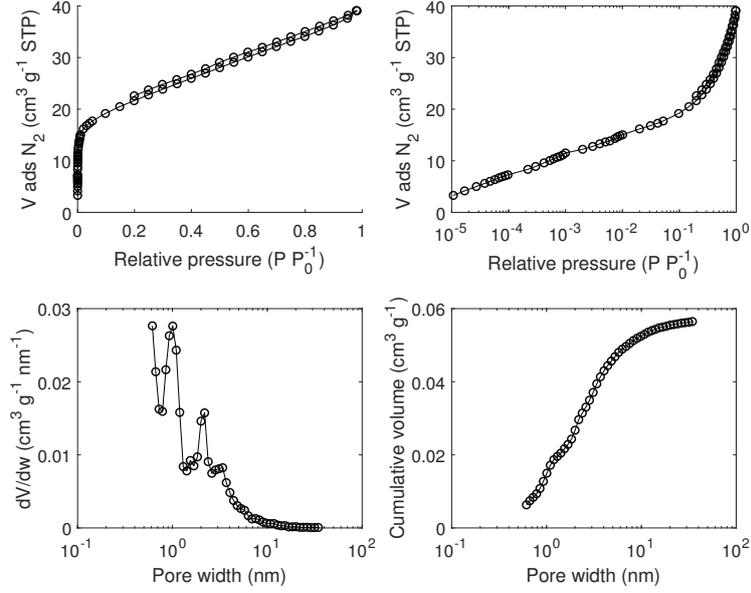
Figure F.21: N<sub>2</sub> adsorption/desorption isotherm data measured at 77 K and pore size analysis by equilibrium QSDFT for carbon FY5 filled with NaClO<sub>4</sub> from a 56 wt% aqueous solution.
