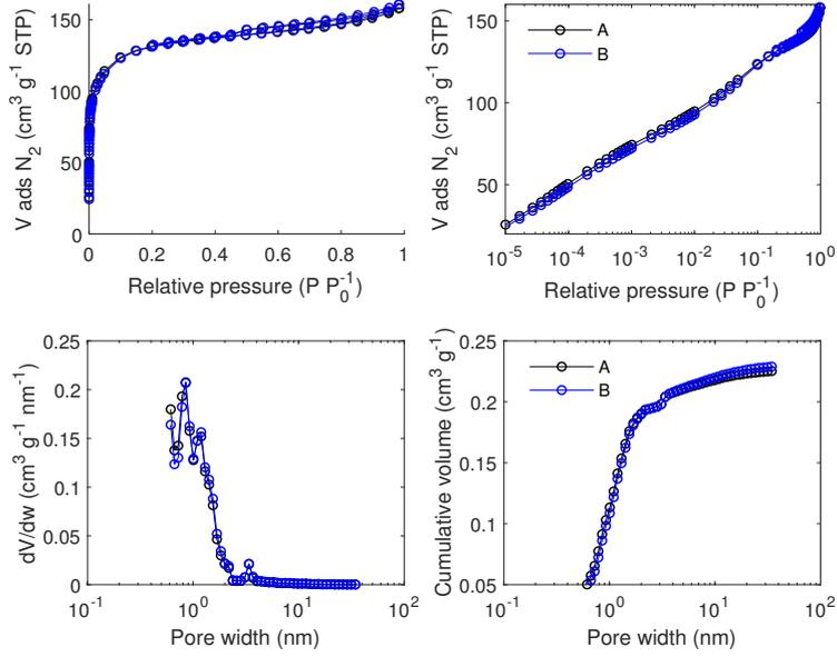
Figure F.24: N<sub>2</sub> adsorption/desorption isotherm data measured at 77 K and pore size analysis by equilibrium QSDFT for carbon FY5-57 filled with NaClO<sub>4</sub> from a 56 wt% aqueous solution. A and B are repetitions (from the synthesis).
