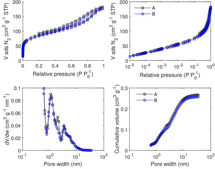
Figure F.6: N<sub>2</sub> adsorption/desorption isotherm data measured at 77 K and pore size analysis by equilibrium QSDFT for carbon C-R600 filled with NaClO<sub>4</sub> from a 56 wt% aqueous solution. A and B are repetitions (from the synthesis).
