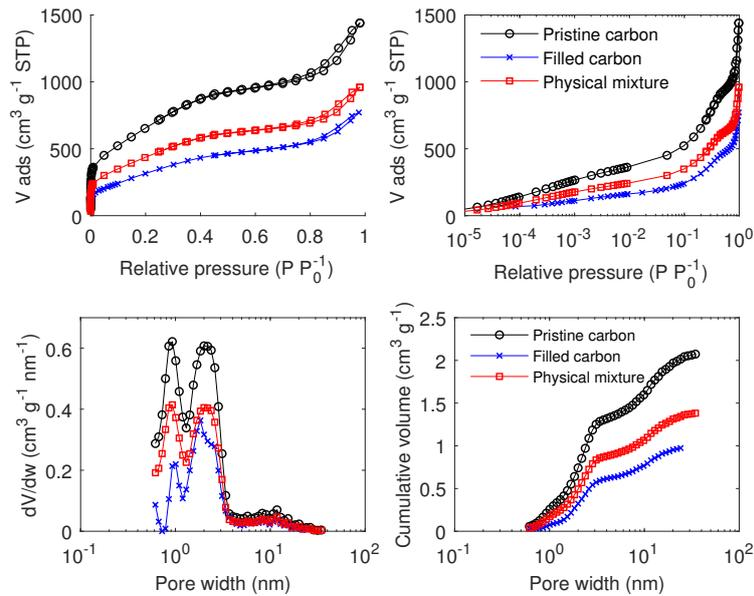
Figure 3.26: Comparison between  $\text{N}_2$  adsorption isotherm and pore size analysis of the pristine carbon, the filled carbon and the corresponding theoretical physical mixture for carbon F5001 filled with  $\text{NH}_4\text{ClO}_4$ .
