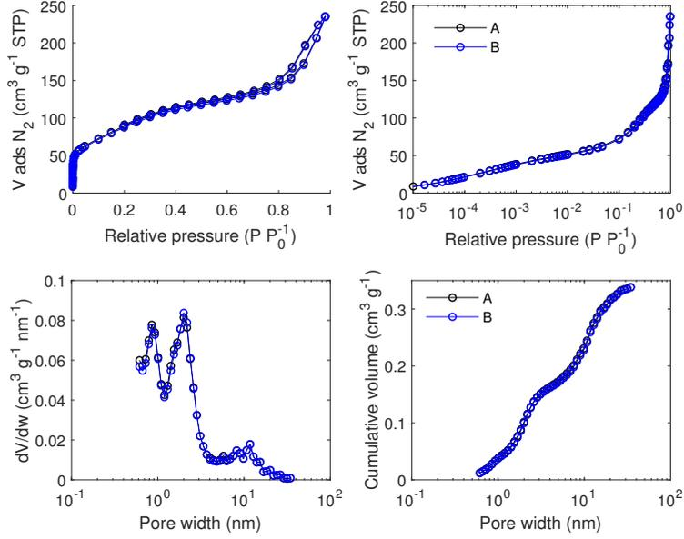
Figure F.12:  $N_2$  adsorption/desorption isotherm data measured at 77 K and pore size analysis by equilibrium QSDFT for carbon F5001-HN filled with  $NaClO_4$  from a 56 wt% aqueous solution. A and B are repetitions (from the synthesis).
