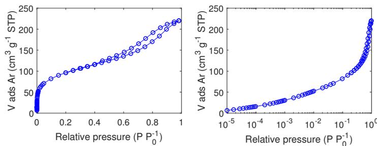
Figure D.11: Ar adsorption/desorption isotherm of carbon C-R600 filled with NaClO<sub>4</sub> from a 56 wt% aqueous solution measured at 87 K.
