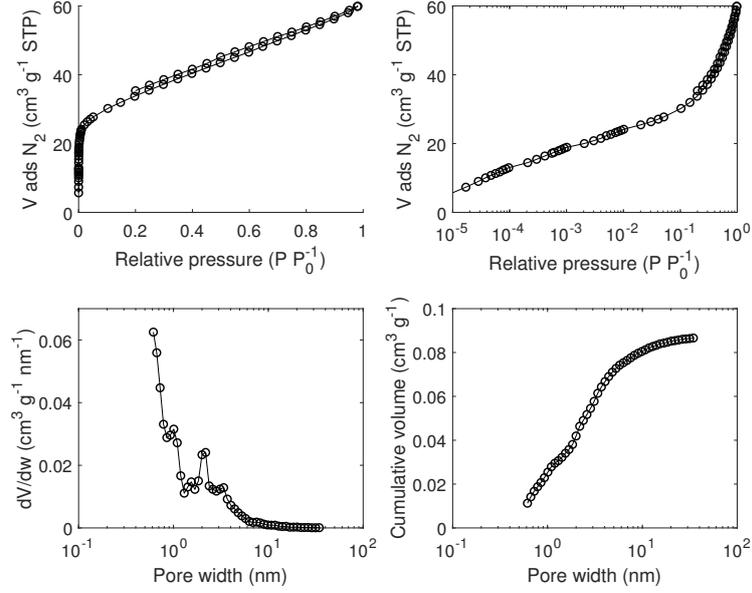
Figure F.20: N<sub>2</sub> adsorption/desorption isotherm data measured at 77 K and pore size analysis by equilibrium QSDFT for carbon FY5 filled with NaClO<sub>4</sub> from a 50 wt% aqueous solution.
