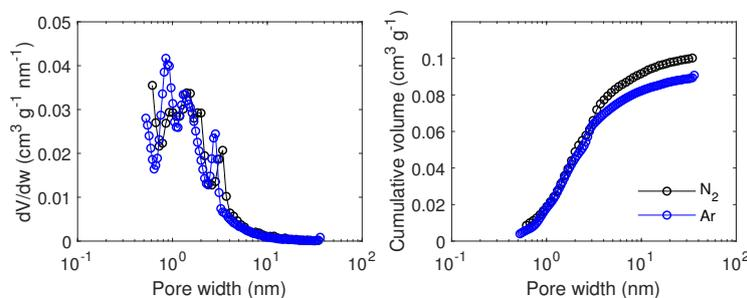
Figure D.30: Pore size distribution modelled by QSDFT based on  $\text{N}_2$  at 77 K and  $\text{Ar}$  at 87 K adsorption/desorption isotherms for carbon BPL filled with  $\text{NaClO}_4$  from a 60 wt% aqueous solution.
