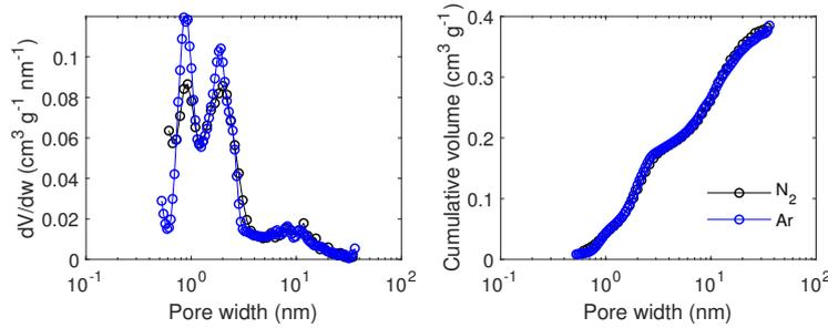
Figure D.18: Pore size distribution modelled by QSDFT based on  $\text{N}_2$  at 77 K and  $\text{Ar}$  at 87 K adsorption/desorption isotherms for carbon F5001 filled with  $\text{NaClO}_4$  from a 60 wt% aqueous solution.
