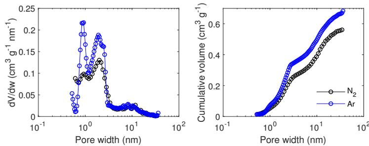
Figure D.15: Pore size distribution modelled by QSDFT based on N<sub>2</sub> at 77 K and Ar at 87 K adsorption/desorption isotherms for carbon F5001 filled with NaClO<sub>4</sub> from a 40 wt% aqueous solution.
