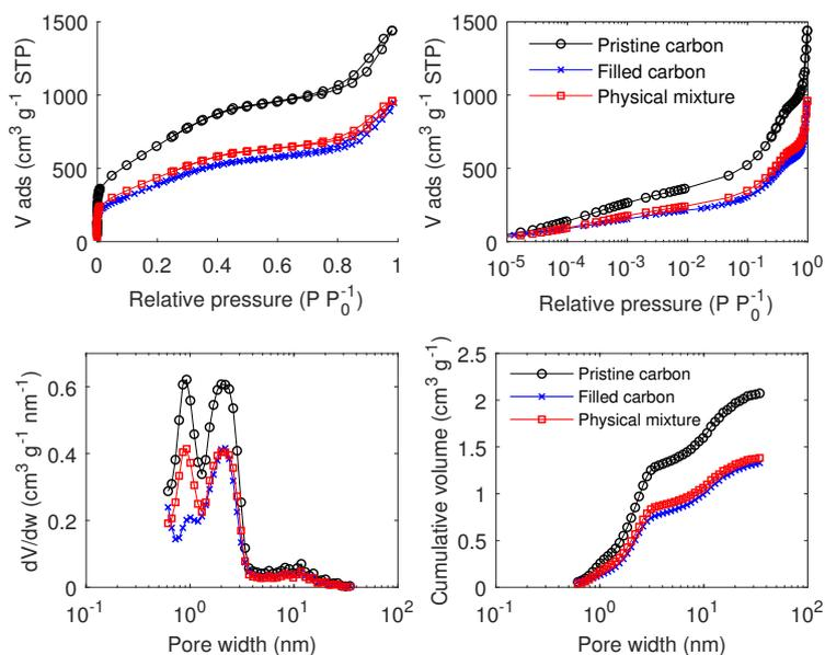
Figure 3.22: Comparison between  $N_2$  adsorption isotherm and pore size analysis of the pristine carbon, the filled carbon and the corresponding theoretical physical mixture for carbon F5001 filled with  $KNO_3$ .
