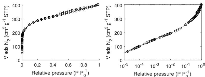
Figure C.28: N<sub>2</sub> adsorption/desorption isotherm of carbon BPL-18 measured at 77 K.
