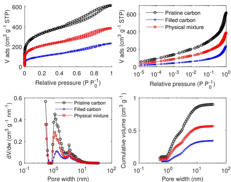
Figure 3.20: Comparison between  $N_2$  adsorption isotherm and pore size analysis of the pristine carbon, the filled carbon and the corresponding theoretical physical mixture for carbon C filled with  $KNO_3$ .
