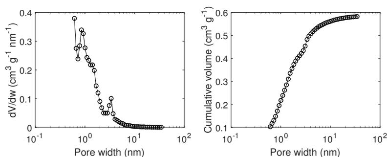
Figure C.29: Pore size distribution modelled by QSDFT based on N<sub>2</sub> adsorption/desorption isotherm for carbon BPL-18.
