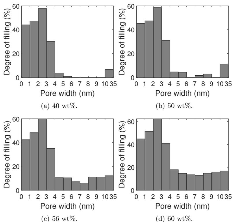
Figure 3.32: Influence of the solution concentration on the degree of pore filling for carbon F5001 filled with NaClO<sub>4</sub>.
