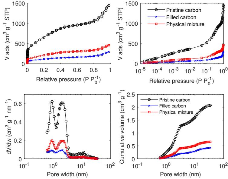
Figure 3.18: Comparison between  $N_2$  adsorption isotherm and pore size analysis of the pristine carbon, the filled carbon and the corresponding theoretical physical mixture for carbon F5001 filled with  $NaClO_4$ .
