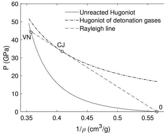
Figure 1.2: Hugoniot curves of pentaerythritol tetranitrate (PETN). The initial state (0) is characterized by a specific mass of  $1.77 \text{ g/cm}^3$ . The Chapman-Jouguet (CJ) and von Neumann (VN) states are represented. Numerical data from the literature [8] are used in equations (1.7), (1.11), and (1.8).
