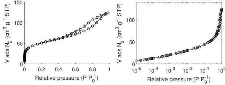
Figure D.7: N<sub>2</sub> adsorption/desorption isotherm of carbon C-R300 filled with NaClO<sub>4</sub> from a 56 wt% aqueous solution measured at 77 K.
