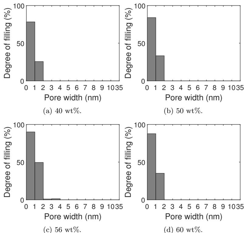
Figure 3.34: Influence of the solution concentration on the degree of pore filling for carbon FY5 filled with NaClO<sub>4</sub>.
