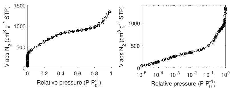
Figure C.20: N<sub>2</sub> adsorption/desorption isotherm of carbon F5001-HN measured at 77 K.
