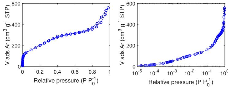
Figure D.14: Ar adsorption/desorption isotherm of carbon F5001 filled with NaClO<sub>4</sub> from a 40 wt% aqueous solution measured at 87 K.
