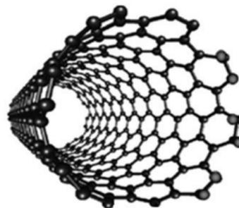
(d) Example of carbon nanotube (adapted from [25]).
