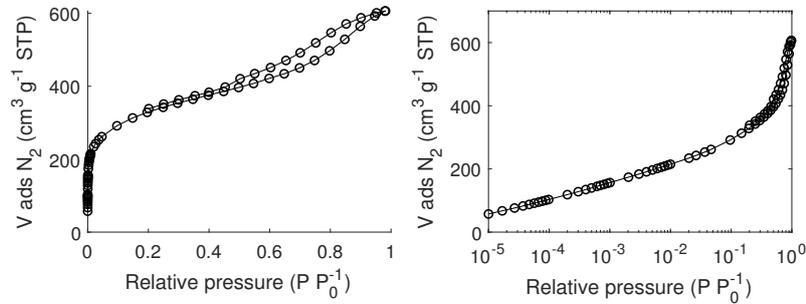
Figure C.9:  $N_2$  adsorption/desorption isotherm of carbon C-R600 measured at 77 K.
