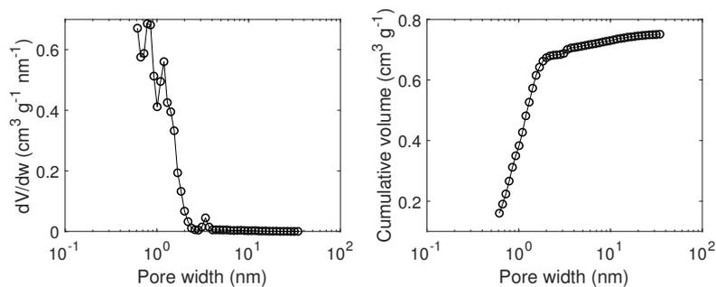
Figure C.43: Pore size distribution modelled by QSDFT based on N<sub>2</sub> adsorption/desorption isotherm for carbon FY5-57.
