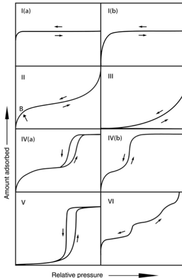
Figure A.2: Classification of gas adsorption isotherm [26].
