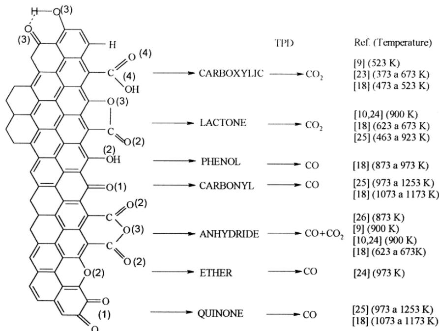
Figure 2.1: Decomposition temperatures of the oxygen-containing functional groups on a carbon surface [83].
