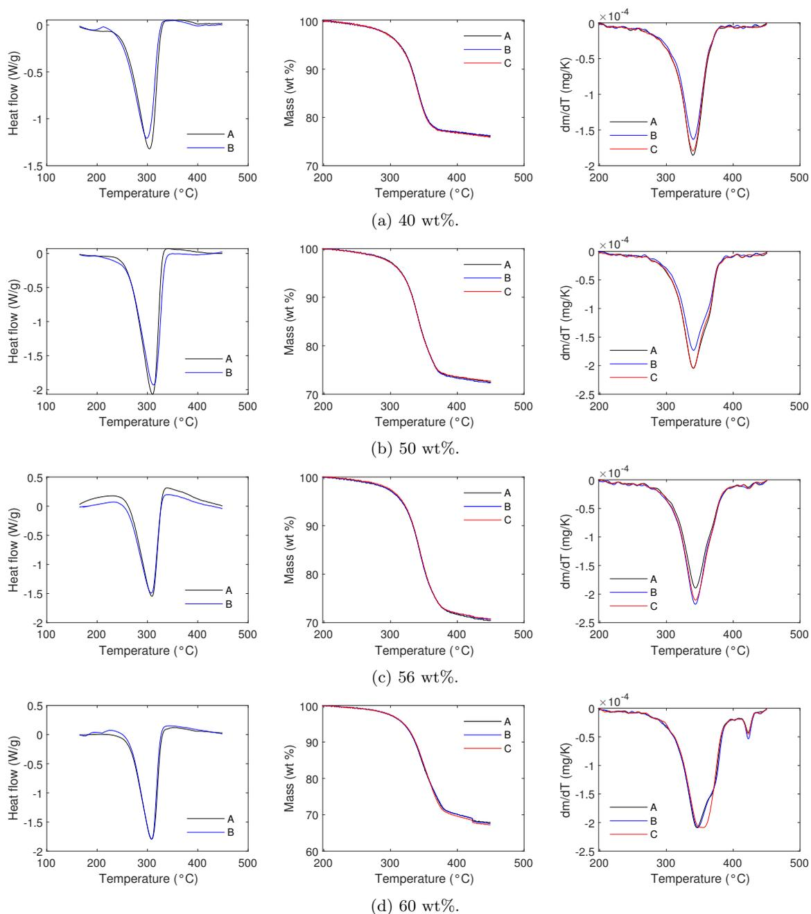
Figure H.5: DSC (left), TGA (middle) and DTG (right) results of carbon BPL filled with  $\text{NaClO}_4$  from solution at different concentrations (40, 50, 56 and 60 wt%).
