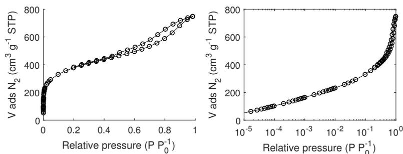
Figure C.6: N<sub>2</sub> adsorption/desorption isotherm of carbon C-R300 measured at 77 K.
