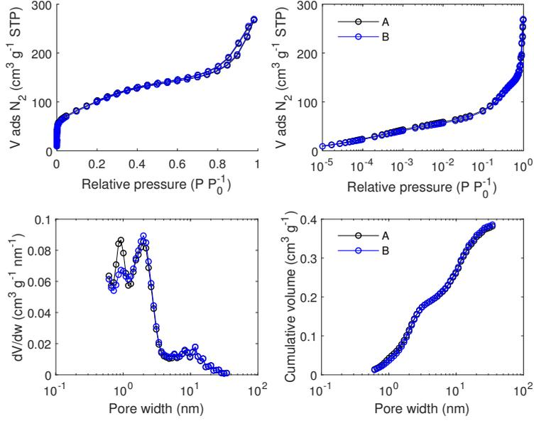
Figure F.10:  $N_2$  adsorption/desorption isotherm data measured at 77 K and pore size analysis by equilibrium QSDFT for carbon F5001 filled with  $NaClO_4$  from a 60 wt% aqueous solution. A and B are repetitions (from the synthesis).
