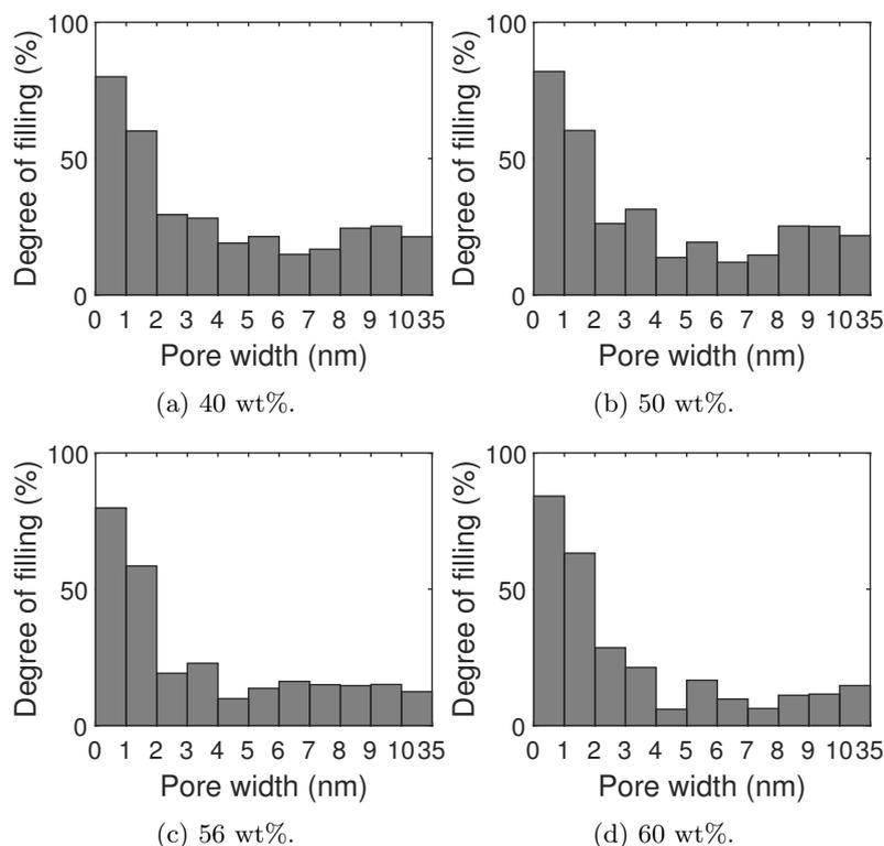
Figure 3.33: Influence of the solution concentration on the degree of pore filling for carbon BPL filled with NaClO<sub>4</sub>.
