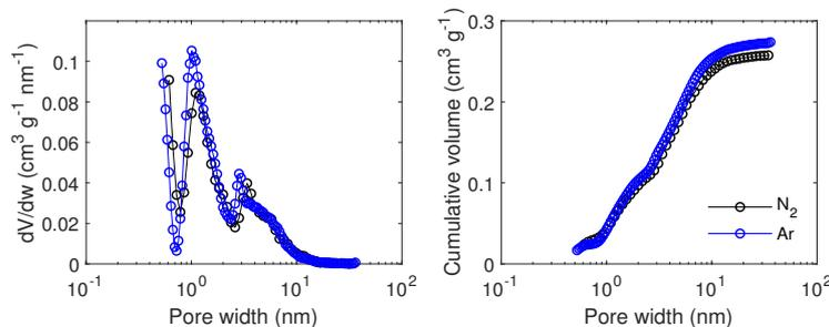
Figure D.12: Pore size distribution modelled by QSDFT based on N<sub>2</sub> at 77 K and Ar at 87 K adsorption/desorption isotherms for carbon C-R600 filled with NaClO<sub>4</sub> from a 56 wt% aqueous solution.
