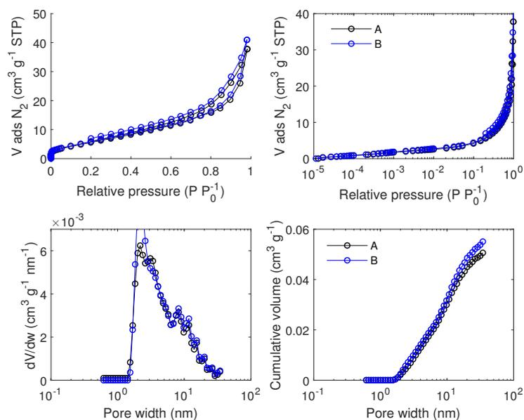
Figure F.11:  $N_2$  adsorption/desorption isotherm data measured at 77 K and pore size analysis by equilibrium QSDFT for carbon F5001-APS filled with  $NaClO_4$  from a 56 wt% aqueous solution. A and B are repetitions (from the synthesis).
