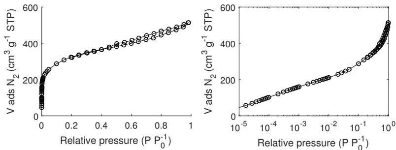
Figure C.31: N<sub>2</sub> adsorption/desorption isotherm of carbon BPL-37 measured at 77 K.
