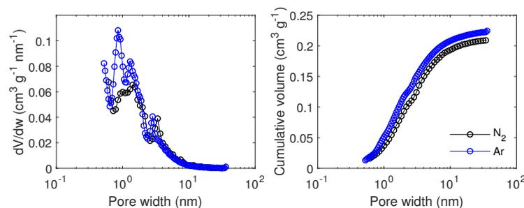
Figure D.33: Pore size distribution modelled by QSDFT based on  $\text{N}_2$  at 77 K and  $\text{Ar}$  at 87 K adsorption/desorption isotherms for carbon BPL-37 filled with  $\text{NaClO}_4$  from a 56 wt% aqueous solution.
