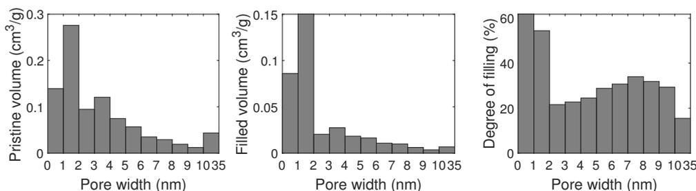
Figure 3.21: Degree of pore filling with respect to the pristine carbon for carbon C filled with KNO<sub>3</sub>.
