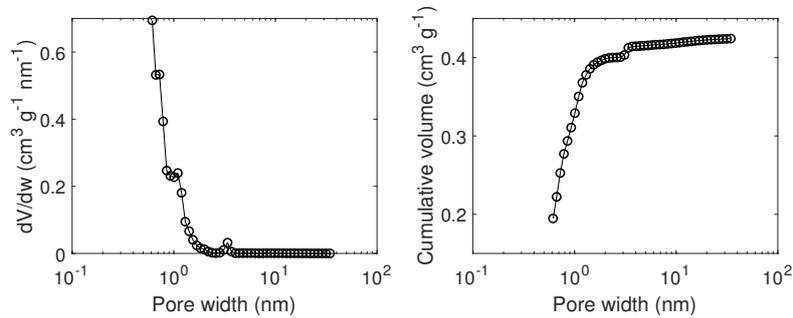
Figure C.40: Pore size distribution modelled by QSDFT based on N<sub>2</sub> adsorption/desorption isotherm for carbon FY5-21.
