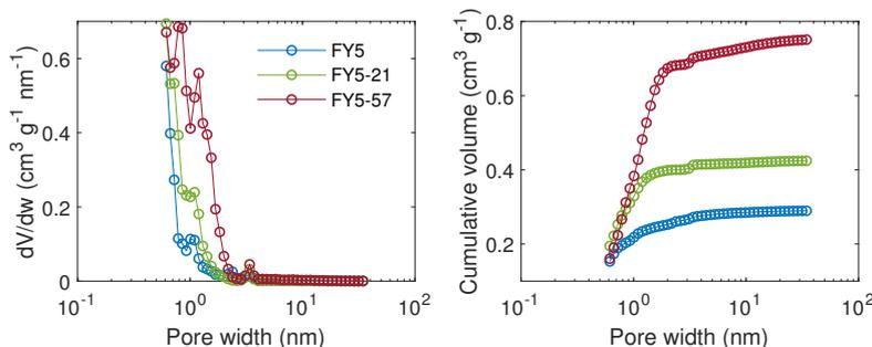
Figure 3.11: Pore size distribution modelled by QSDFT based on N<sub>2</sub> isotherm of carbon FY5 and its overactivated derivatives.
