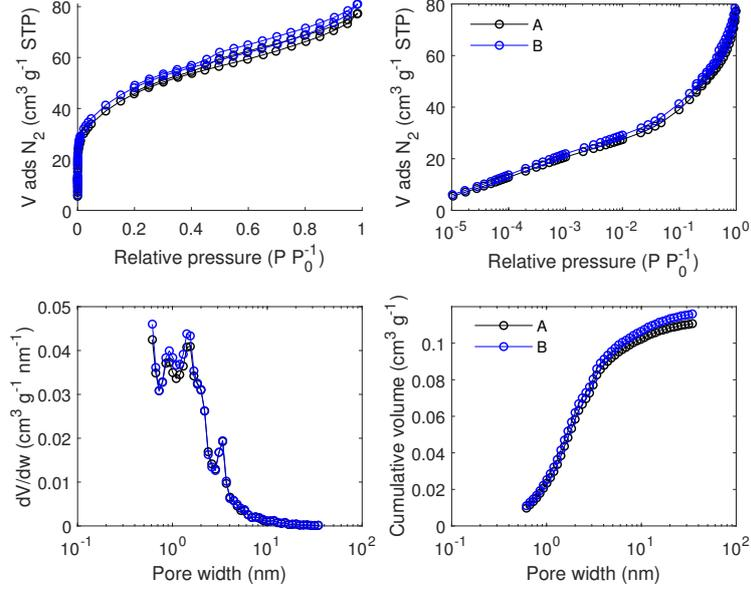
Figure F.14: N<sub>2</sub> adsorption/desorption isotherm data measured at 77 K and pore size analysis by equilibrium QSDFT for carbon BPL filled with NaClO<sub>4</sub> from a 50 wt% aqueous solution. A and B are repetitions (from the synthesis).
