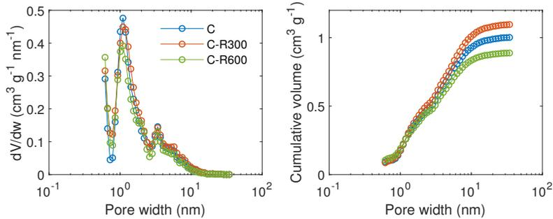
Figure 3.2: Pore size distribution modelled by QSDFT based on  $N_2$  isotherm of carbon C and its derivatives obtained by thermal treatment.
