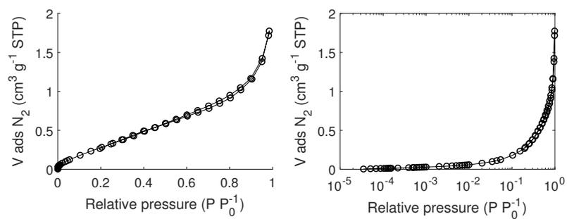
Figure E.3: N<sub>2</sub> adsorption/desorption isotherm of ammonium perchlorate measured at 77 K.
