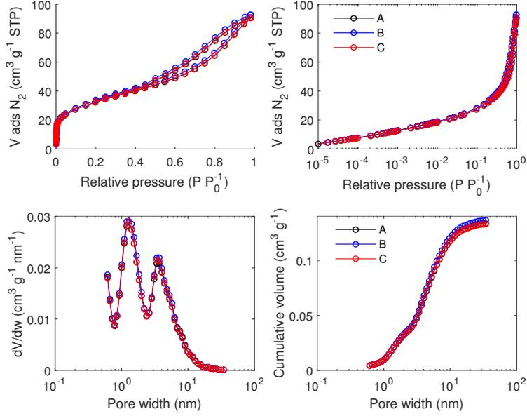
Figure F.3:  $N_2$  adsorption/desorption isotherm data measured at 77 K and pore size analysis by equilibrium QSDFT for carbon C filled with  $NaClO_4$  from a 56 wt% aqueous solution. A, B and C are repetitions (from the synthesis).
