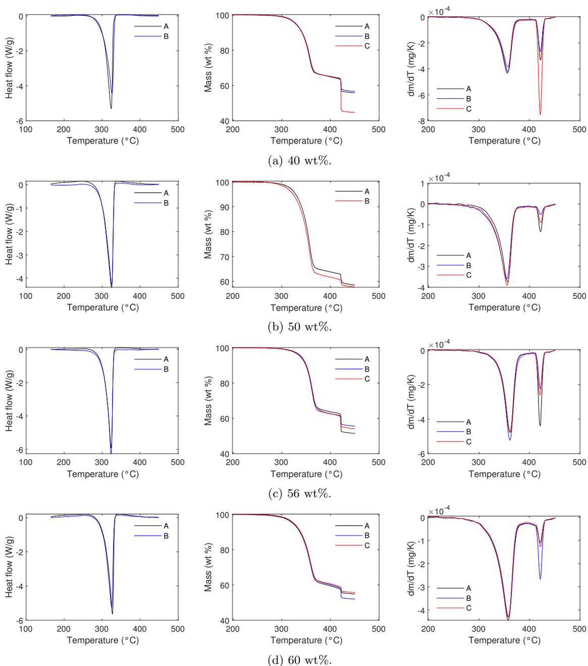
Figure H.3: DSC (left), TGA (middle) and DTG (right) results of carbon F5001 filled with NaClO<sub>4</sub> from solution at different concentrations (40, 50, 56 and 60 wt%).
