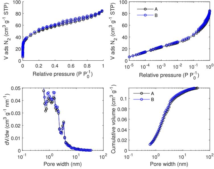
Figure F.15:  $N_2$  adsorption/desorption isotherm data measured at 77 K and pore size analysis by equilibrium QSDFT for carbon BPL filled with  $NaClO_4$  from a 56 wt% aqueous solution. A and B are repetitions (from the synthesis).
