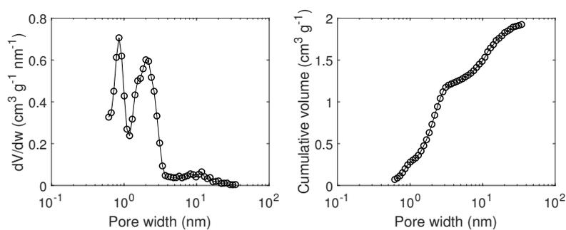
Figure C.21: Pore size distribution modelled by QSDFT based on N<sub>2</sub> adsorption/desorption isotherm for carbon F5001-HN.
