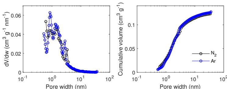
Figure D.27: Pore size distribution modelled by QSDFT based on  $\text{N}_2$  at 77 K and  $\text{Ar}$  at 87 K adsorption/desorption isotherms for carbon BPL filled with  $\text{NaClO}_4$  from a 40 wt% aqueous solution.
