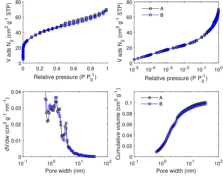
Figure F.16: N<sub>2</sub> adsorption/desorption isotherm data measured at 77 K and pore size analysis by equilibrium QSDFT for carbon BPL filled with NaClO<sub>4</sub> from a 60 wt% aqueous solution. A and B are repetitions (from the synthesis).
