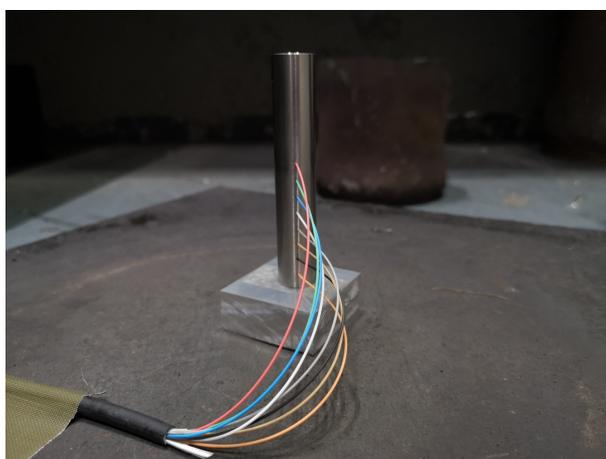
Figure 2.4: Example of the experimental set-up used to measure the velocity of detonation of a charge confined in a steel tube.
