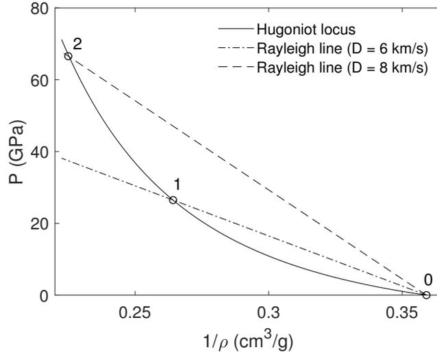
Figure 1.1: Determination of the properties of the shocked state of aluminum. The initial state (0) is characterized by a specific mass of  $2.8 \text{ g/cm}^3$ . Two shocked states, 1 and 2, are represented as illustrations. Numerical data from the literature [8] were used in equations (1.7) and (1.8).
