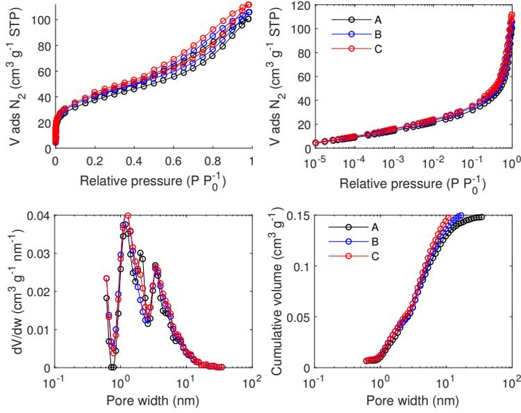
Figure F.1:  $N_2$  adsorption/desorption isotherm data measured at 77 K and pore size analysis by equilibrium QSDFT for carbon C filled with  $NaClO_4$  from a 40 wt% aqueous solution. A, B and C are repetitions (from the synthesis).
