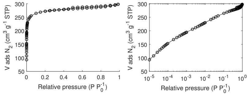
Figure C.39: N<sub>2</sub> adsorption/desorption isotherm of carbon FY5-21 measured at 77 K.
