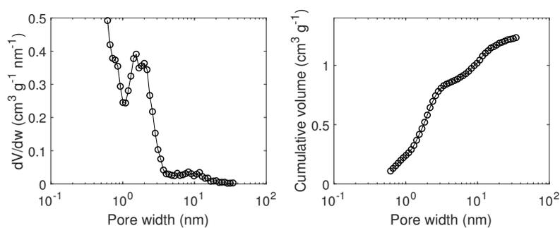
Figure C.18: Pore size distribution modelled by QSDFT based on N<sub>2</sub> adsorption/desorption isotherm for carbon F5001-APS.
