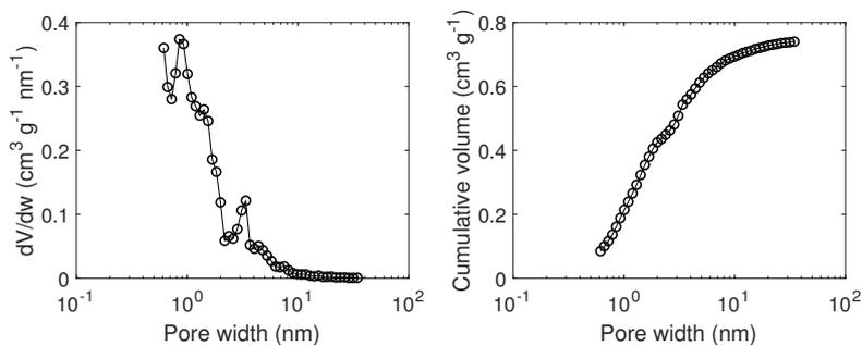
Figure C.32: Pore size distribution modelled by QSDFT based on N<sub>2</sub> adsorption/desorption isotherm for carbon BPL-37.
