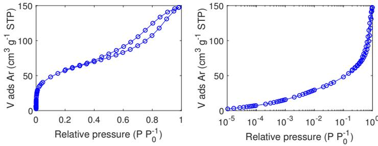
Figure D.8: Ar adsorption/desorption isotherm of carbon C-R300 filled with NaClO<sub>4</sub> from a 56 wt% aqueous solution measured at 87 K.
