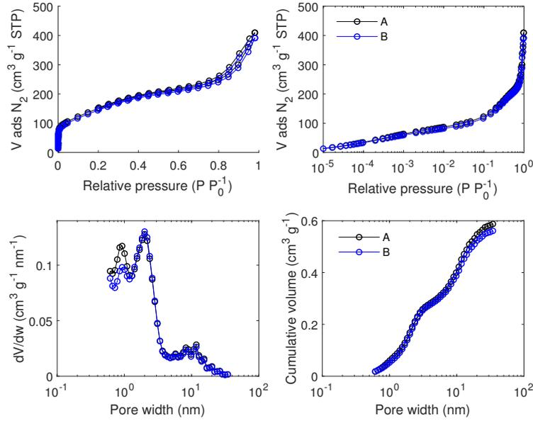
Figure F.7: N<sub>2</sub> adsorption/desorption isotherm data measured at 77 K and pore size analysis by equilibrium QSDFT for carbon F5001 filled with NaClO<sub>4</sub> from a 40 wt% aqueous solution. A and B are repetitions (from the synthesis).
