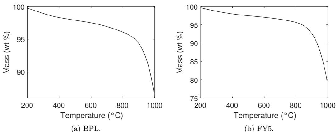
Figure A.1: CO<sub>2</sub> reactivity curves measured by TGA.
