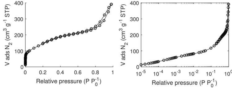
Figure D.13: N<sub>2</sub> adsorption/desorption isotherm of carbon F5001 filled with NaClO<sub>4</sub> from a 40 wt% aqueous solution measured at 77 K.
