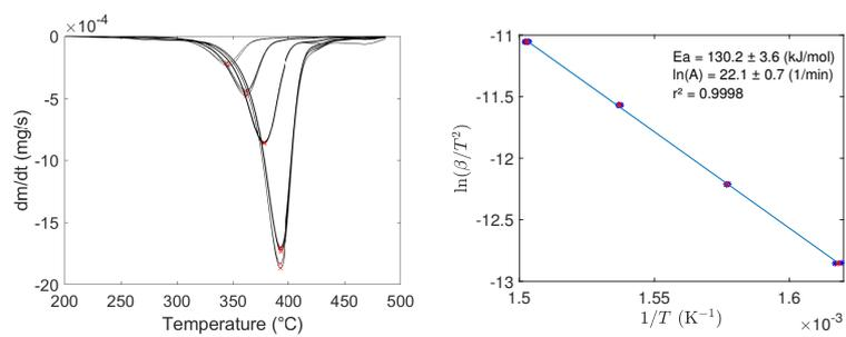
Figure H.13: TGA results (at 1, 2, 4 and 7 K/min) of a physical mixture of carbon F5001 and sodium perchlorate at 2.15 g/g, both milled and sieved between 25 and 50  $\mu\text{m}$ , and decomposition kinetics modelling.
