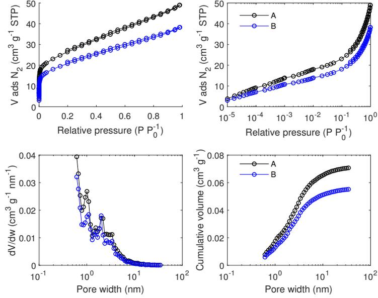
Figure F.22:  $N_2$  adsorption/desorption isotherm data measured at 77 K and pore size analysis by equilibrium QSDFT for carbon FY5 filled with  $NaClO_4$  from a 60 wt% aqueous solution. A and B are repetitions (from the synthesis).
