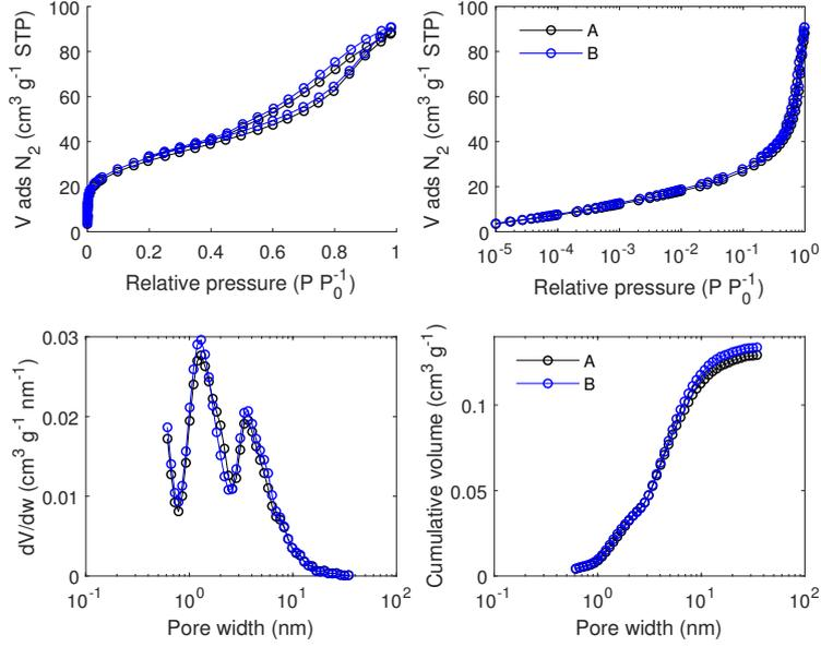
Figure F.4:  $N_2$  adsorption/desorption isotherm data measured at 77 K and pore size analysis by equilibrium QSDFT for carbon C filled with  $NaClO_4$  from a 60 wt% aqueous solution. A and B are repetitions (from the synthesis).
