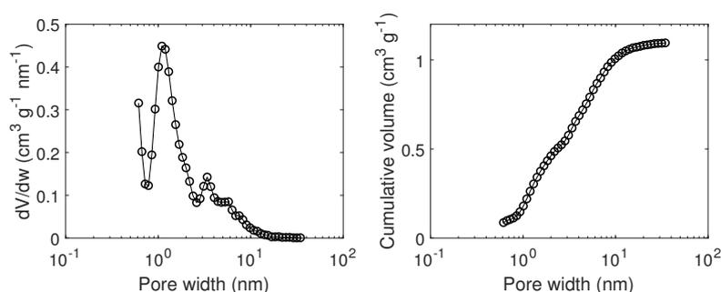
Figure C.7: Pore size distribution modelled by QSDFT based on N<sub>2</sub> adsorption/desorption isotherm for carbon C-R300.
