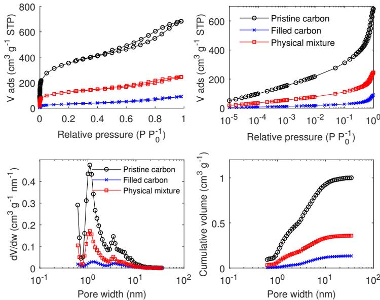
Figure 3.16: Comparison between  $\text{N}_2$  adsorption isotherm and pore size analysis of the pristine carbon, the filled carbon and the corresponding theoretical physical mixture for carbon C filled with  $\text{NaClO}_4$ .
