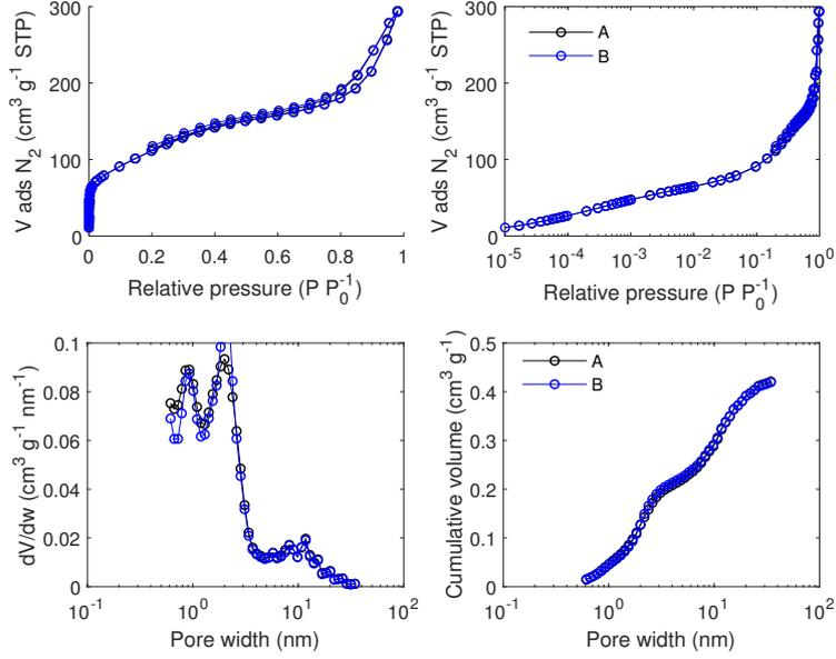
Figure F.9:  $N_2$  adsorption/desorption isotherm data measured at 77 K and pore size analysis by equilibrium QSDFT for carbon F5001 filled with  $NaClO_4$  from a 56 wt% aqueous solution. A and B are repetitions (from the synthesis).
