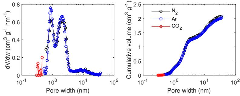
Figure C.15: Pore size distribution modelled by QSDFT for N<sub>2</sub> and Ar adsorption/desorption isotherms and NLDFT for CO<sub>2</sub> adsorption/desorption isotherm for carbon F5001.
