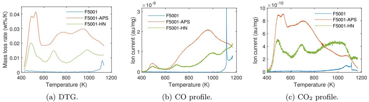
Figure 3.6: TPDMS analysis of carbon F5001 and its derivatives obtained by chemical oxidation.
