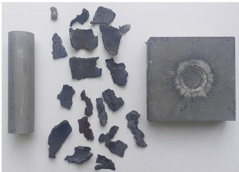
Figure I.2: Fragmentation pattern obtained after the initiation of a physical mixture of carbon C and sodium perchlorate at a density of  $0.73 \text{ g/cm}^3$  and heavily confined in a 30 mm steel tube (a pristine tube is shown on the left side of the picture). The recovered witness plate is also shown on the right side of the picture.
