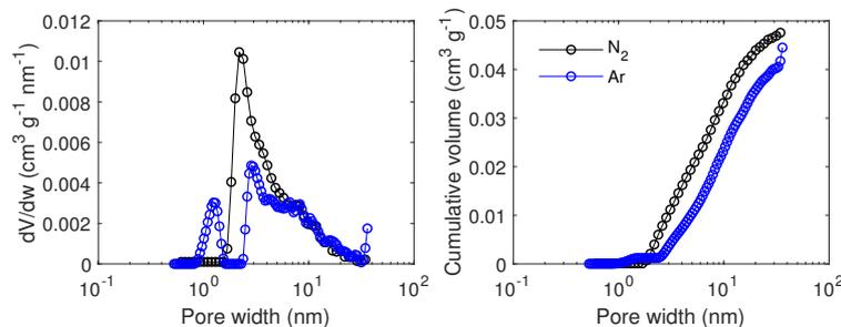
Figure D.21: Pore size distribution modelled by QSDFT based on  $\text{N}_2$  at 77 K and  $\text{Ar}$  at 87 K adsorption/desorption isotherms for carbon F5001-APS filled with  $\text{NaClO}_4$  from a 56 wt% aqueous solution.
