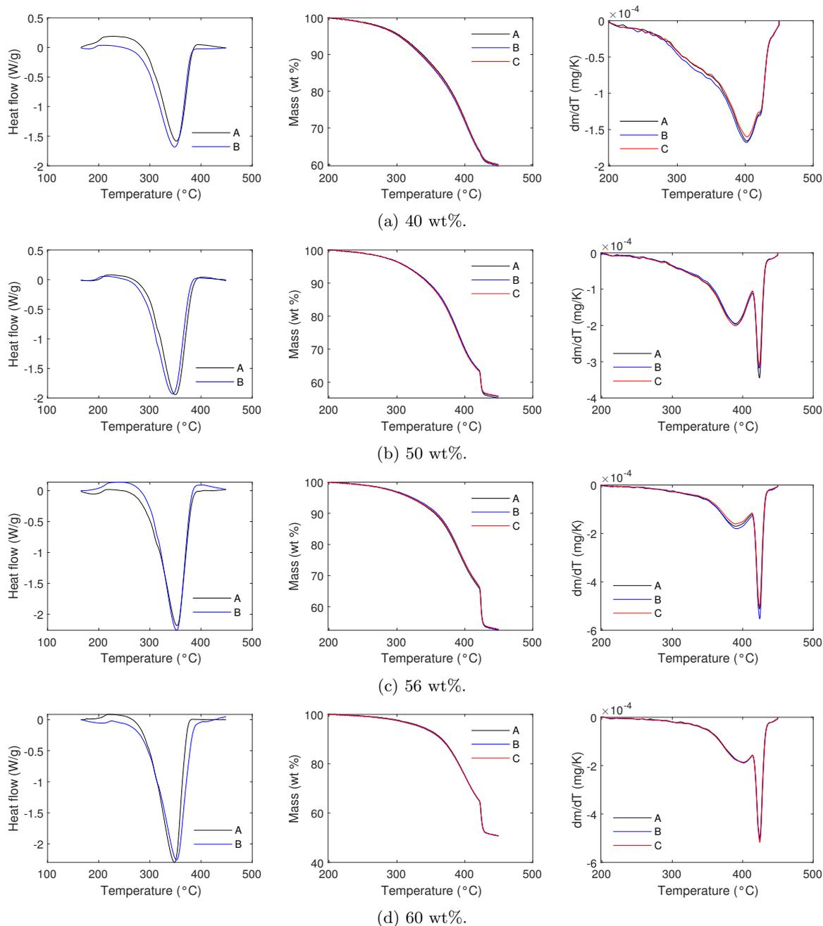
Figure H.1: DSC (left), TGA (middle) and DTG (right) results of carbon C filled with NaClO<sub>4</sub> from solution at different concentrations (40, 50, 56 and 60 wt%).
