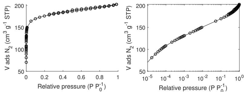
Figure C.34:  $N_2$  adsorption/desorption isotherm of carbon FY5 measured at 77 K.
