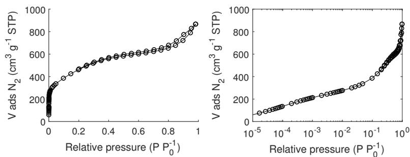
Figure C.17: N<sub>2</sub> adsorption/desorption isotherm of carbon F5001-APS measured at 77 K.
