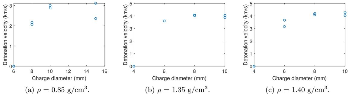
Figure 4.11: Measured detonation velocities in function of the charge diameter for carbon C filled with  $\text{NaClO}_4$  from a 56 wt% aqueous solution compressed at different densities ( $\rho$ ), in a heavy confinement and initiated by a standard detonator.
