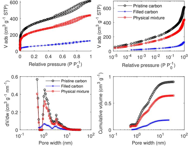
Figure 3.24: Comparison between  $N_2$  adsorption isotherm and pore size analysis of the pristine carbon, the filled carbon and the corresponding theoretical physical mixture for carbon C filled with  $NH_4ClO_4$ .
