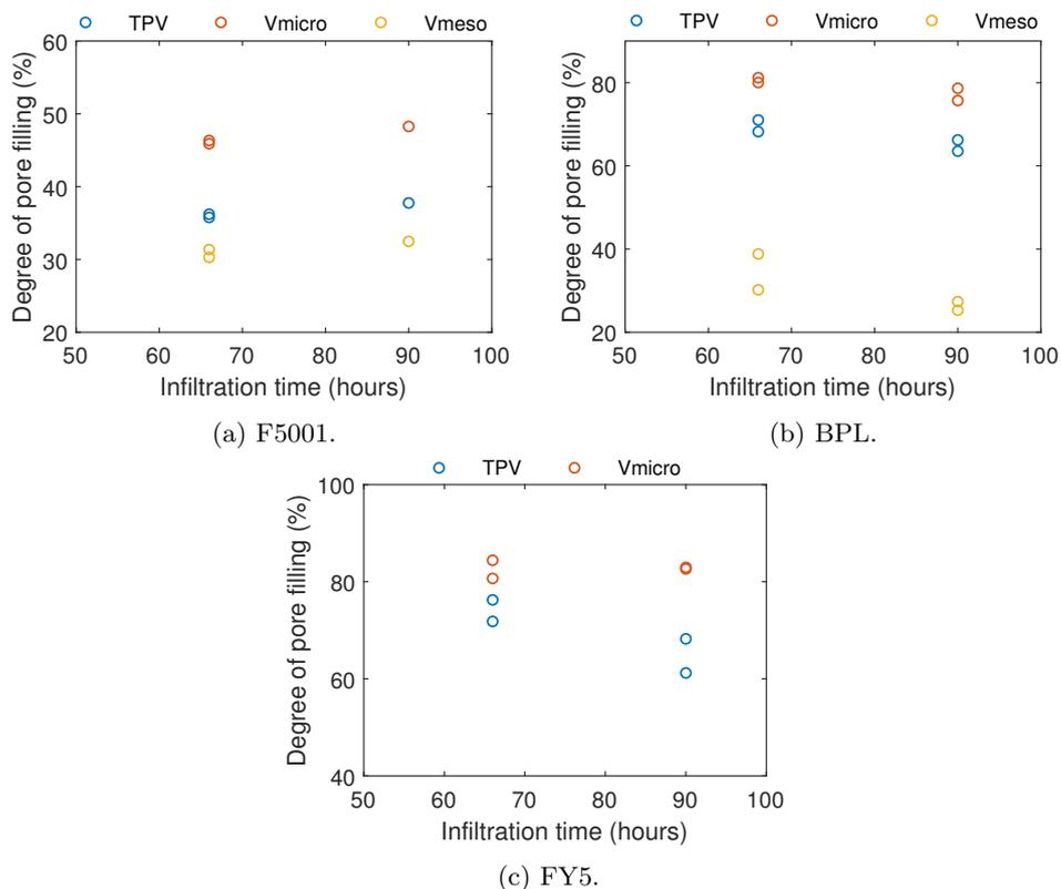
Figure 3.29: Carbons F5001, BPL and FY5 filled with  $\text{NaClO}_4$ . Influence of the infiltration time on the degree of pore filling.
