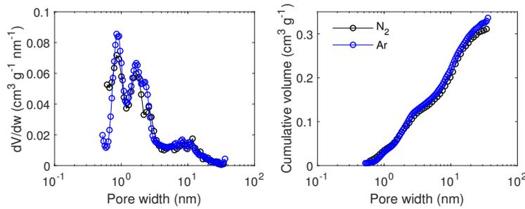
Figure D.24: Pore size distribution modelled by QSDFT based on  $\text{N}_2$  at 77 K and  $\text{Ar}$  at 87 K adsorption/desorption isotherms for carbon F5001-HN filled with  $\text{NaClO}_4$  from a 56 wt% aqueous solution.
