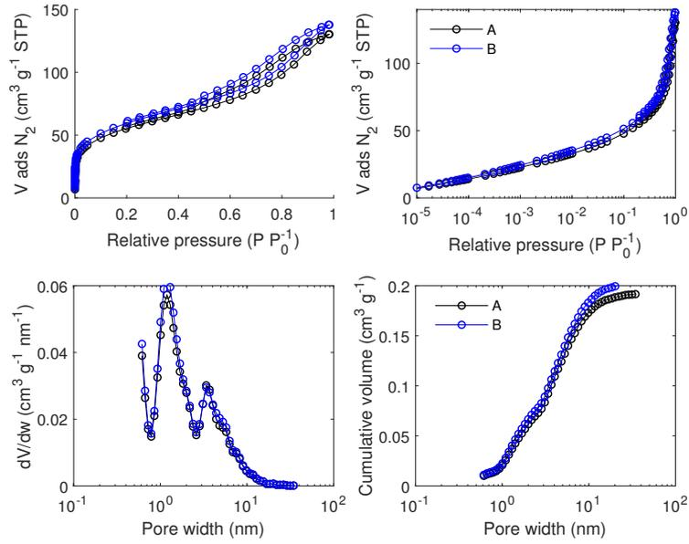
Figure F.5:  $\text{N}_2$  adsorption/desorption isotherm data measured at 77 K and pore size analysis by equilibrium QSDFT for carbon C-R300 filled with  $\text{NaClO}_4$  from a 56 wt% aqueous solution. A and B are repetitions (from the synthesis).
