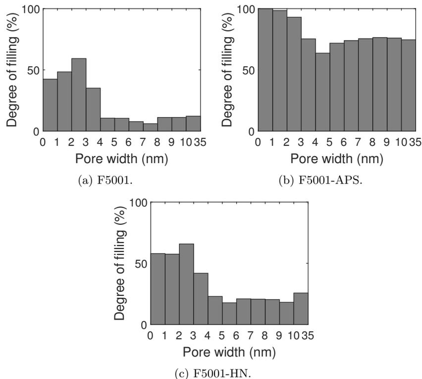
Figure 3.36: Degree of pore filling of carbon F5001 and its derivatives filled with NaClO<sub>4</sub>.
