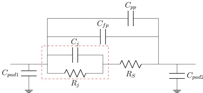
**Figure 3.14:** Schottky diode equivalent circuit. Highlighted in red, the basic Schottky diode model
