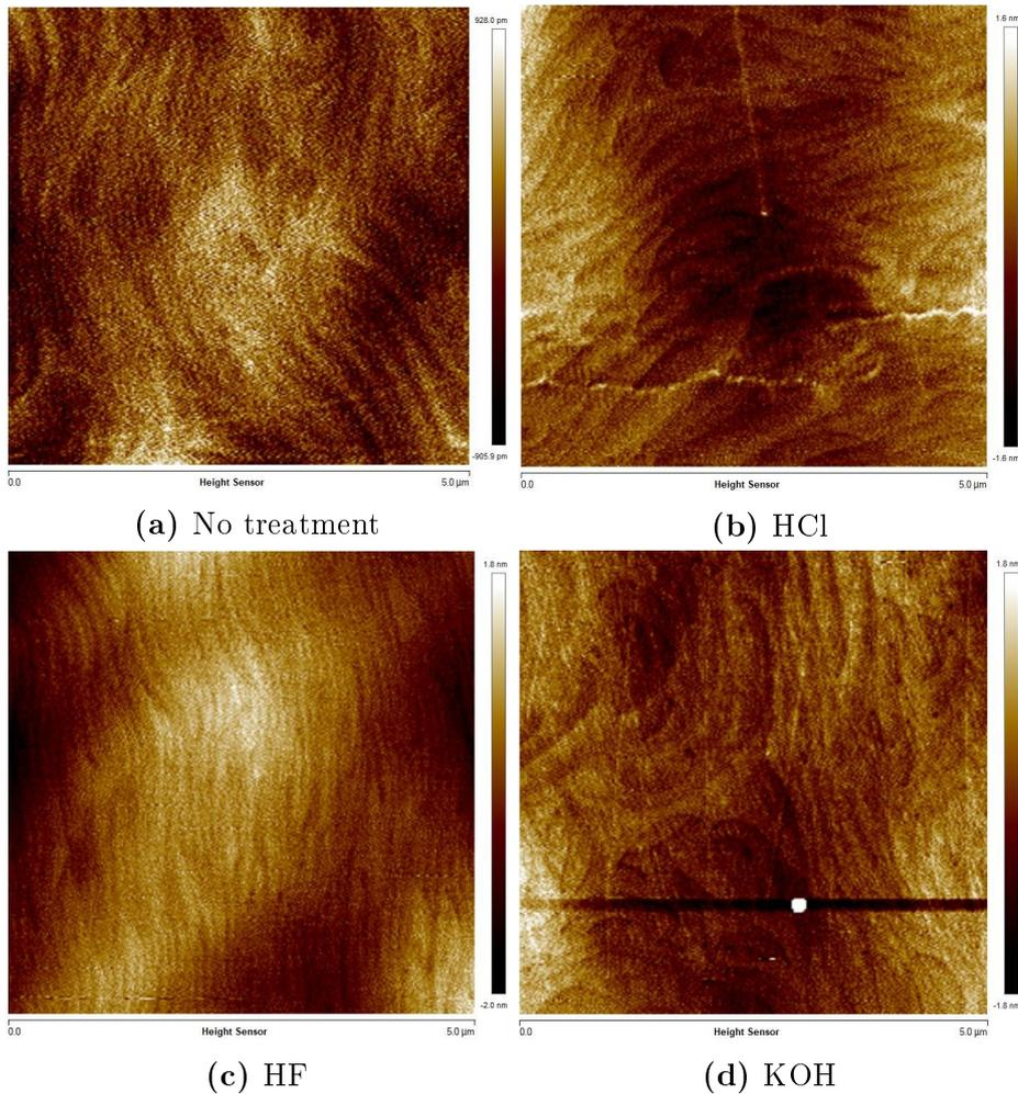
**Figure 2.21:** AFM images from randomly selected  $5\ \mu\text{m} \times 5\ \mu\text{m}$  areas of GaN on SiC samples for each of the surface treatments performed
