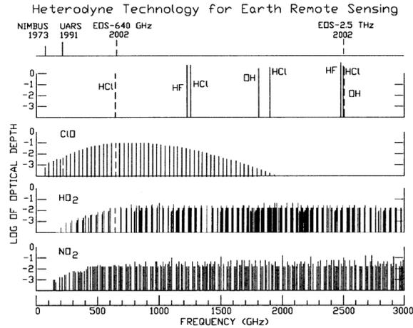
**Figure 1.3:** Spectra of some important molecules in the Earth’s upper atmosphere and measurements being addressed by NASA heterodyne instruments. The peak power or minimum frequency for many emission lines occurs in the terahertz region [3]
