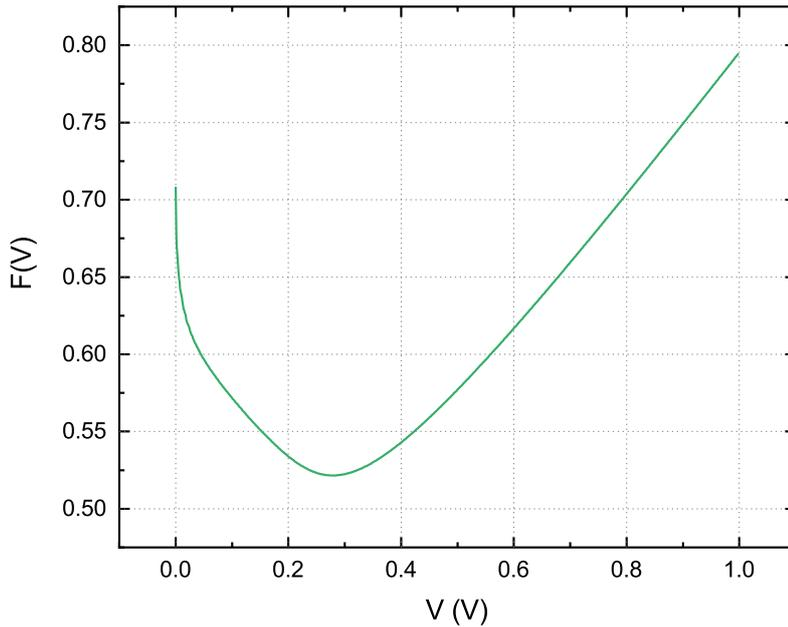
**Figure 3.7:** Norde's auxiliary function extracted for the 70  $\mu\text{m}$  diode. In this case, the minimum is found at  $V_0 = 0.278$  V. Therefore, the extracted parameters are  $\phi_B = 0.635$  eV and  $R_S \approx 807.72$   $\Omega$
