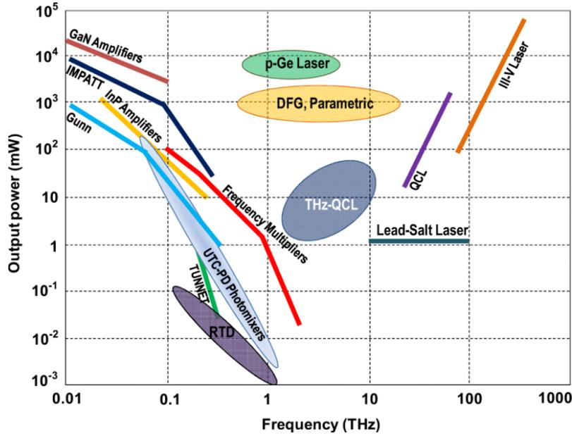
Figure 1.6: THz sources as a function of frequency [28]
