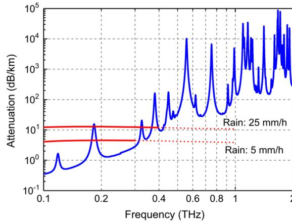
**Figure 1.4:** Atmospheric attenuation computed at sea-level altitude, water content of  $7.5 \text{ g/m}^3$ , and atmospheric temperature of  $20^\circ\text{C}$  [11].
