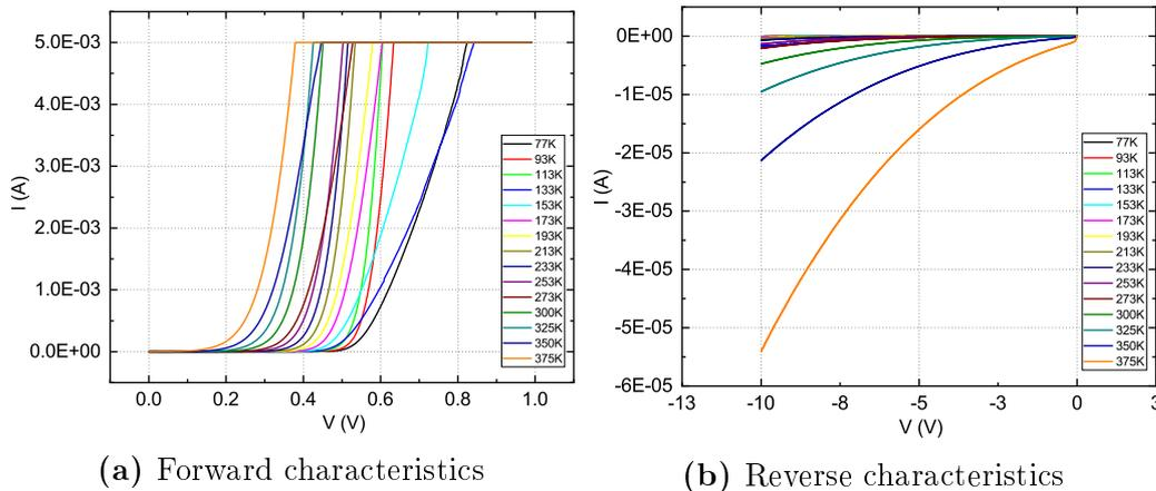
**Figure 3.10:** Experimental DC characteristics for the 70  $\mu\text{m}$  diode taken at temperatures ranging between 77–375 K. A current compliance of 5 mA was used during the measurements in order to avoid premature breakdown
