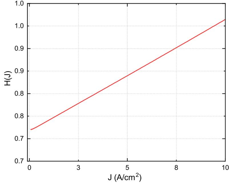
**Figure 3.9:** Plot of  $H(J)$  versus  $J$  for the 70  $\mu\text{m}$  diode using the ideality factor extracted previously. From the linear fit,  $\phi_B = 0.593 \text{ eV}$  and  $R_S^2 = 658.45 \Omega$ , in good agreement with the value of  $R_S^1$
