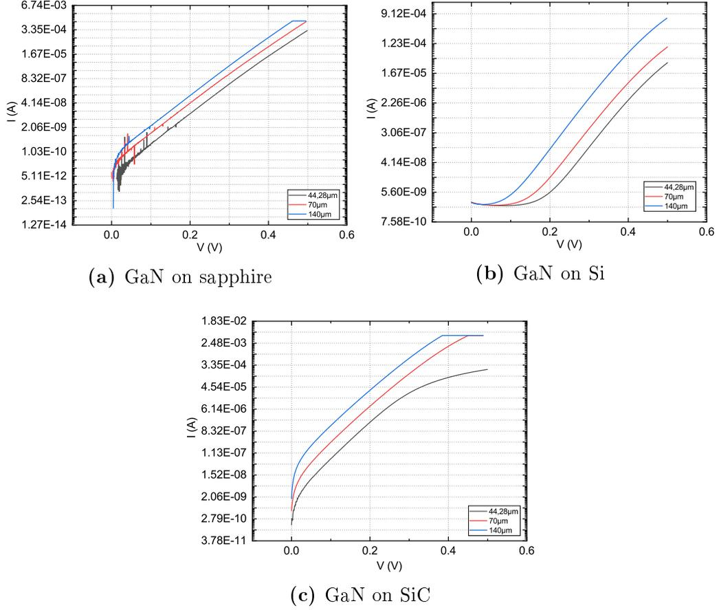
**Figure 3.17:** Typical DC characteristics for the three diode measured (140  $\mu\text{m}$ , 70  $\mu\text{m}$ , 44.28  $\mu\text{m}$  in diameter) on each substrate. The characteristics were measured between 0 V and 0.5 V with a current compliance of 1 mA
