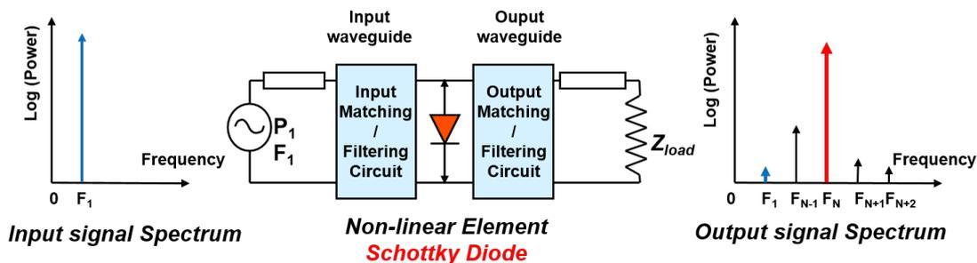
Figure 1.8: A schematic view of a frequency multiplier
