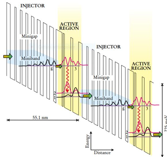
**Figure 1.7:** Band diagram of a QCL stage, from [37]
