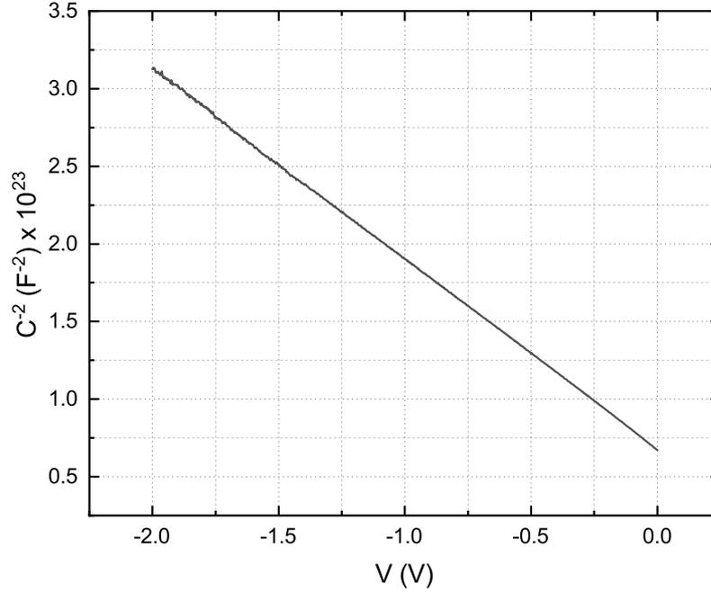
**Figure 3.13:** Plot of  $C^{-2}$  vs  $V$  for the 70  $\mu\text{m}$  diode for barrier height extraction. The resulting flat-band barrier height is equal to 0.675 eV, and  $N_d = 8.83 \cdot 10^{16} \text{ cm}^{-3}$
