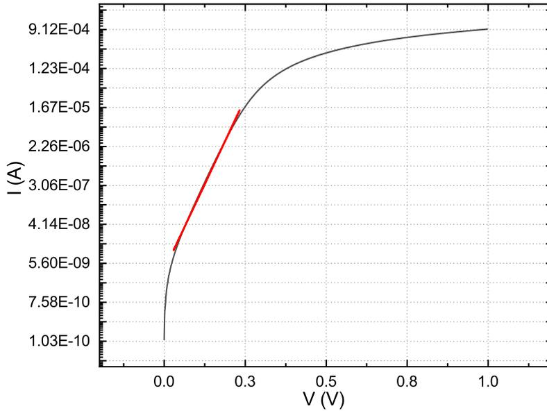
**Figure 3.5:** Forward characteristics of a 70  $\mu\text{m}$  diode (GaN on SiC) with its linear fit (in red). The barrier height and ideality factor extracted with this fit are, respectively, 0.615 eV and 1.098
