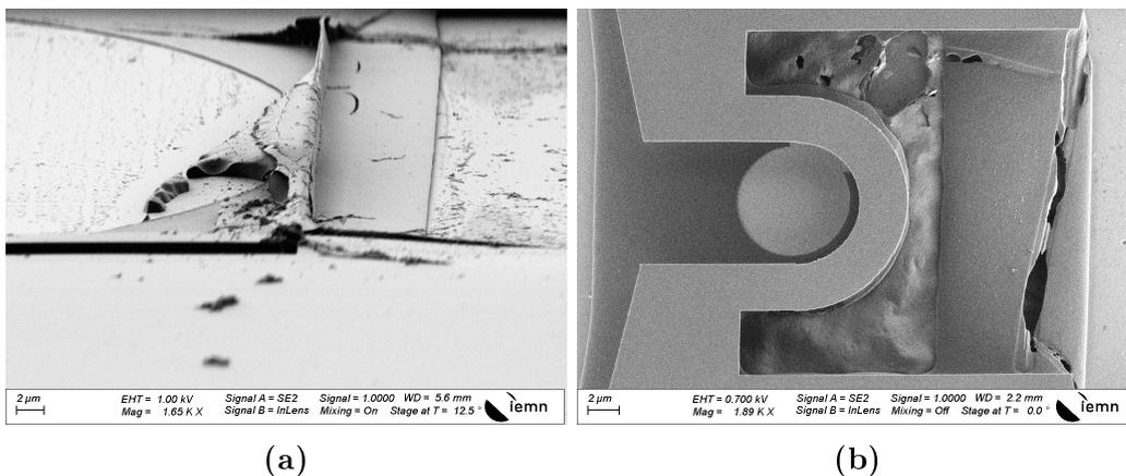
**Figure 2.17:** Over-development of the reflow resist on GaN on Si process. In the profile view shown in (a), the reflow resist got completely develop by the secondary exposure, while in the top view shown in (b) the reflow resist presented severe cracks after the develop of the last lithographic step
