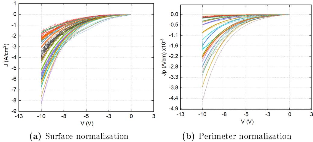
**Figure 3.21:** Normalization of the current with respect to surface and perimeter in order to investigate the nature of leakage current. In this case, 23 GaN on Si Schottky diodes with diameters between 2–40  $\mu\text{m}$  were analyzed
