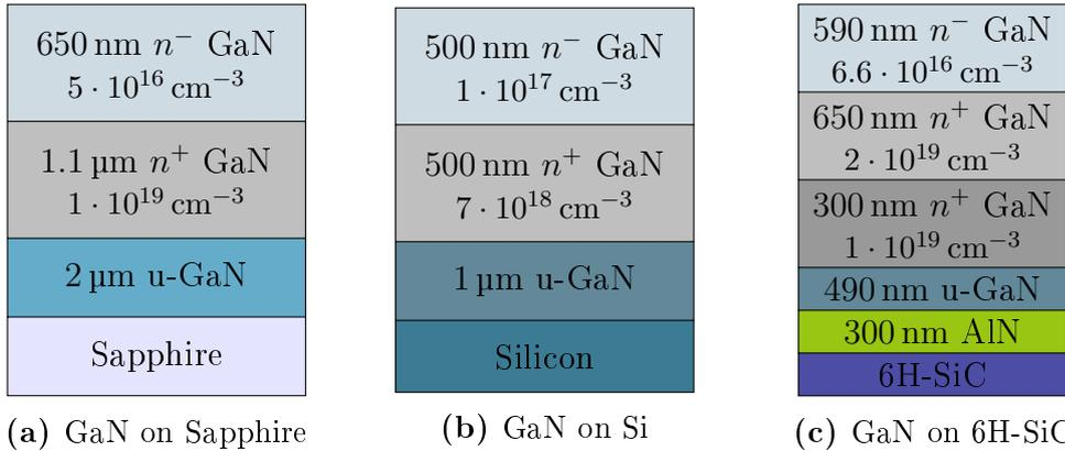
**Figure 2.1:** Schematic cross-view of the three epitaxies used
