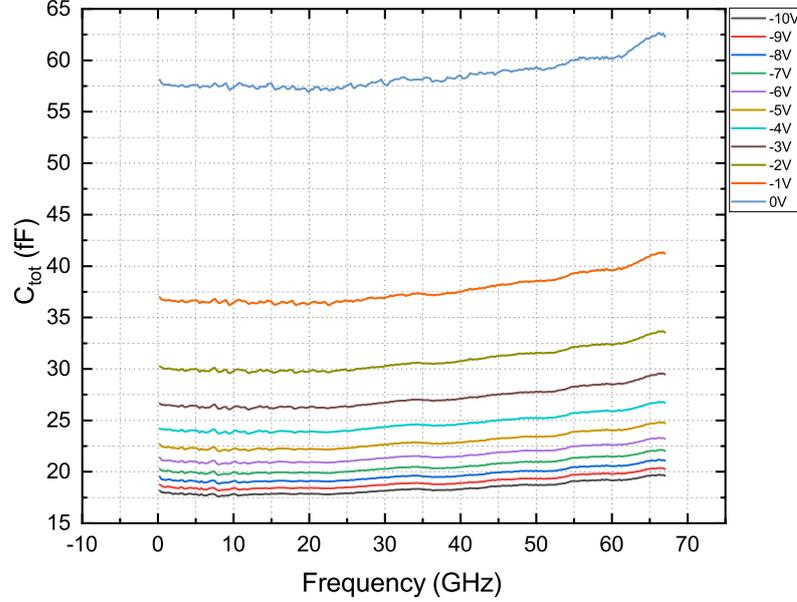
**Figure 3.15:** Capacitance measurements obtained from S-parameters for an 8  $\mu\text{m}$  diode (GaN on SiC)
