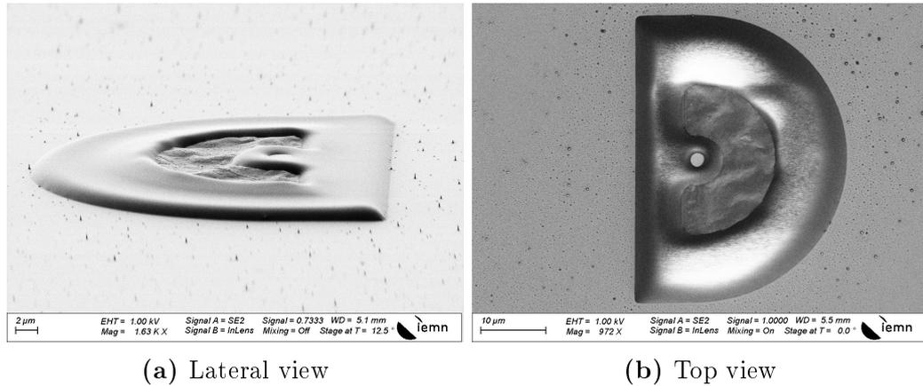
**Figure 2.13:** Resist reflow
