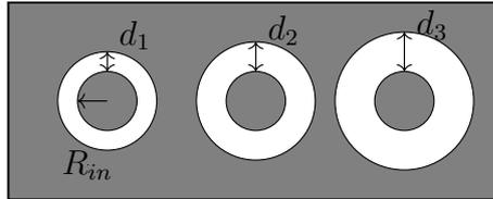
**Figure 2.8:** Circular TLM pattern structure
