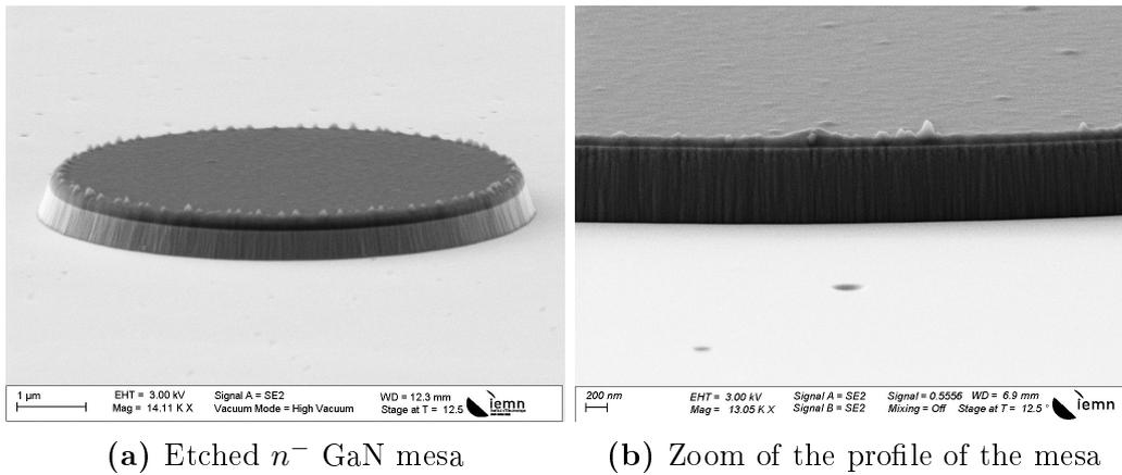
**Figure 2.5:**  $n^-$  GaN mesa after dry etching
