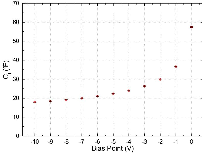
**Figure 3.16:** Experimentally obtained values of the junction capacitance for the  $8\mu\text{m}$  diode. By fitting to Eq. 3.55,  $C_{j0} = 5.11 \cdot 10^{-14}\text{ F}$ ,  $C_{par} = 6.3 \cdot 10^{-15}\text{ F}$ , and  $V_{bi} = 0.54\text{ eV}$
