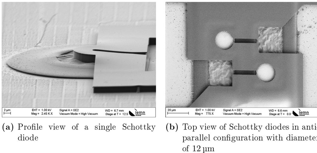
**Figure 2.14:** SEM images of Schottky diodes after the development of the final lithographic step, just before air-bridge metallization
