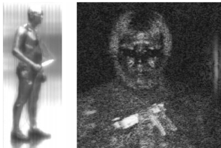
Figure 1.5: Active and passive images: on the left, 94-GHz passive image: metal knife inside newspaper; on the right, 640 GHz active image: toy gun under cotton shirt [21]
