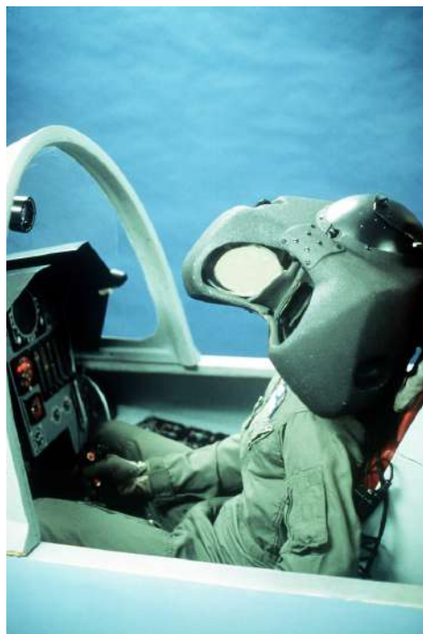
FIGURE 1.3 – Visually Coupled Airborne Systems Simulator (VCASS) . Developed by Tom Furness in 1982.
