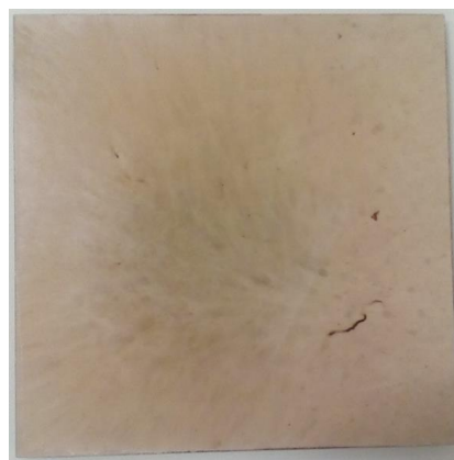
Figure 118. Single 25 \times 25 \times 0.42 \text{ cm} PEKK layer after the molding process.
