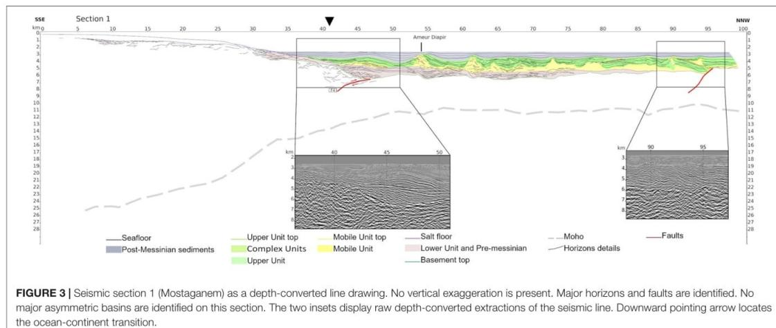
**FIGURE 3 |** Seismic section 1 (Mostaganem) as a depth-converted line drawing. No vertical exaggeration is present. Major horizons and faults are identified. No major asymmetric basins are identified on this section. The two insets display raw depth-converted extractions of the seismic line. Downward pointing arrow locates the ocean-continent transition.
