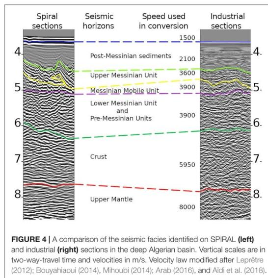
**FIGURE 4 |** A comparison of the seismic facies identified on SPIRAL (left) and industrial (right) sections in the deep Algerian basin. Vertical scales are in two-way-travel time and velocities in m/s. Velocity law modified after Leprêtre (2012); Bouyahiaoui (2014), Mihoubi (2014); Arab (2016), and Aïdi et al. (2018).
