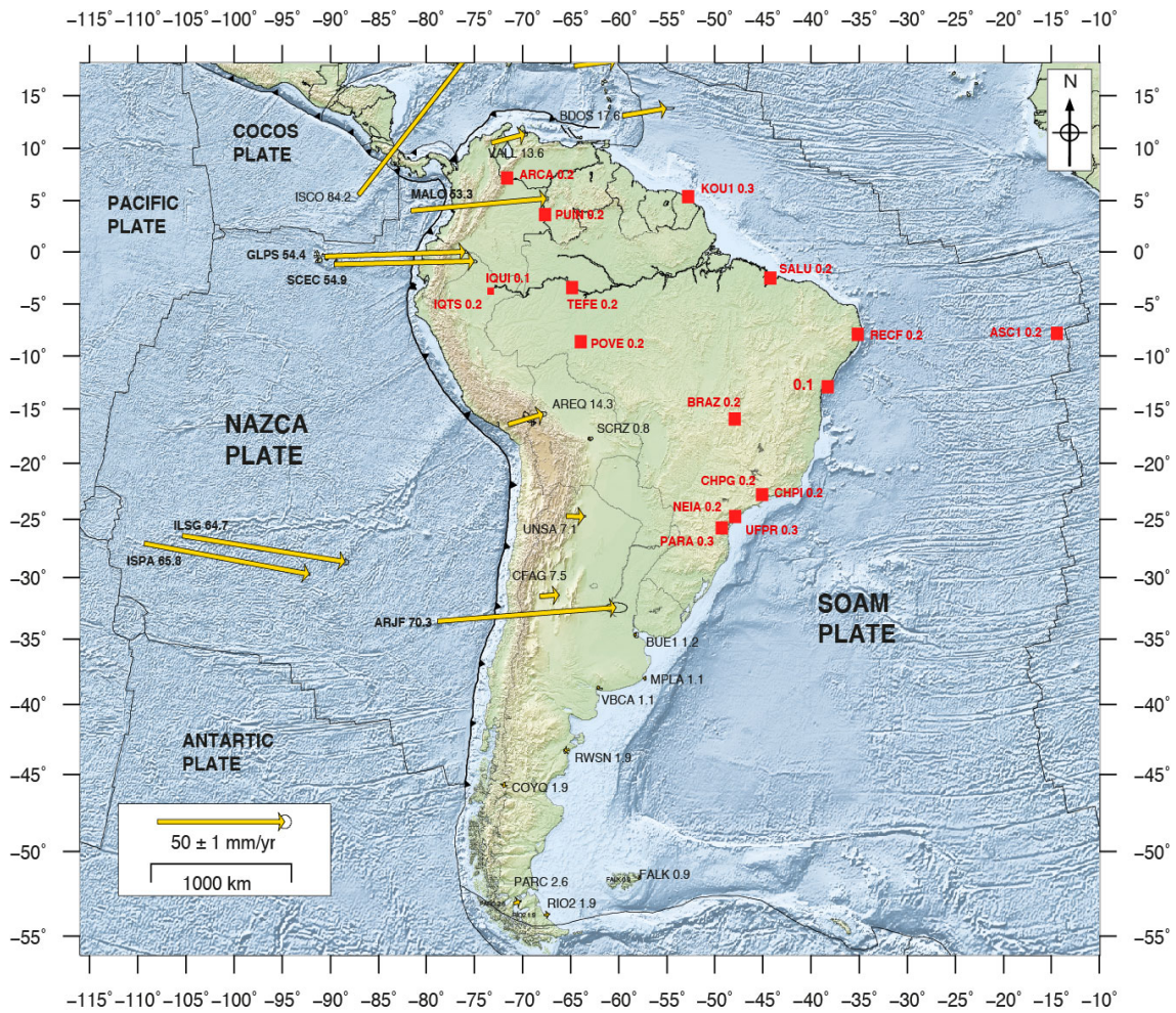
Figure 2.17 – Large scale of GPS stations used to define the stable South America (SOAM) reference frame. 17 sites (labelled in red with its corresponding horizontal velocities values) was used to compute the rotation vector, which is located at 18.41°S, 133.28°W, 0.121 °/Myr. Ellipses show 95% of confidence (see table 2.1). Yellow arrows are sites velocities in Nazca, Cocos and Caribbean plates relative to SOAM.
