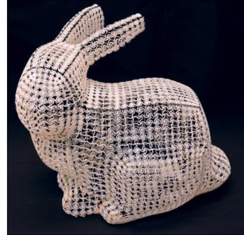
In some cases, it is possible to control how the material will deform by carefully picking the right tileable elements that compose the metamaterial, and thus to create *programmable materials* which have their deformation behavior encoded within their structure, the process of designing such materials is called *inverse design*.
