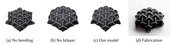
Fig. 3.5: Impact of critical components of our model when simulating a uniform field of stars. (a) Neglecting bending forces in the fabric makes the stars contract independently of each other, preventing the emergence of global curvature. (b) Using a flat rest shape for the rods makes the stars less curved than in reality. (c, d) Our complete model better reproduces the fabricated surface.
