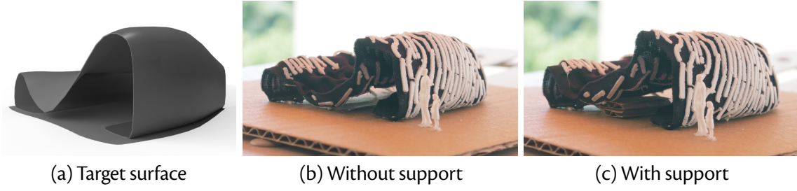
Fig. 5.13: Limitation. Without additional support, this architectural model sags under its own weight (b). Adding a cardboard support underneath the structure brings it closer to the target surface (c).
