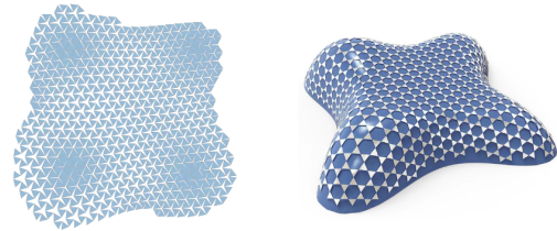
Fig. 2.5: left: flattened auxetic pattern, right: projected pattern onto the target surface [68].
