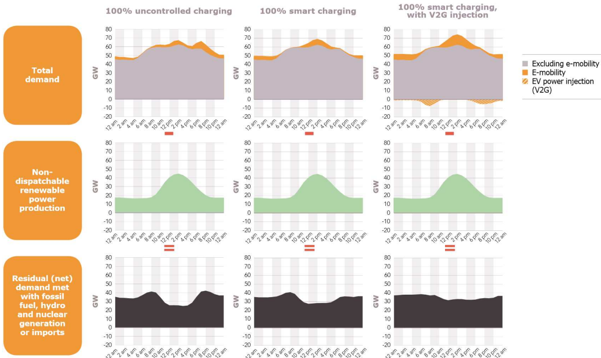
Figure 1.4: Total electricity demand in France and residual demand (total demand minus non-dispatchable renewable energy generation) in different EV smart charging configurations for an average weekday in 2035. Source: [RTE, 2019], Crescendo intermediate 2035 scenario.
