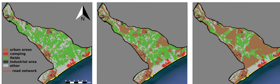
Fig. 1 Illustration of urban expansion (from left to right) in a river delta flowing into the Mediterranean Sea, as modelled with a cellular automaton using the NetLogo® platform. The urban areas (brown areas) are constrained by the distance to the road network (red lines) and the distance to the sea. Land uses derive from a study on the Lower Orb river fluvial plain by Saint-Geours et al. (2015) .
